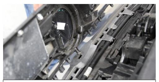
33. Insert the grill back into place – starting with placing it into the bumper.
