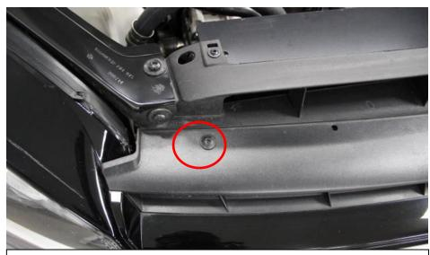
23. We will now remove the front grill. Start by removing the 2 screws, one on each side as shown here.
