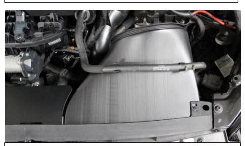
15. Now push the rubber hose into the clips on the duct to secure it.
