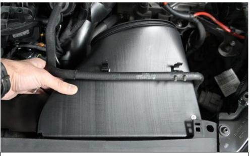
10. Place the duct assembly as shown and guide it into place – you might need to push the duct panels into place by inserting your hand inside the duct as shown in next step.
