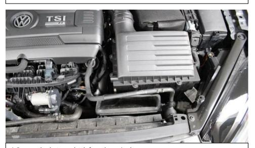
4. Remove the duct completely from the engine bay.
