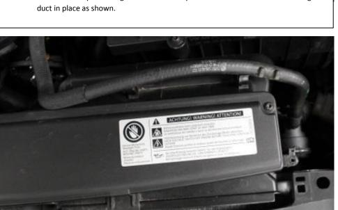
3. Now you should be able to remove the duct. If you cannot get enough movement, pull the airbox out of the mounts and push the airbox back for more clearance.
