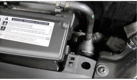
2. Now push the duct clips down to release from the slam panel. Do for both sides.
