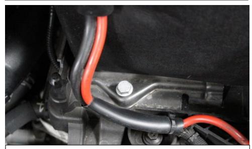
7. Remove this 13mm Bolt from the battery clamp. His is where the intake will secure.
