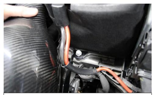
20. Keep the housing pressed against the duct and secure the bracket with the 13mm bolt removed in step 7.
