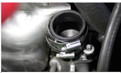
10. Push the tapered side down onto the flanges all the way down. Install the smaller hose clamps (40-60mm) onto the silicons. Make sure the clamps do not interfere with the screw face them away as shown. Tighten the clamps around the flange.
