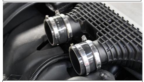
11. Push the larger silicons onto the charge cooler with the larger hose clamps. Tighten the clamps around the cooler.
