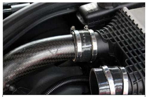
13. Now push into the upper silicons. For easier access you can loosen the charge cooler and lift it slightly.
