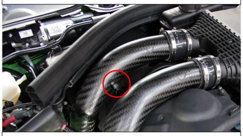
16. Remove the upper engine cover mount and install 1 spacer washer as provided.
