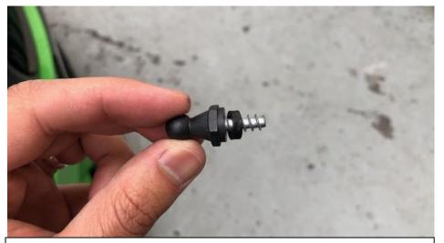
17. Use the provided plastic spacer washer and re-install it.
