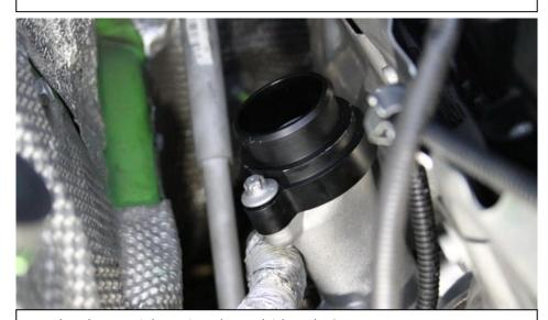
7. Push Both Eventuri Flanges into place and tighten the OEM screws.
