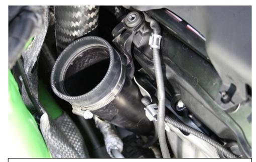
14. Install the turbo inlet tube again and secure with the OEM screw.
