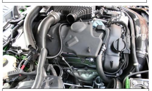
3. Remove the front chargepipe from the engine bay.
