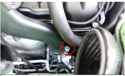
2. Remove the screw holding the front chargepipe on the turbo outlet pipe.
