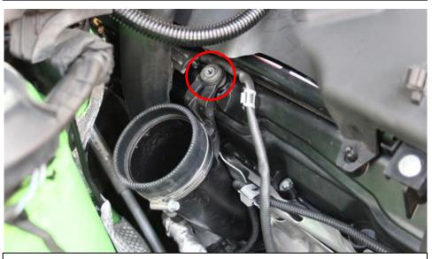
4. Remove the plastic turbo inlet pipe by removing the retaining screws and then pulling out the pipe.
