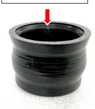
9. Use the smaller silicons for the flanges. One side of the silicon has a tapered edge as shown. This side must face down onto the flange and the non-tapered edge should face upwards for the carbon pipe.
