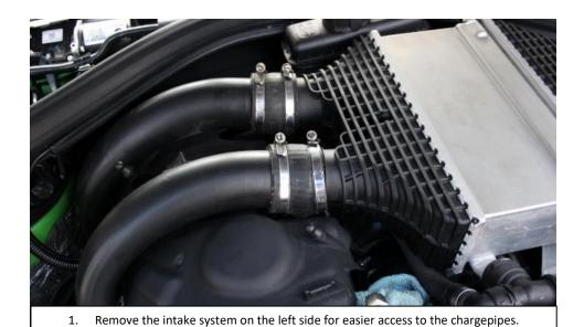
Start by loosening the hose clamps on the top side of the chargepipes.
