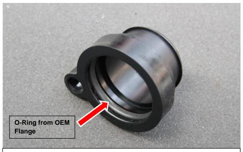
6. Remove the O-Rings inside the OEM chargepipe flanges and transfer them to the new Eventuri flanges.
