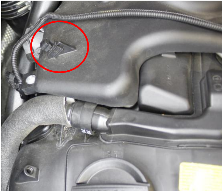
9. Remove engine cover to reveal MAF sensor plug wiring for the left side. Using a flat head screw driver, open the wire holder and take the loom out.
