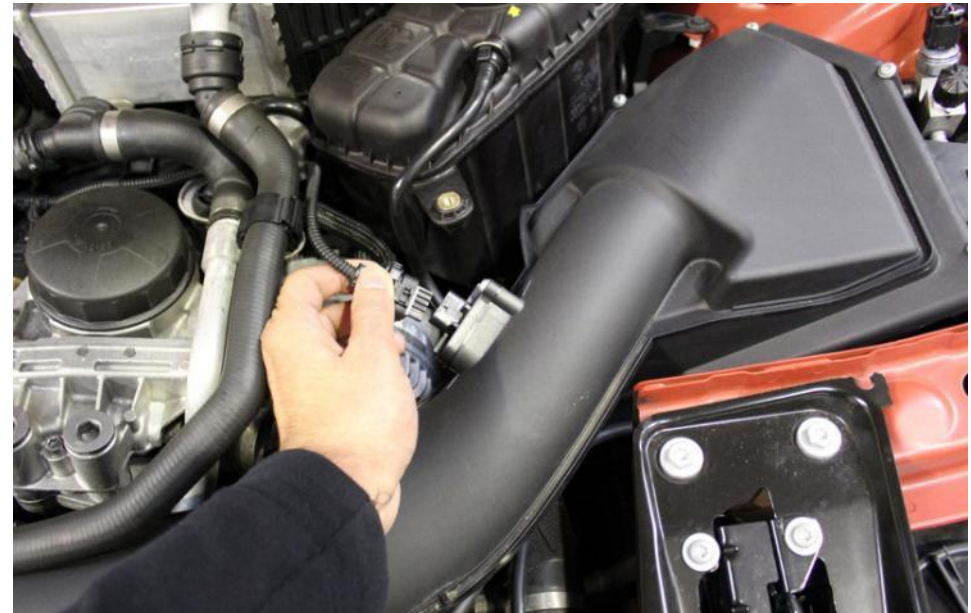
10. Remove MAF plug from right side airbox.
