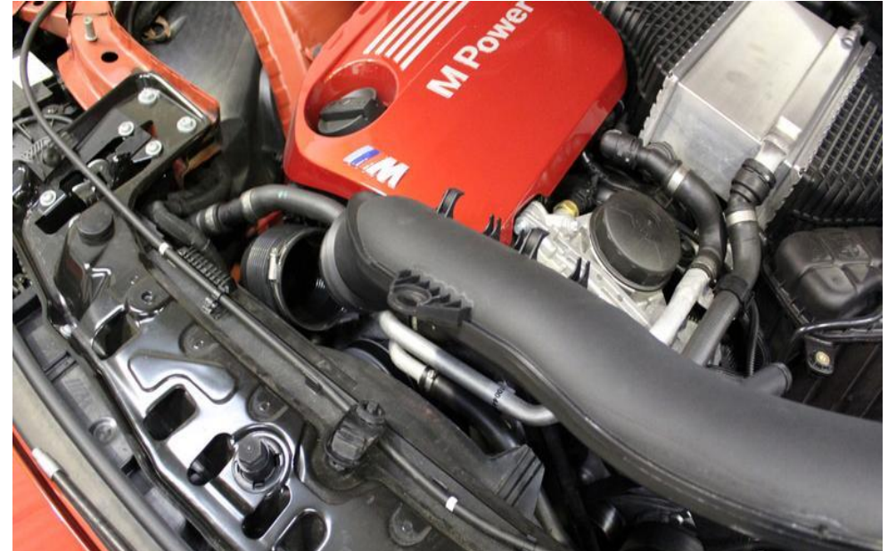
14. Loosen hose clamp and pull the tube out from the intake pipe.
