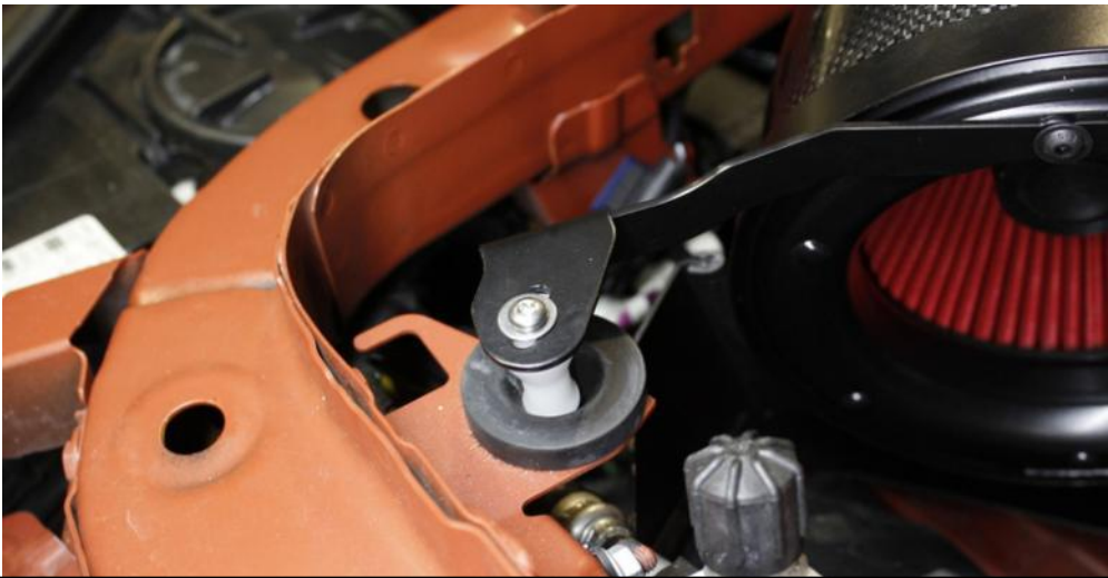
41. Locate the mounting boss over the stock rubber grommet. If required, rotate the mount and filter assembly in the housing. Band clamp should be loose enough to allow this – otherwise loosen to allow rotation. (Photo shown without the duct)
