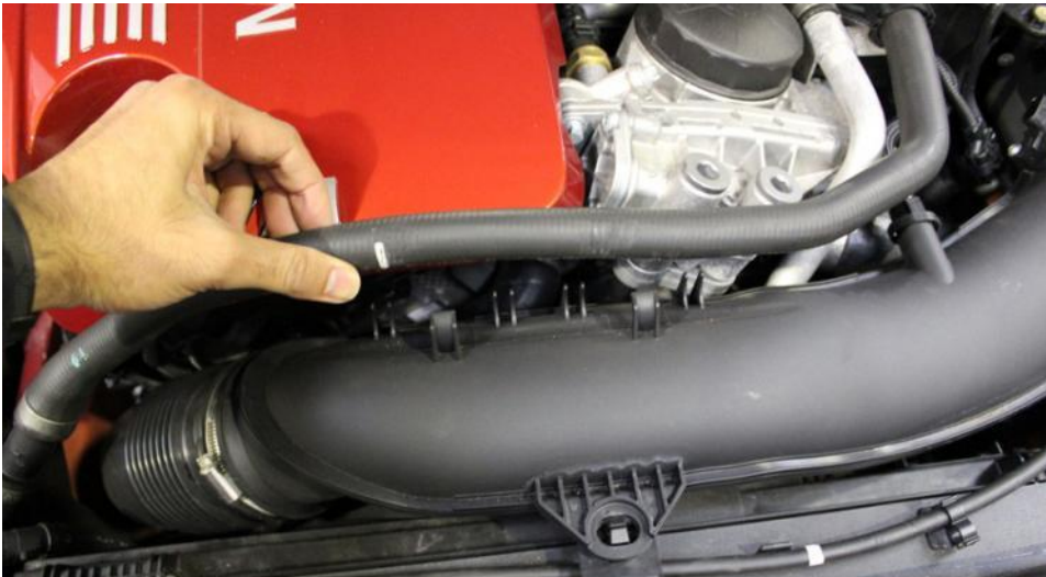
11. Pull the rubber hosing out of the long intake tube.
