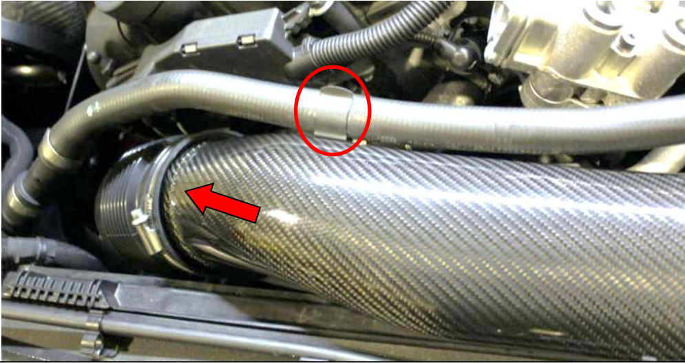
39. Raised section of the carbon tube pushed inside the flexible hose (red arrow). Also push the stock rubber hose into the metal clip on the carbon tube as circled.
