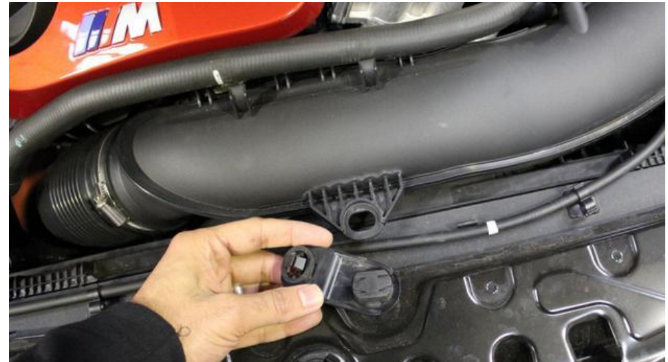
12. Remove the centre mount from the tube by pushing the two tabs together and down. Then remove this mount from the engine bay completely by rotating rubber head 90 degrees.
