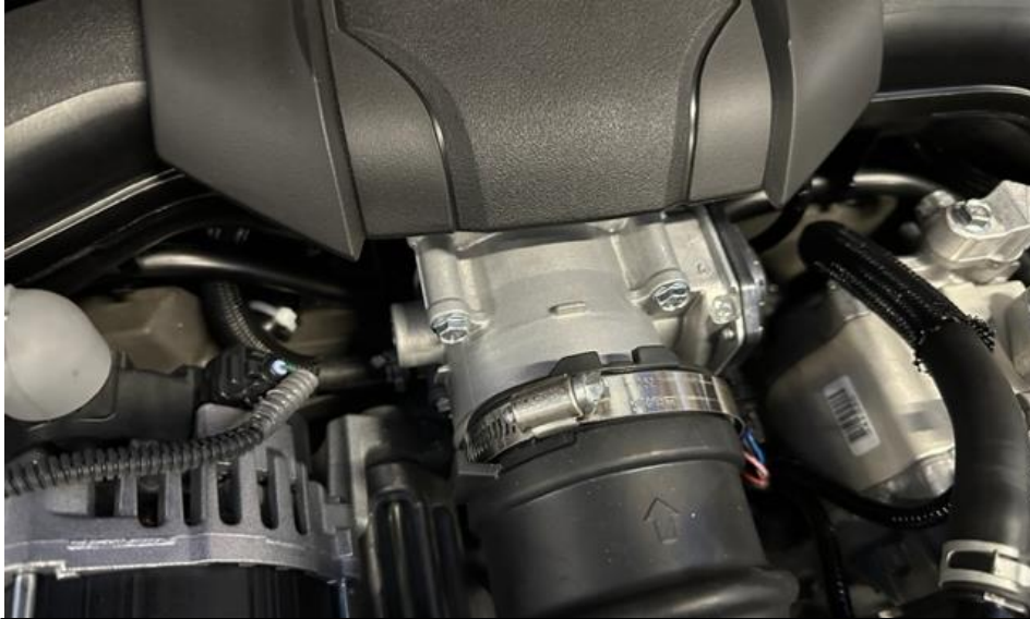
9. loosen the clamp around the inlet hose.
