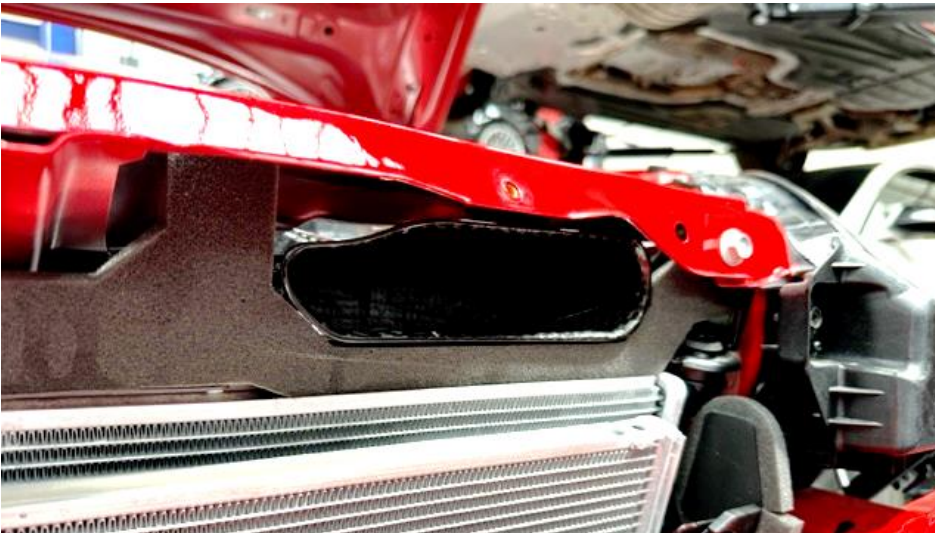
19. The right side of the duct should go through the existing opening.
