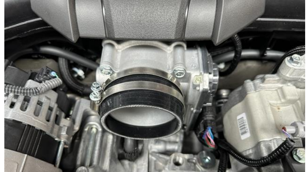
26. Install the supplied silicon coupler onto the throttle body. Push the hose clamps back as far as possible to allow the filter housing to be placed into position.
