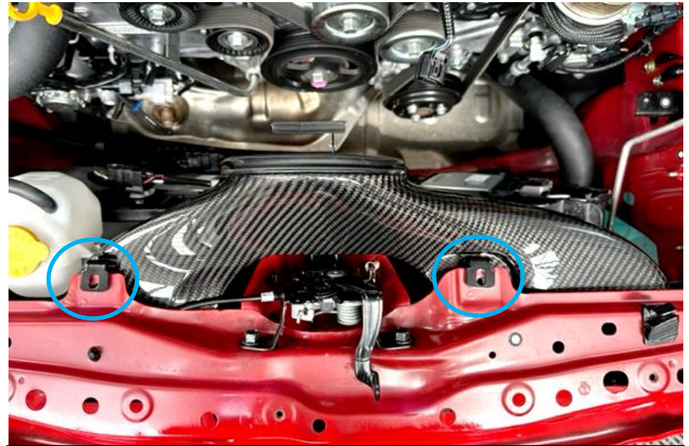
18. Position the 2 brackets as shown over the OEM mounting holes. Push the duct through the foam gaps in the slam panel area see next steps.
