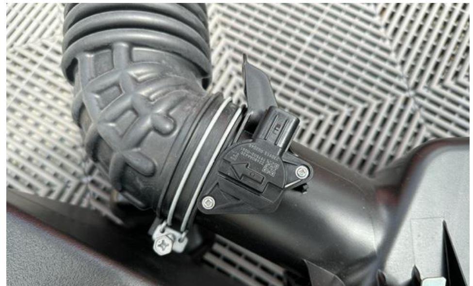
12. Remove the MAF Sensor from the airbox by removing the 2 screws. We will not be using these screws.
