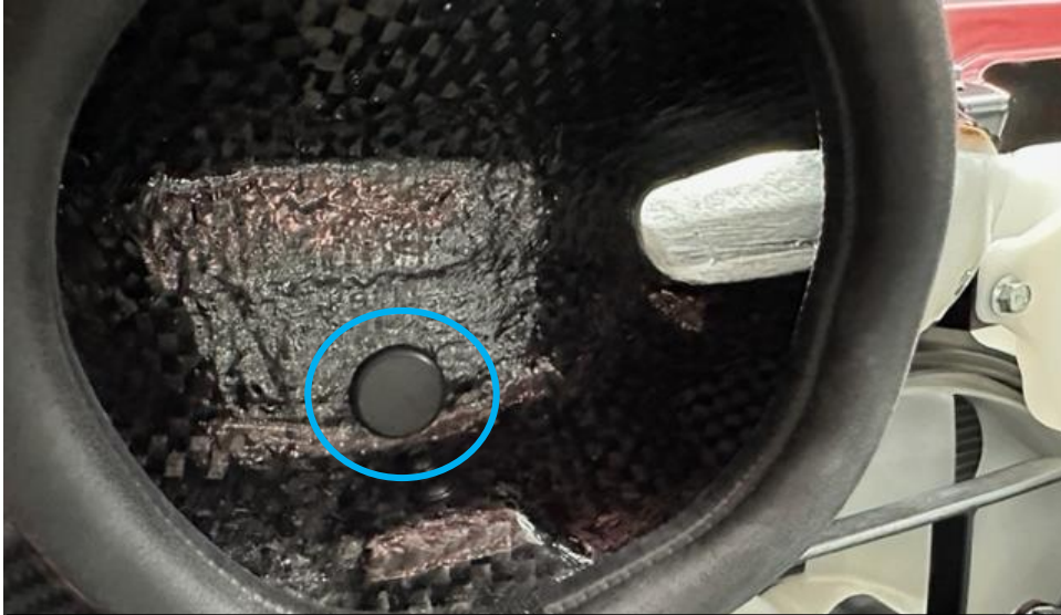
25. Now plug the hole with the supplied rubber grommet.
