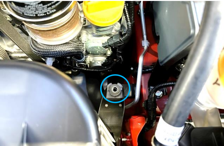
7. Remove the bolt holding the base of the airbox.
