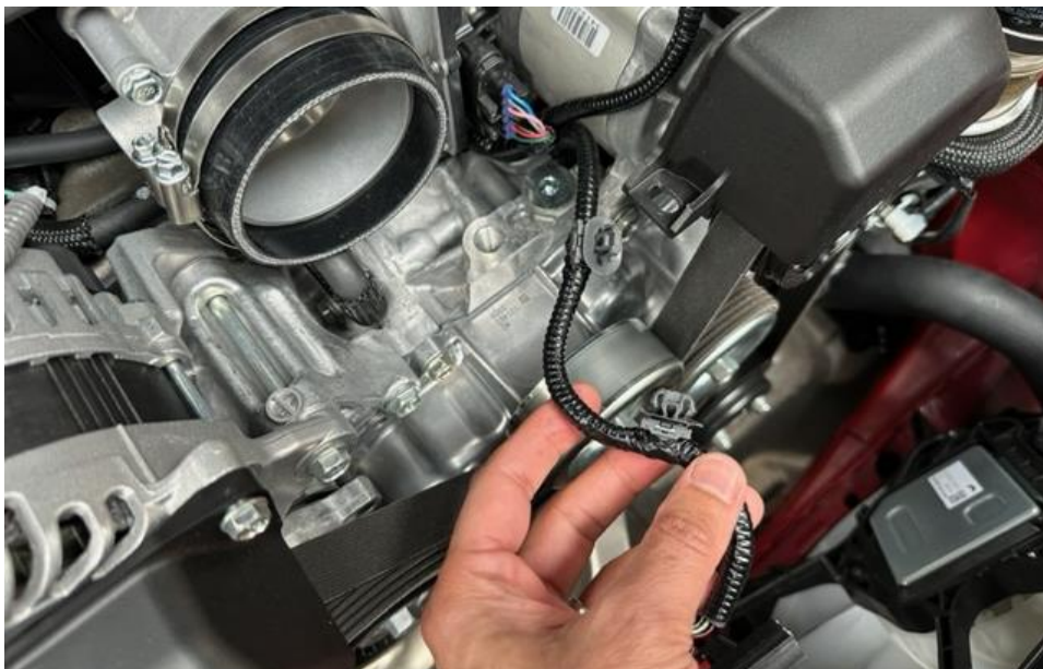
27. Unclip the MAF sensor loom from the pulley cover.
