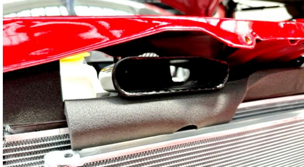
20. On the left side, fold the foam down and push into the gap between the radiator and condenser.
