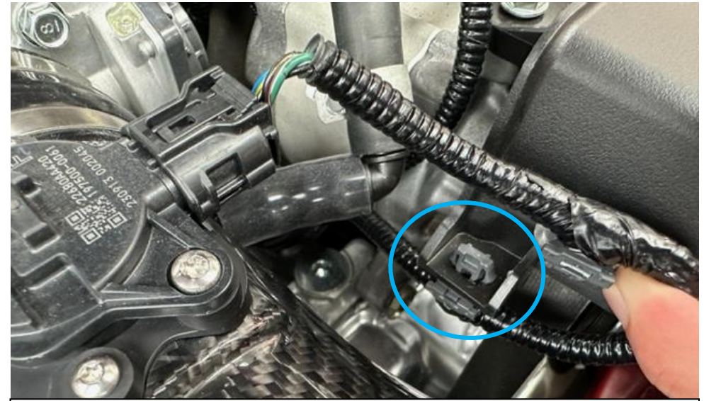
30. Push the second clip on the MAF wire into the mounting hole from underneath.
