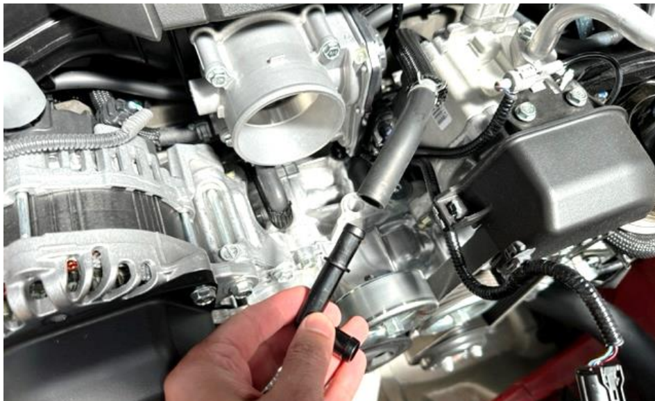
11. Remove the L shape breather pipe from the rubber breather hose.
