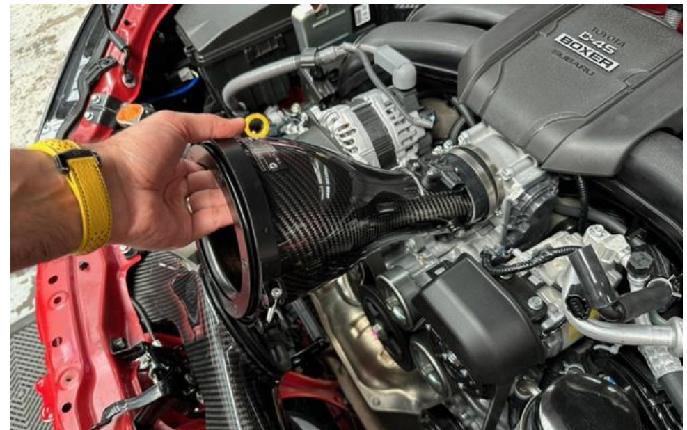
28. Place the back of the filter housing into the silicon and carefully rotate the housing downwards.
