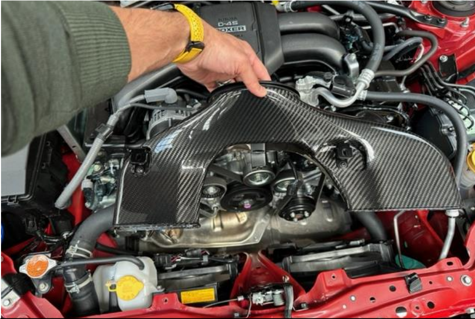
17. Lower the carbon duct into position. The 2 openings on each side should go into the gaps in the slam panel – see next step.
