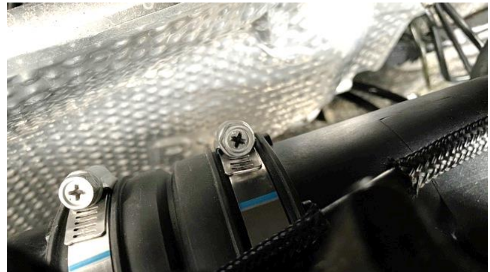
18. With the tube mount rotated into the correct place – tighten the hose clamp around the tube.
