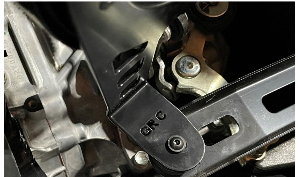
24. Push the mounts into the rubber grommets on both sides.
