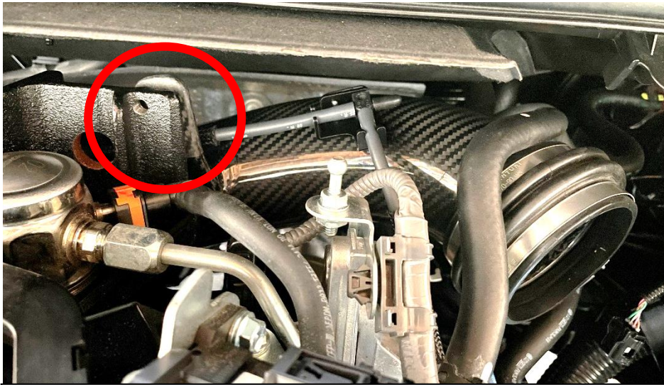
17. Insert the tube into the OEM rear rubber hose. Rotate the tube so that the tube mount lines up with the metal bracket. Do not insert the newly supplied M8 bolt yet.
