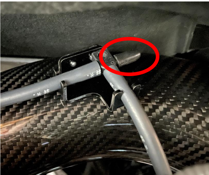
19. Plug the T-Piece with the supplied banking plug and secure it to the bracket on the tube.
