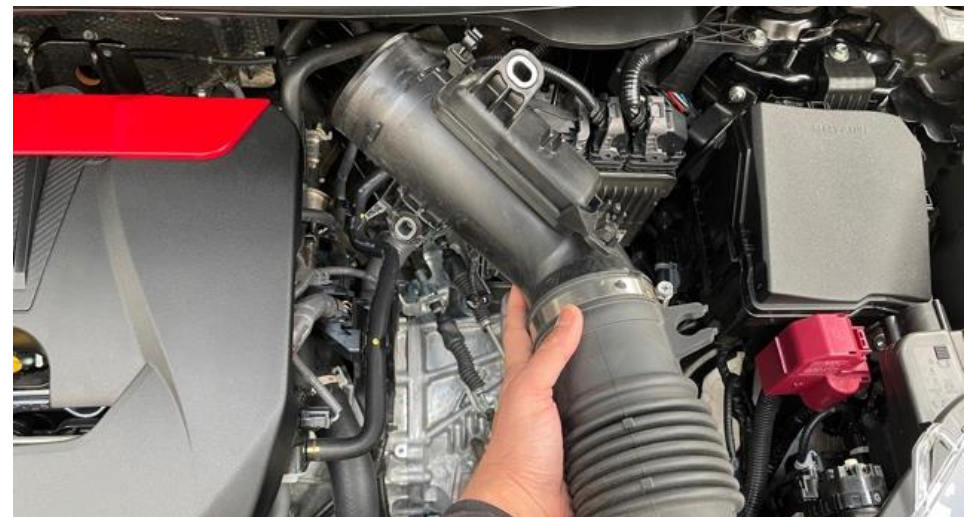
12. Remove the tube from the engine bay.
