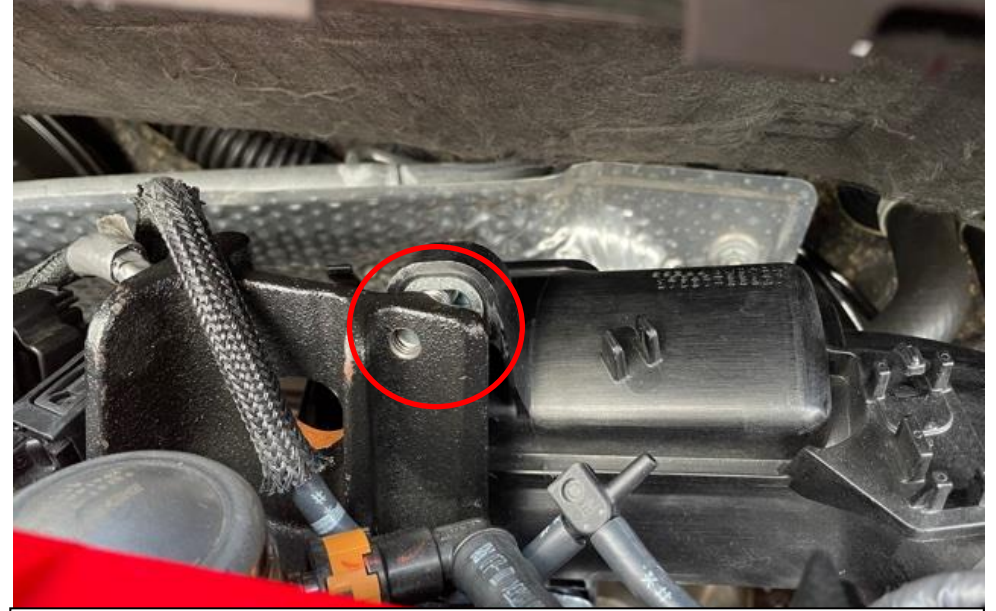
10. Move the vacuum line out of the way and remove the M8 bolt with 12mm head holding the top of the tube in place. There is also a second M8 bolt on the lower side of the tube – remove this also (cannot be seen in the photo).
