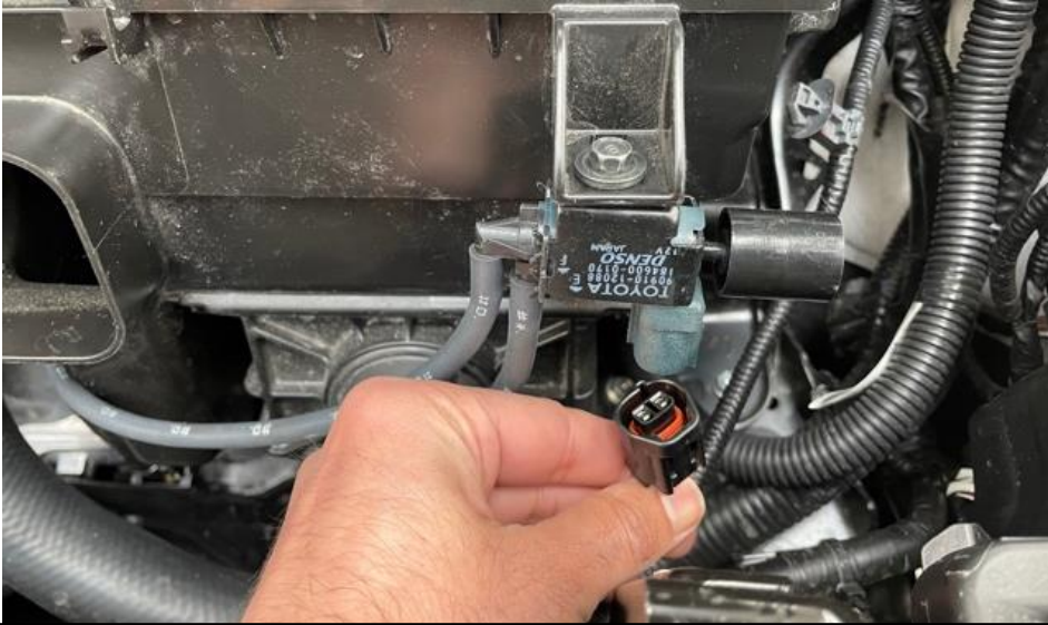
5. Unplug the module on the airbus and remove the bolt holding it secure.
