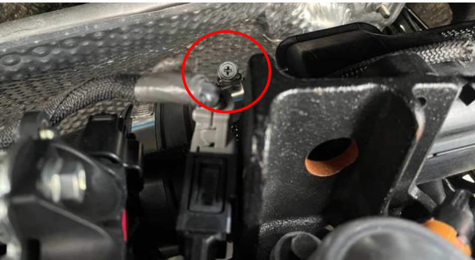
11. Loosen the hose clamp at the back of the tube.
