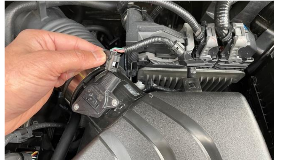
8. Disconnect the MAF sensor plug – make sure the ignition is OFF.
