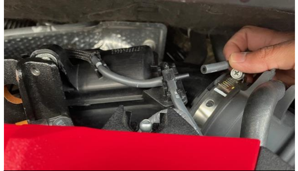
6. Disconnect the vacuum line from the T-Piece on top of the rear tube.
