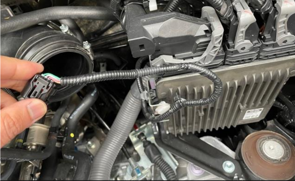
21. Remove the plastic shroud around the MAF sensor wire.
