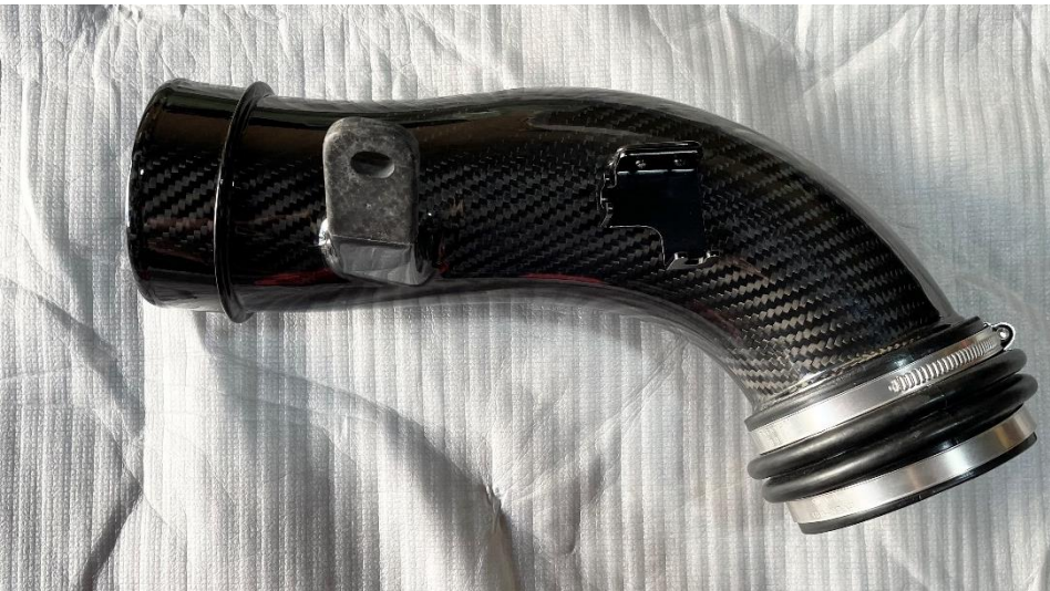
15. Push the flexible hose onto the carbon tube as shown.
