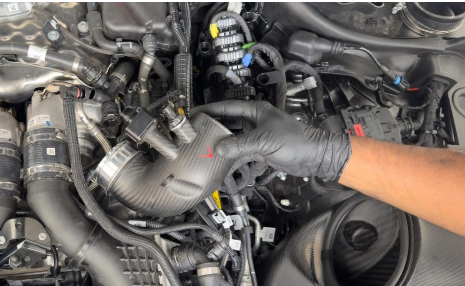
11. Install the RHS inlet. Push it onto the turbo and the spring clip should lock it into place.
