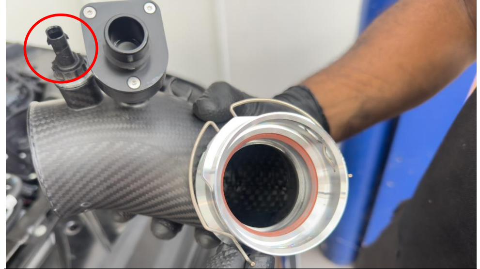
10. Screw the sensor into the RHS inlet.
