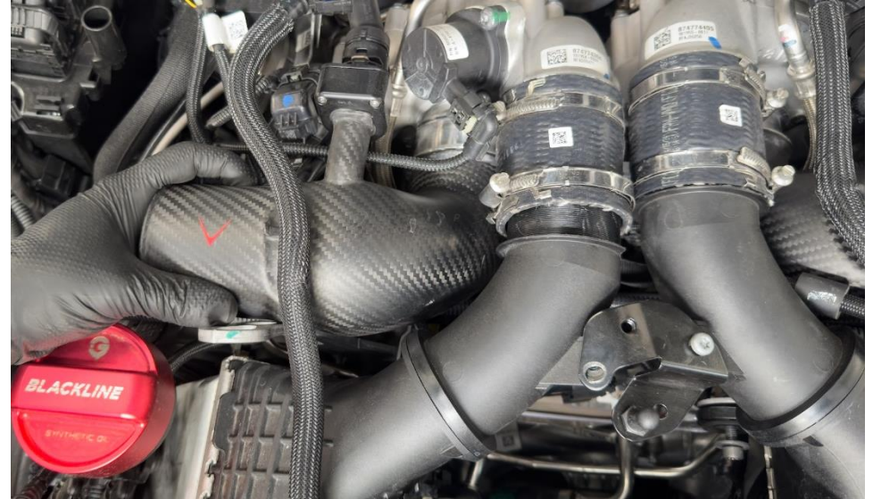
18. Pull the charge-cooler out to allow enough clearance for the inlet to be installed.
