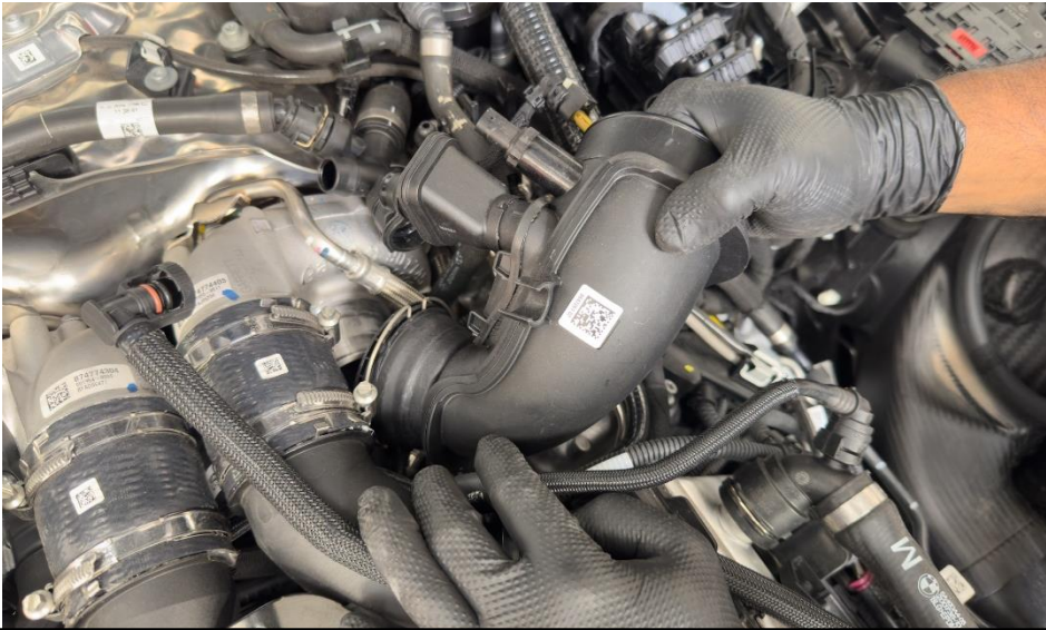
5. Remove the inlet from the engine.
