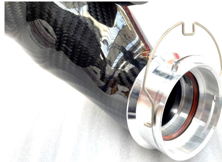
8. Insert the spring clip onto the machines flange with the top of the clip positioned over the raised section. Also insert the O-ring inside the flange as shown. The tapered face of the gasket should face the turbo.
