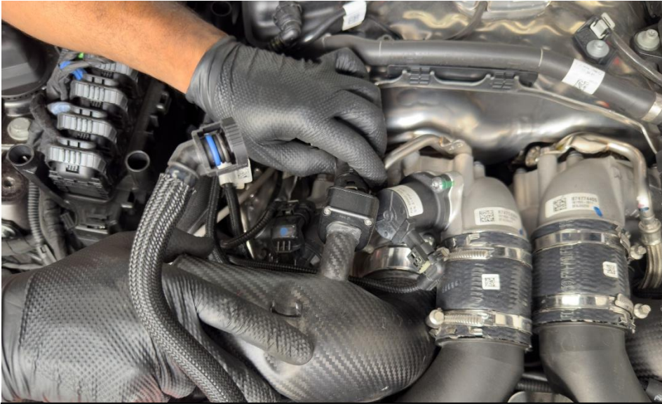
21. Reconnect the breather system to the inlet tube and the breather hoses together.
