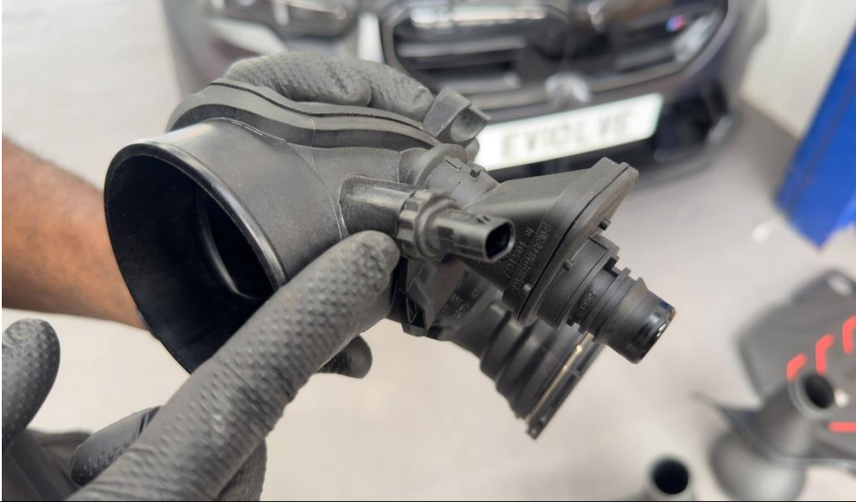
9. Unscrew the temperature sensor from the RHS inlet.
