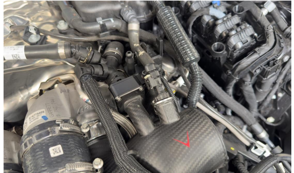
12. Reconnect the temperature sensor plug and the breather hoses.
