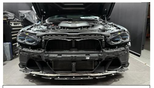
1. We recommend having the front bumper professionally removed. It is held in place by a number of push clips, 10mm screws and T30 Torx screws. BMW M4 shown for illustration.
