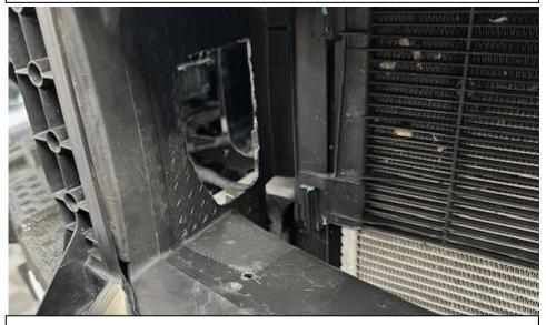
4. Mark the shape of the opening and then using a Dremel or similar, carefully cut away the shape.
