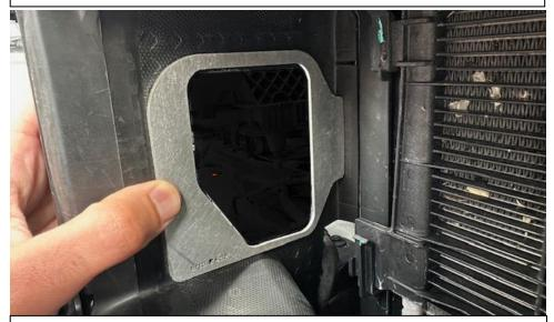
3. Take the LHS template and place it on the left side of the front shroud panel (left side as you look at the car from the front). The bottom of the template should touch the base panel and the back of the template should touch the rear panel as shown.
