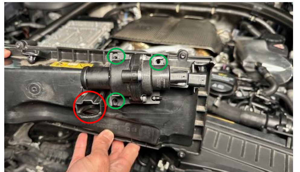
12. Remove the rubber mount circled red. Also remove the 3 screws holding the module in place.
