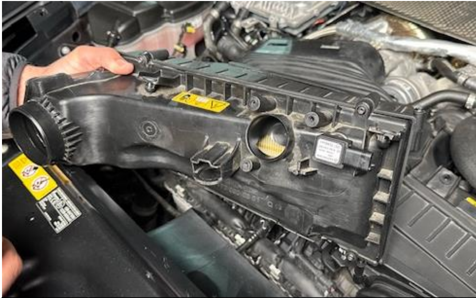
13. Remove the module from the air box.
