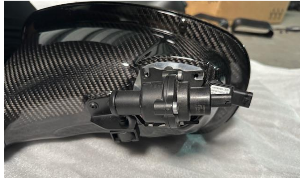
20. Push the air module into the airbox as shown and line up the 3 holes on the bracket.
