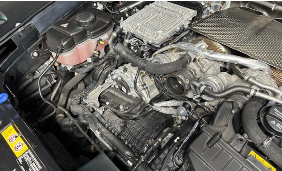
11. Remove airbox from engine and repeat for the other side.
