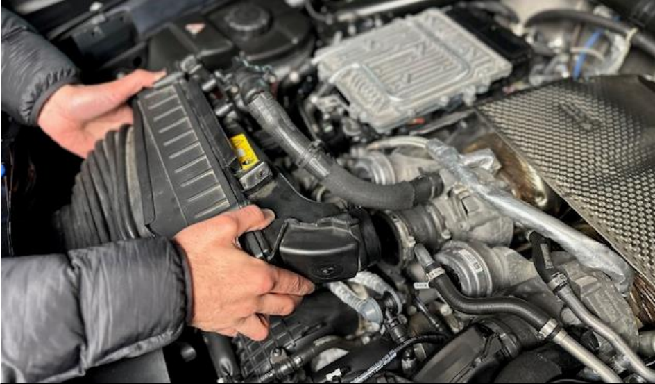
9. Pull the airbox away from the turbo.
