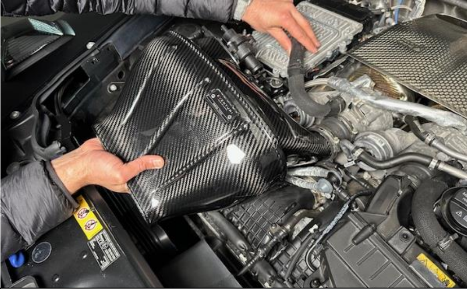
25. Take the Left side assembly and push into the turbo inlet. Then rotate it down.
