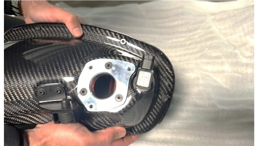
18. Push the MAP sensor into the Eventuri airbox as shown – starting with the sensor in a vertical orientation.
