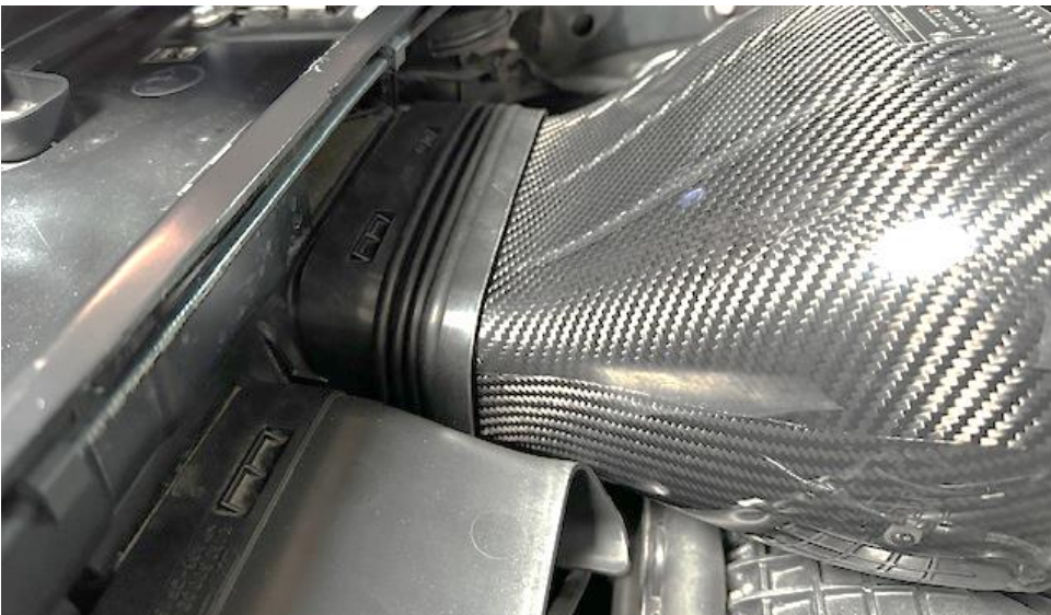
27. Once the airbox is fully located pull the flexible coupler around the carbon and into position as shown.
