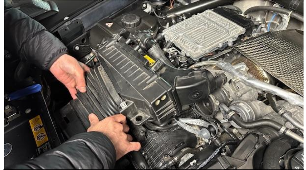
10. Now remove the duct from the from air feed.
