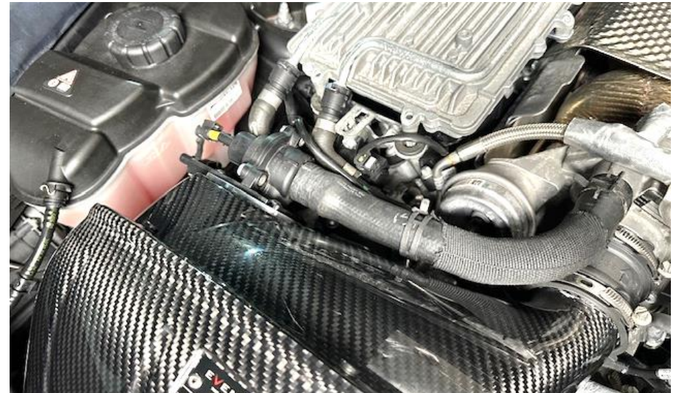
28. Push the hose back into the air module. Secure it with the spring clamp.
