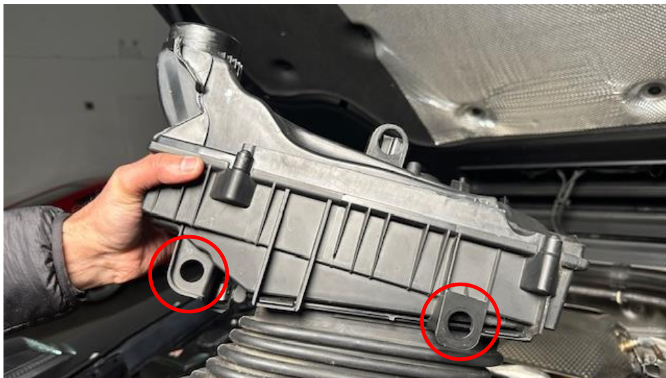
15. Remove the 2 rubber mounts from the airbox base as shown. We will re-use these in the next step.
