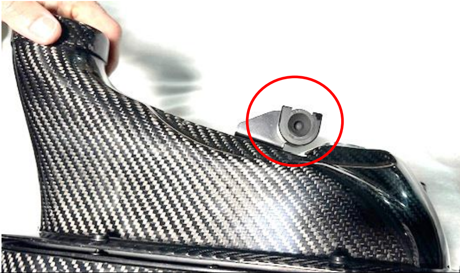
17. Install the rubber mount from step 12 into the machined mount holder on the lid as shown.
