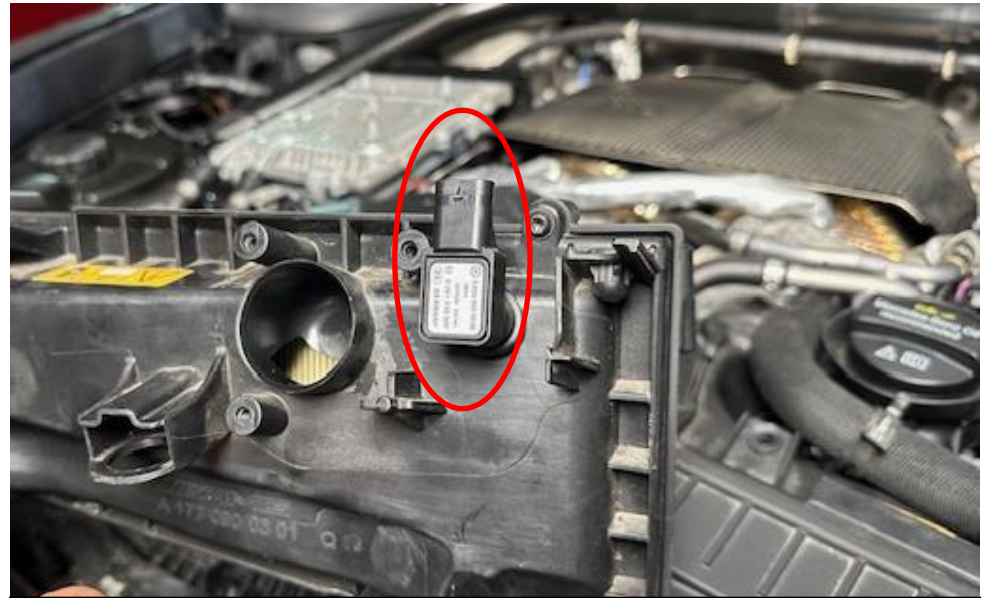
14. Rotate the MAP sensor 90 degrees as shown and pull it out.
