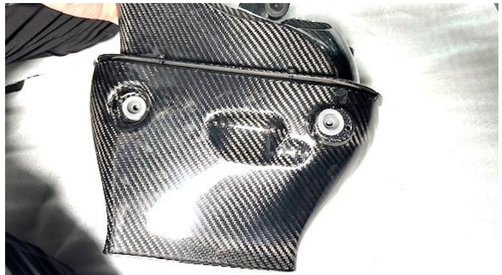
16. Install the 2 rubber mounts into the holes on the carbon duct as shown.
