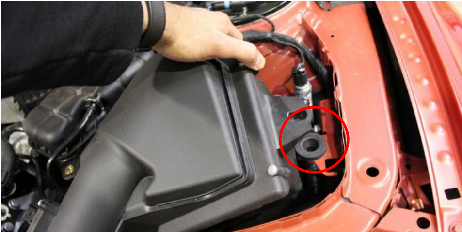
15. Pull the right side of the airbox upwards and out of the rubber grommet as can be seen here. Remove the airbox and tube assembly completely from the engine bay.
