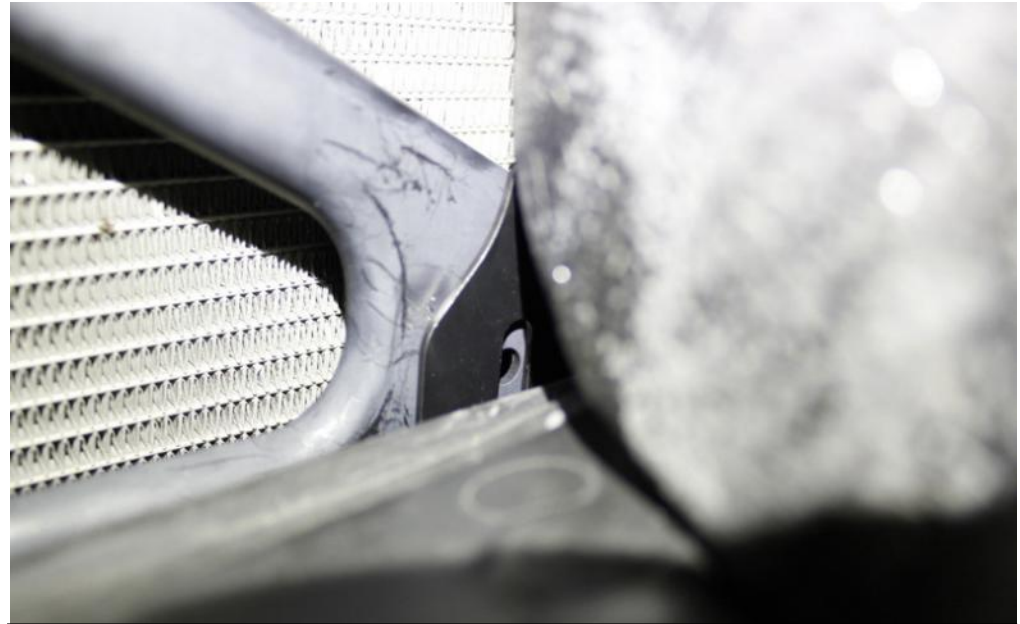
61. As previously, align the bracket with the hole on the strut brace and secure with the push rivet.
