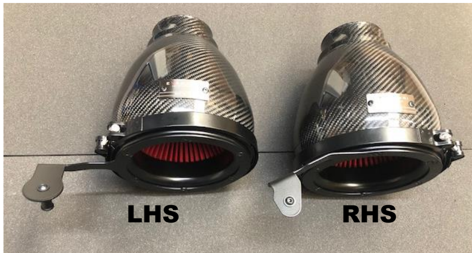
30. Identify the left and right side intakes. The left side has the mounting bracket secured around the bottom of the opening. The right side has it secure around the top as shown. The brackets are also a different shape.
