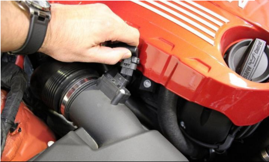
5. Disconnect MAF sensor plug from left hand side airbox.
