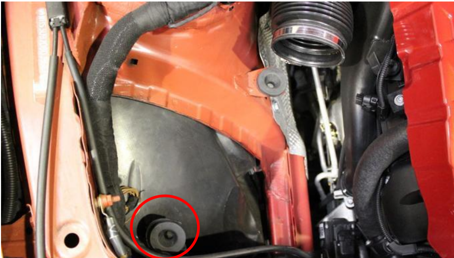
7. The front grommet is placed on a thin metal plate which can bend upwards with the removal of the airbox – if so, push it back down so that it is horizontal again.
