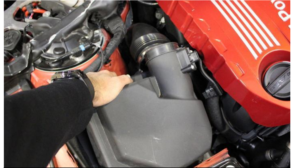
6. Push the intake tube off the airbox and then pull the back of the airbox upwards to remove. It is held in place by 2 rubber grommets. Remove the airbox from the engine bay.
