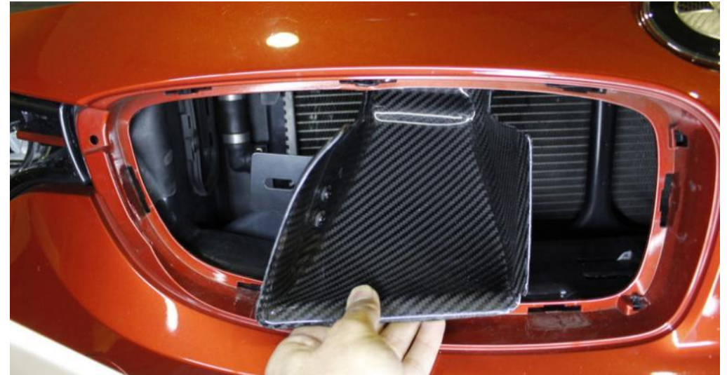
51. Insert the LHS scoop into the left side as shown with the bracket towards the left headlight. Once inside, rotate 90 degrees counter clockwise so that the bracket faces down. The scoop should be positioned as shown in the next steps.
