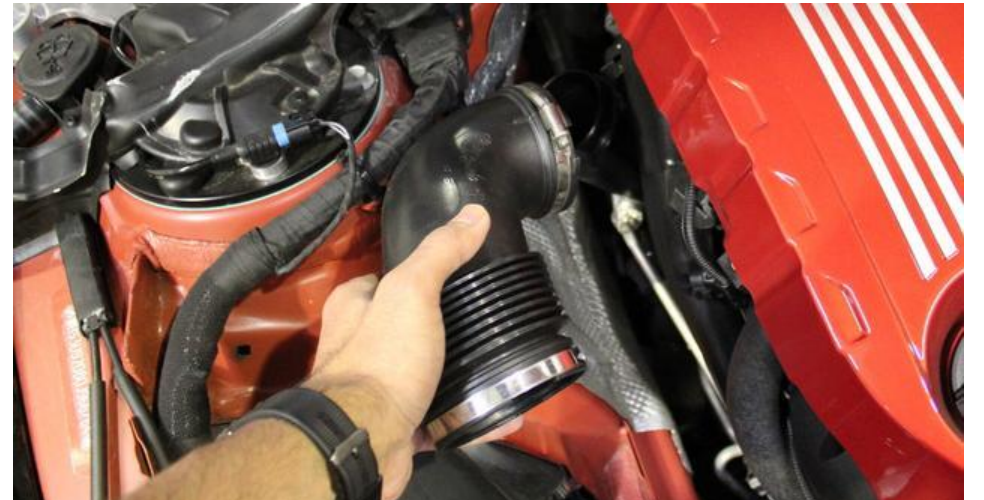
8. Loosen the remaining hose clamp on the intake tube and remove from engine bay.
