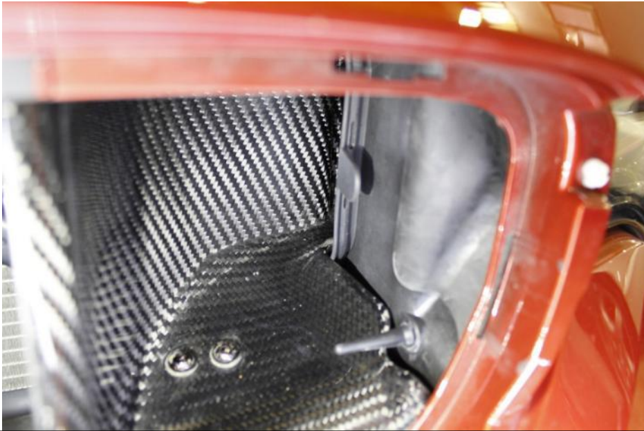
60. The back of the scoop should be positioned as shown inside the stock opening.
