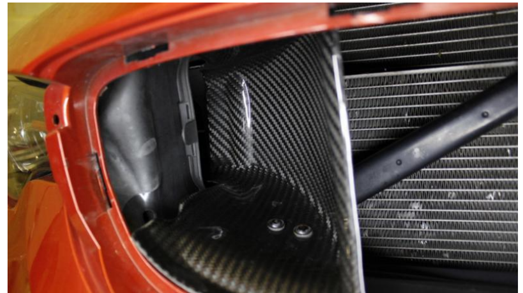
53. The back of the scoop should be sitting inside the stock duct opening as shown.
