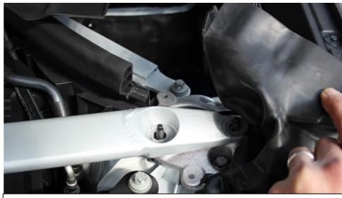
2. Underneath the rubber end covers on each side of the brace there are 2 nuts to remove.
