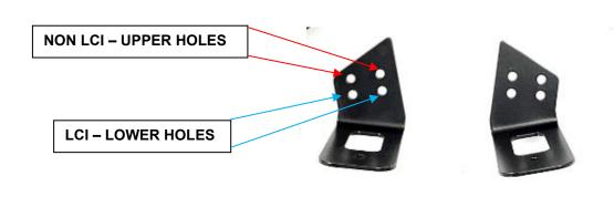
2. Secure the brackets to the scoops as shown. Notice there are 2 sets of holes on each bracket. Please use the correct holes depending on if your car is an LCI or not. See next steps.
