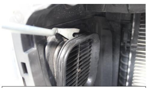
15. The grills are held in place with a tab on top and at the bottom. Carefully prise the clips out and remove the grills.
