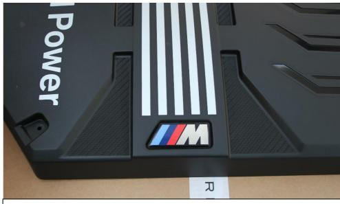
10. Remove the M Badge from the cover – it is held in place with tabs on the reverse – these can be carefully bent back and the badge can be removed.
