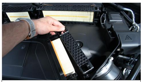
6. With the clips removed, the frames can be removed as well. Take out all the filters. If you also have grey charcoal filters behind the paper filters, you may also remove these.
