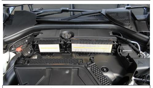
4. Loosen the screws on top of the airbox lid and lift the lid off to expose the filters.
