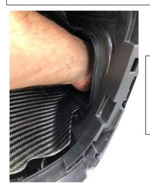
20. The inner duct panel may come loose as you push the clips in – pull the panel towards the scoop to ensure it secures with the scoop clips.
