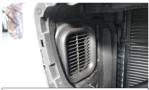
14. Remove the grills covering the air entry ducts.
