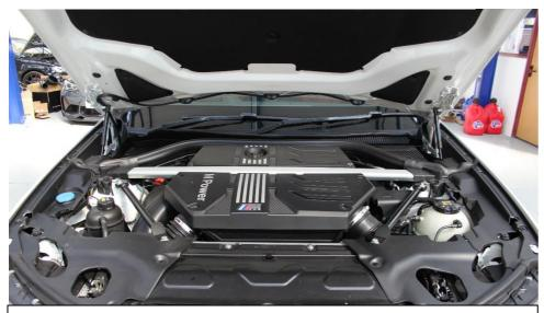
1. Start by removing the strut brace.
