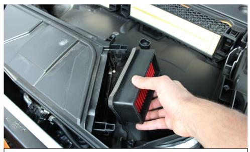
7. Install the new filters into the airbox as shown.
