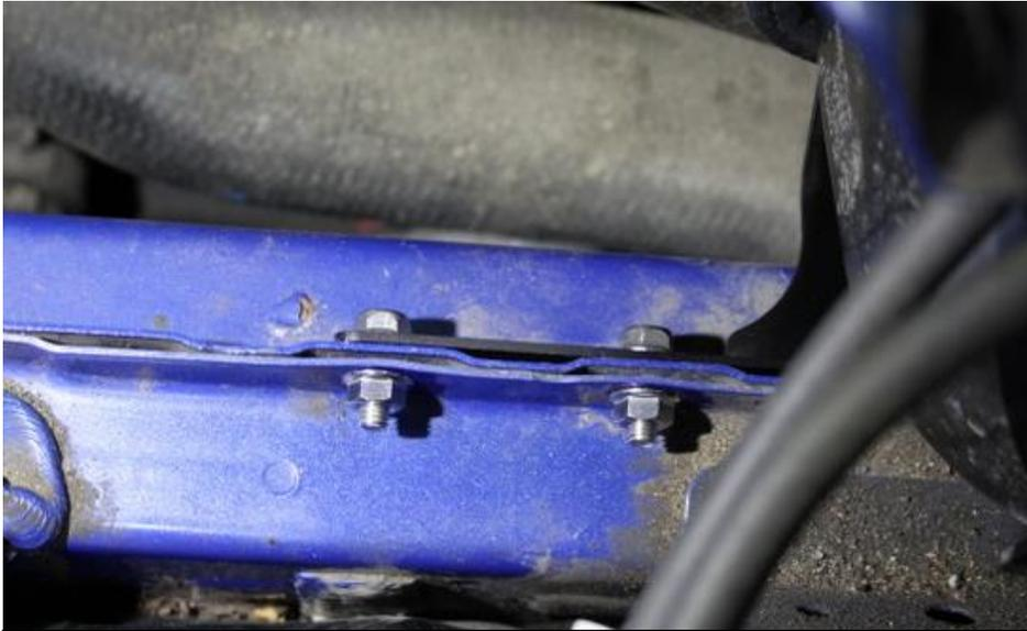
21. Use the supplied M6 Bolts and Lock nuts to secure the lower duct bracket to the chassis as shown.
