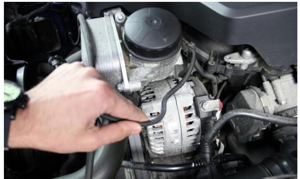
8. Pull the MAF sensor wire out of the clip located above the alternator. We will re-route this wire.
