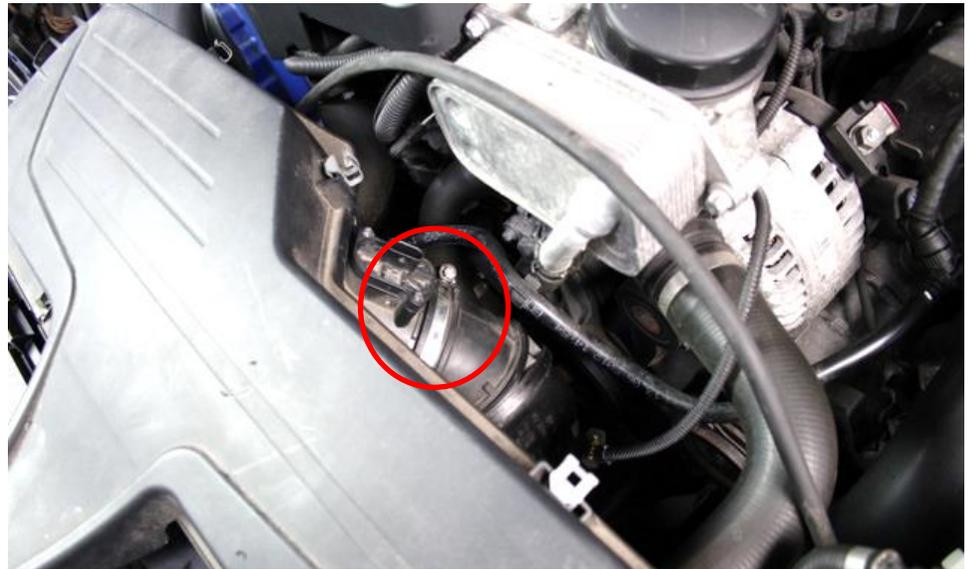
4. Loosen the hose clamp which secures the inlet pipe to the back of the airbox.
