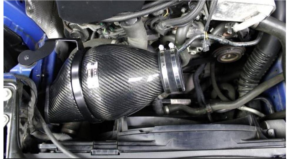
22. Push the supplied silicon coupler onto the filter housing with the 2 supplied hose clamps. Leave half the silicon extending outside the housing for the carbon tube. Secure the clamp around the Housing.
