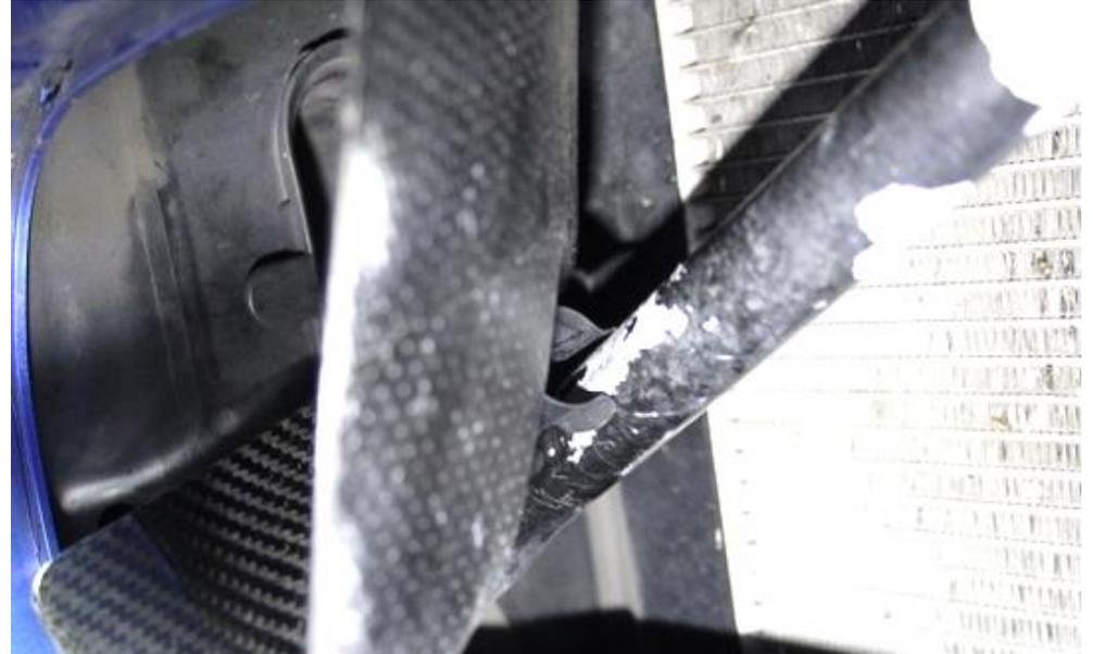
34. The clip should go over the strut bar.
