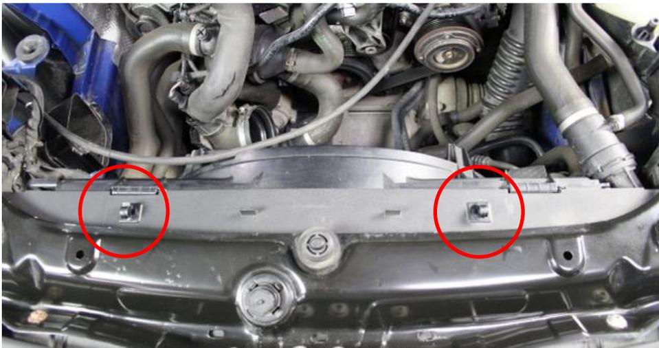
11. Insert the clips into the 2 holes shown above – located above the fan.
