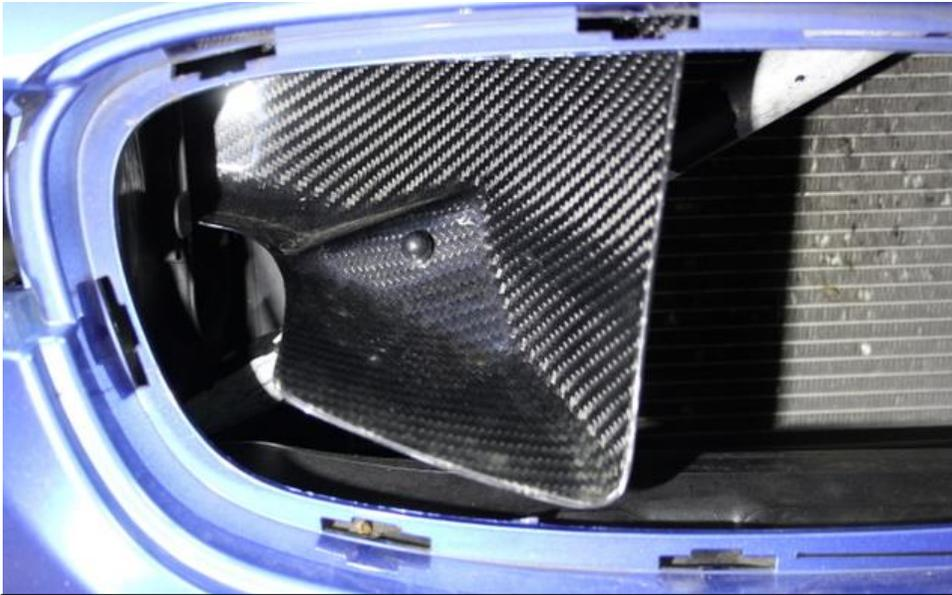
33. With the scoop rotated – now place the clip on the back of the scoop over the strut bar.
