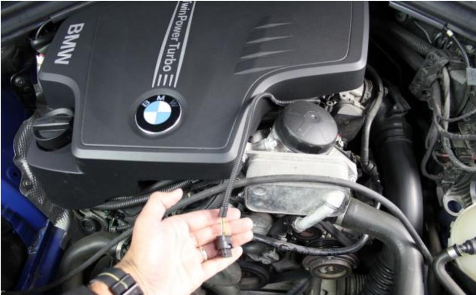
9. Route the MAF sensor wire around the back of the coolant module as shown.
