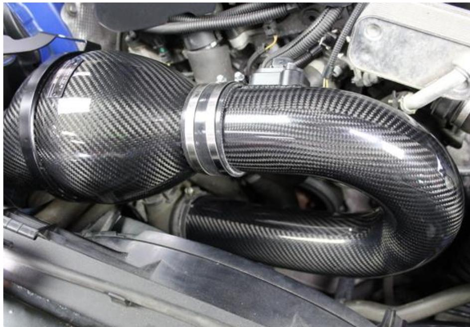
27. Push the upper part of the tube into the silicon fully and secure the hose clamp.
