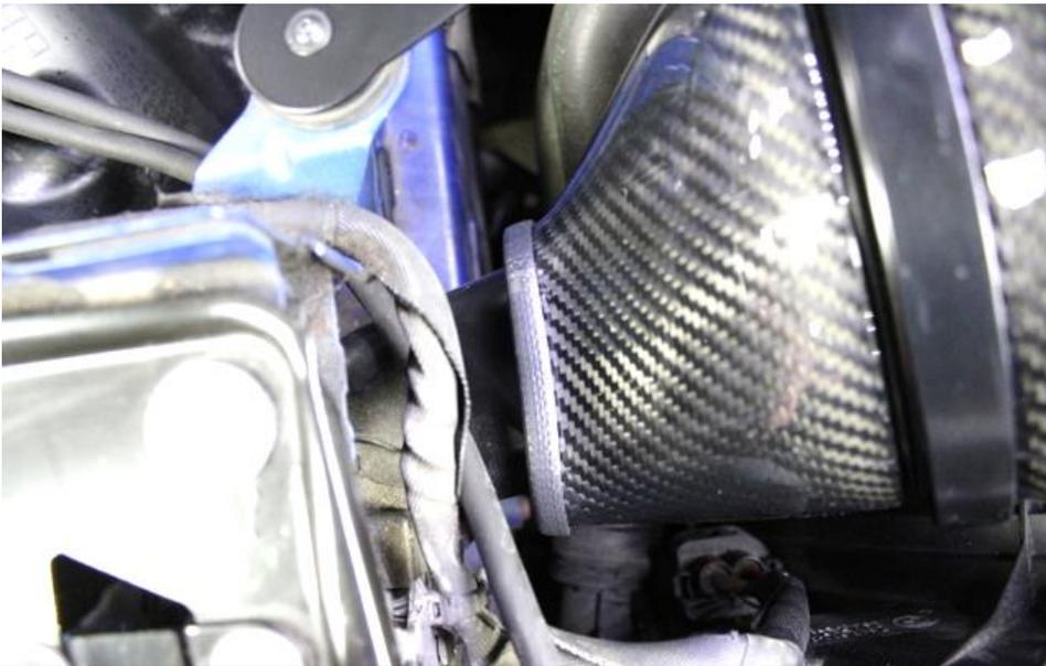
19. The carbon duct should sit as shown – squarely over the plastic OEM duct.
