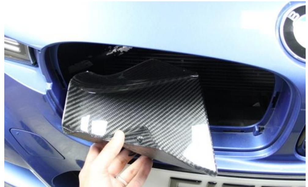
32. Insert the scoop into the nose of the bumper as shown and then rotate as shown in the next step.
