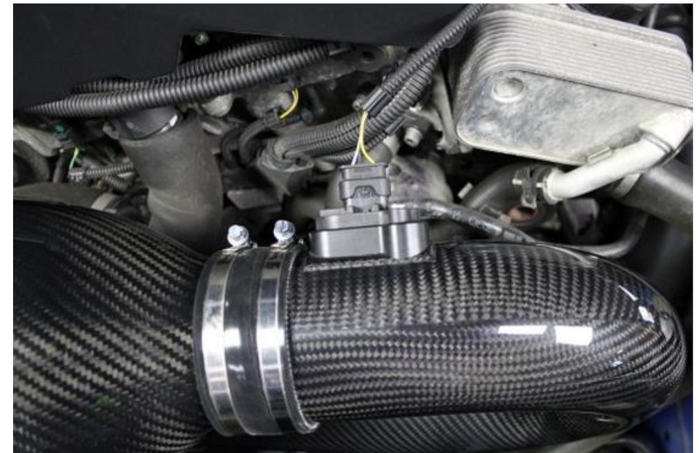
28. Firmly push the MAF sensor plug back into the sensor.
