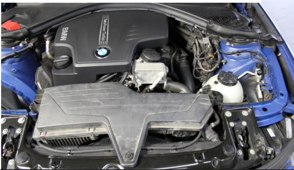
1. We will start by removing the stock airbox system
