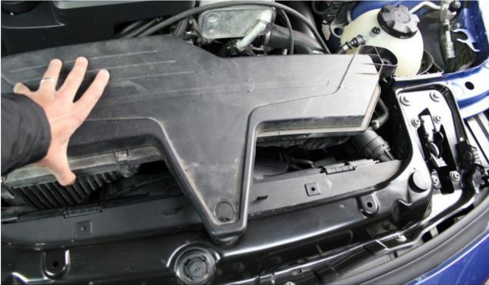
5. The Airbox can now be removed by lifting it out of the rubber mounts and inlet tube.
