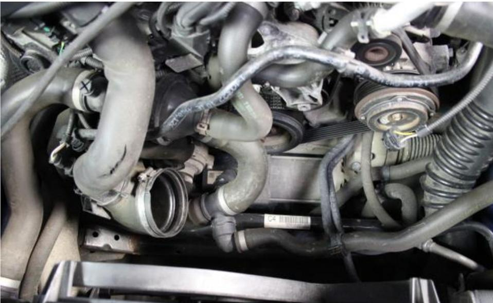
7. Remove the inlet hose from the engine bay.
