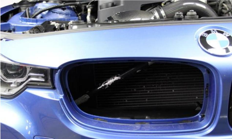
29. Remove the left grill = it is held in place with 8 tabs which need to be pulled towards the centre of the grill while pulling the grill out to release.
