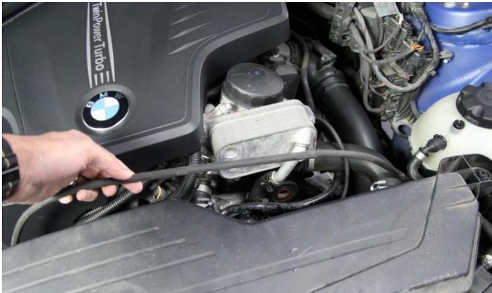
3. Remove the hose from the clips around the rear of the airbox.
