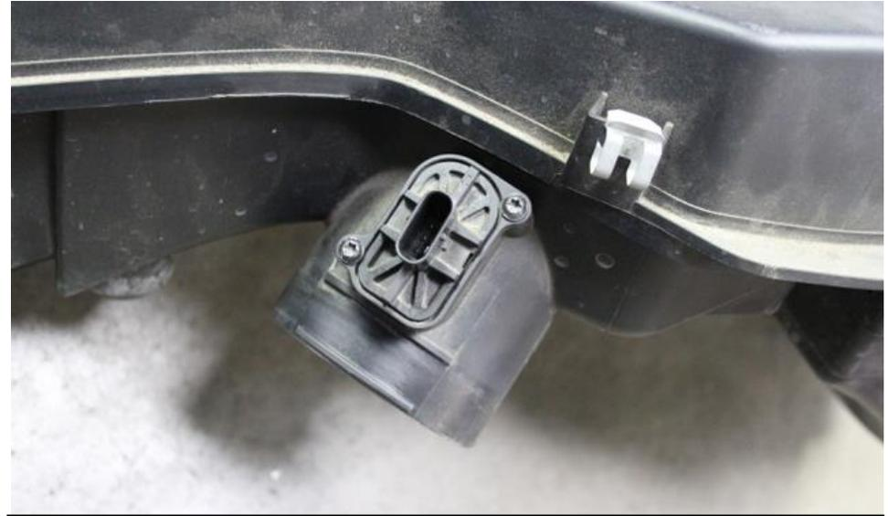
14. Remove the MAF sensor from the airbox – it is held in place with 2 torx screws.
