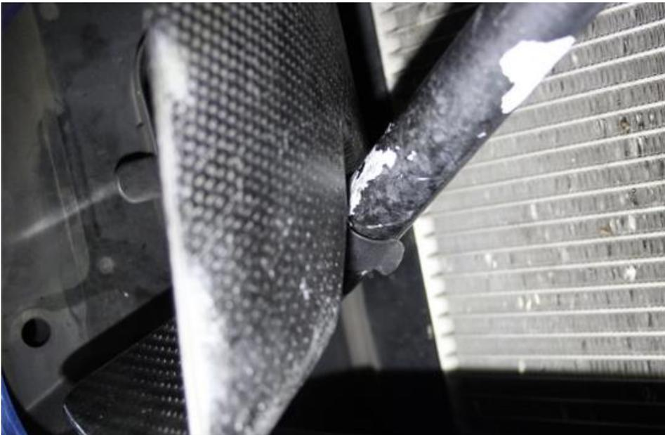
35. Now push the scoop so that the clip locks over the strut bar.
