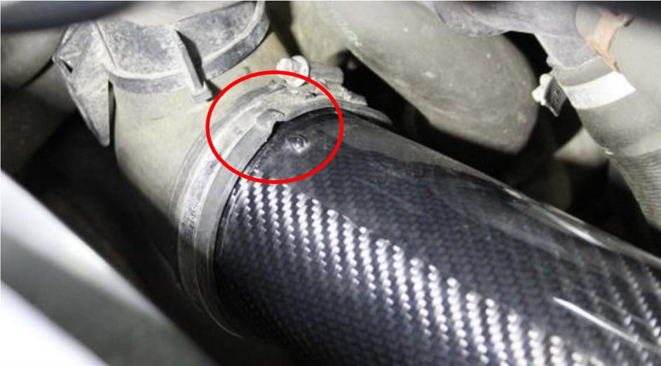
25. Push the lower part of the tube into the inlet – notice that the notch on the tube should line up with the notch in the inlet hose.
