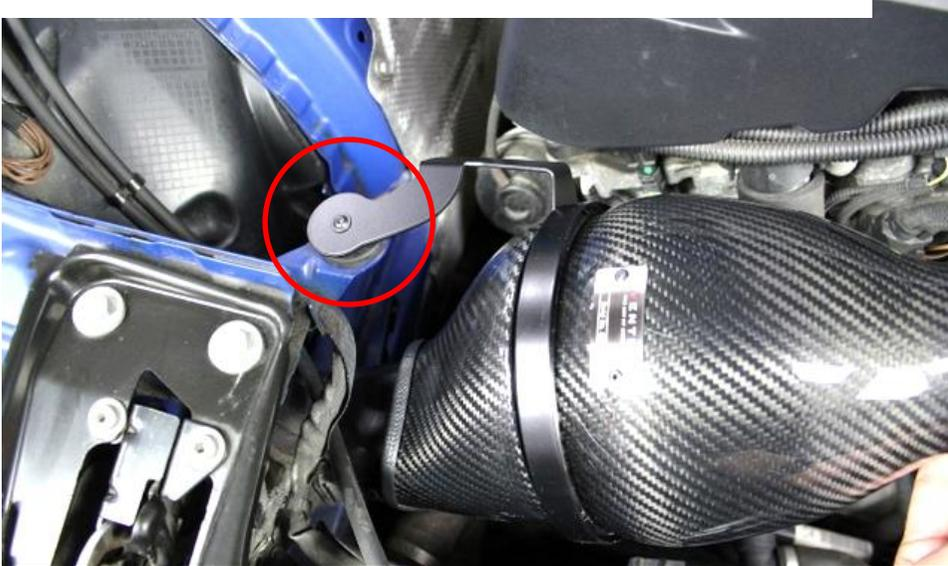
17. Lower the assembly into position and push the upper bracket mount into the OEM rubber mount used for the airbox as shown. The rubber mount might still be attached to the airbox.
