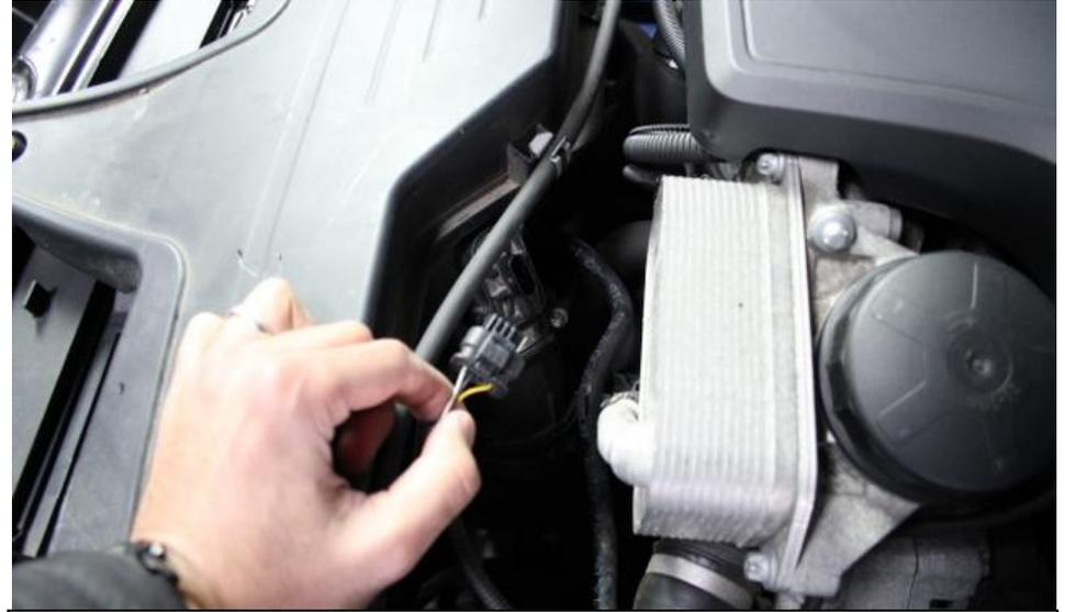
2. Remove the MAF sensor plug located at the back of the airbox.
