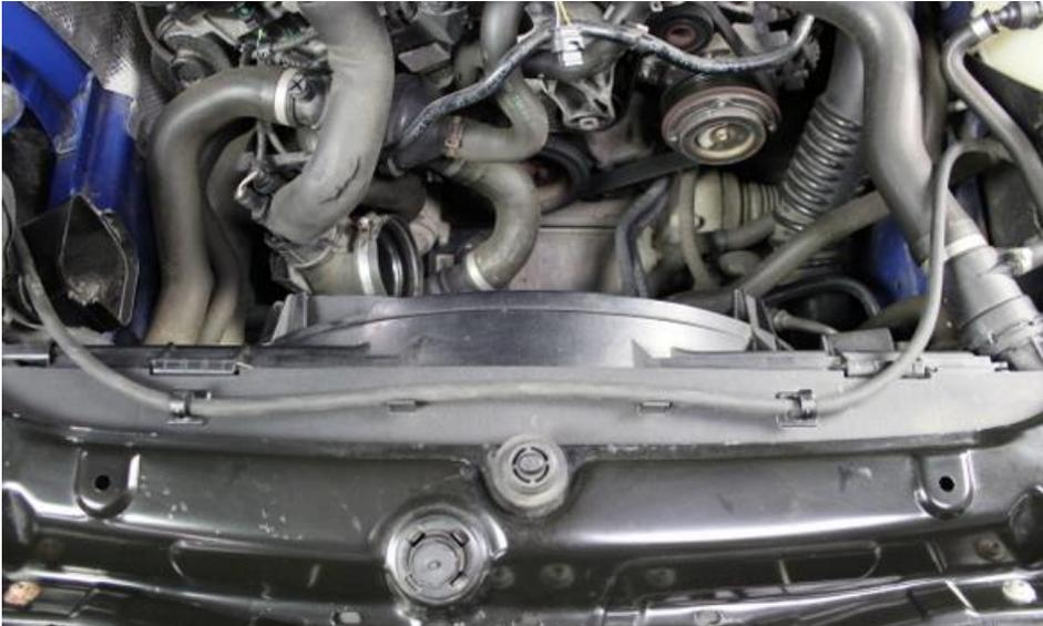
13. Route the hose removed from the airbox in step 3 over the fan and into the installed clips as shown.
