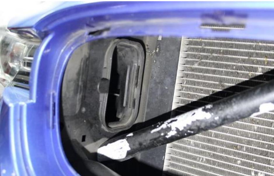
31. Remove the protective mesh inside the opening behind the grille. This is done by pulling the rubber tab and then taking the mesh out.
