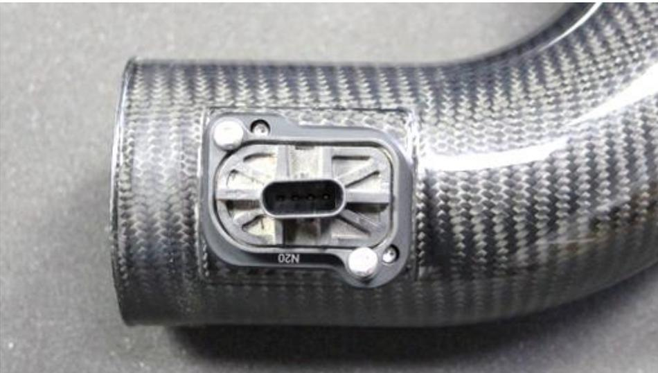
15. Install the sensor into the carbon tube – it must be installed in the correct orientation as shown. Secure with the 2 supplied Torx screws – NOT with the OEM screws.
