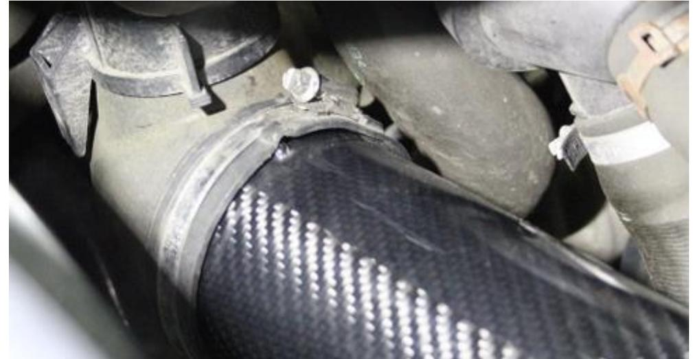
26. Push the carbon tube fully into the inlet hose – the notch on the carbon should go into the notch in the inlet hose. Secure the clamp around the hose.
