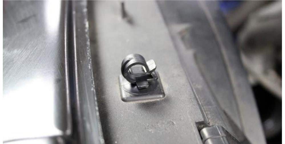
12. Push the clips in fully with the openings facing the engine as shown.
