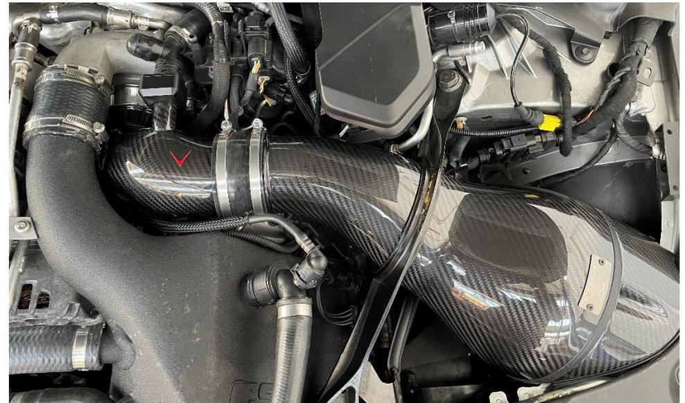
8. Now the intake can be installed back into place.
