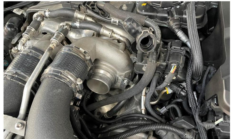
4. Remove the inlets from the turbos.
