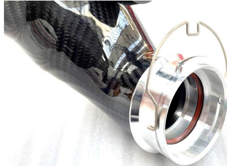
6. Insert the spring clip onto the machines flange with the top of the clip positioned over the raised section. Also insert the O-ring inside the flange as shown. The tapered face of the gasket should face the turbo.
