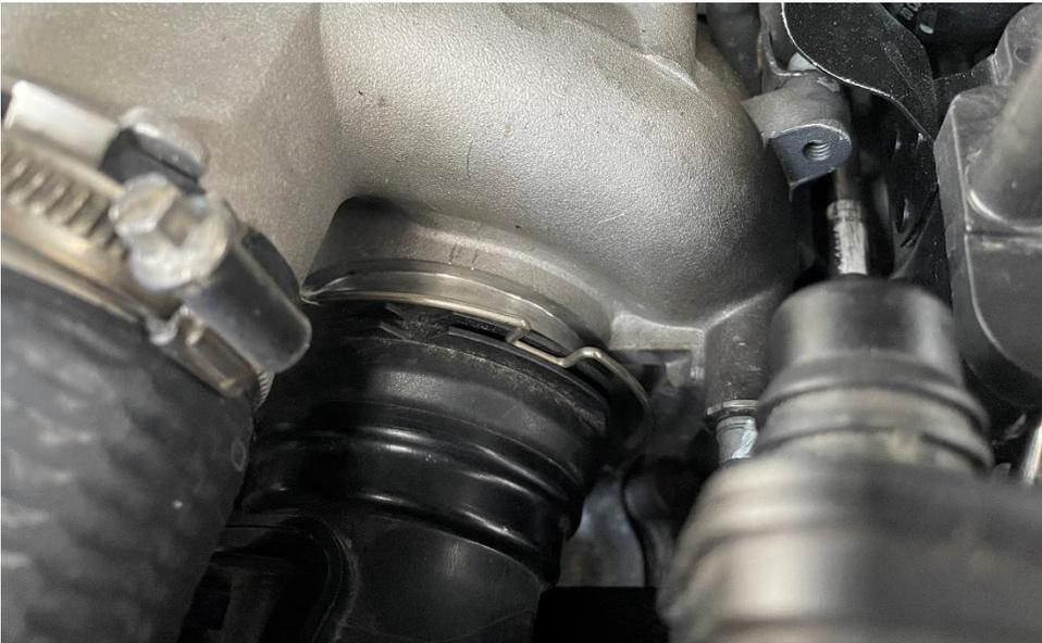
3. The inlets can be removed by pulling up the spring clips around the turbo flanges.
