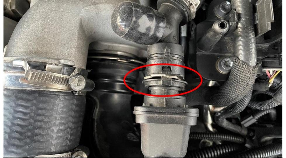
2. Pull up the spring clips holding the breather connectors to the inlets.
