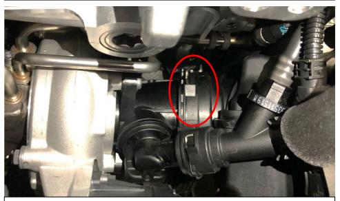
4. Pull the spring clip away from the tube flange and this will allow you to pull the tube away from the turbo. There is also a breather connector to remove – see next step.
