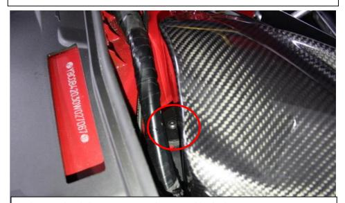
20. locate and push the top mount into the upper rubber bush.
