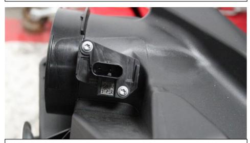
7. Remove the temperature sensor from the airbox.
