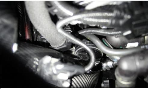
22. Secure the remaining hose clamp around the carbon tube – DO NOT overtighten.
