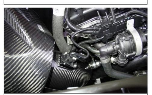
23. Connect the temperature sensor plug.
