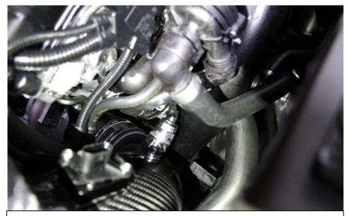
21. Rotate the tube into the silicon and connect the breather plug.
