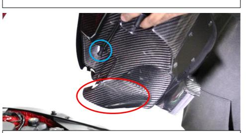
15. Carefully lower the airbox into the engine bay. Note that the secondary scoop circled above goes into the gap shown in the next photo. Also the mount circled blue should sit in the rubber mount shown in next photo.
