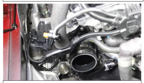
8. install the supplied silicon coupler onto the turbo inlet with the 2 hose clamps. Position the clamp screws so that they are accessible from the side as shown. See next photo for another angle.
