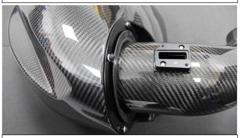
12. Insert the filter into the airbox and line up the holes on the sealing plate. Secure with the supplied M5 screws and lock washers.
