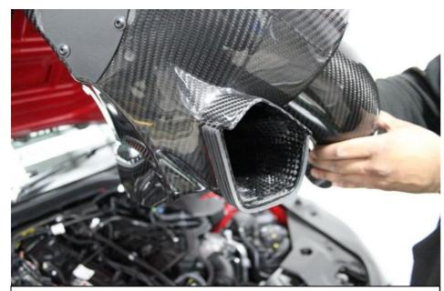
17. The main opening of the airbox should sit inside the stock duct – next photo.
