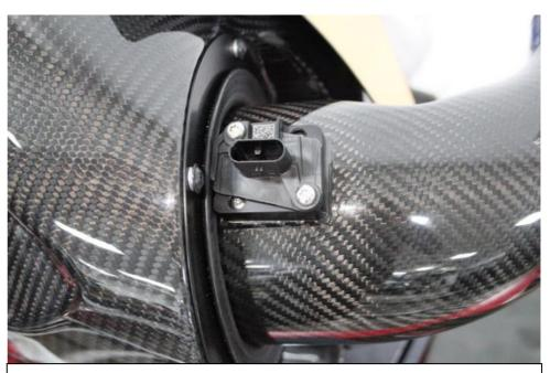
14. Install the temperature sensor onto the tube using the supplied screws. DO NOT use the stock screws.
