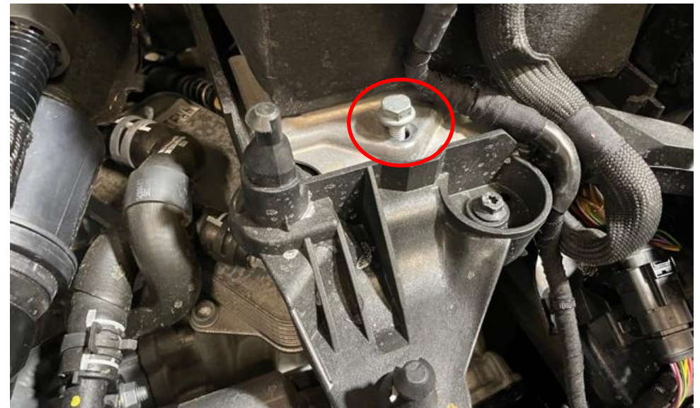
8. Remove the bolt holding the battery clamp down.
