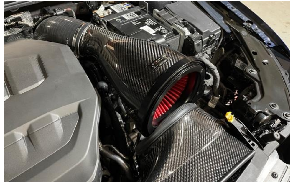
20. Push the filter housing into the silicon hose and lower it into place.
