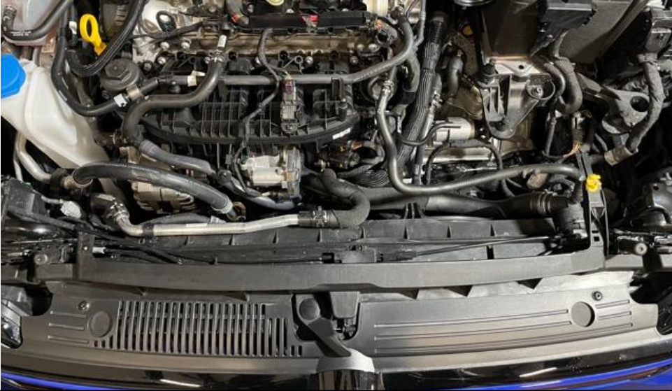
5. Remove the duct from the engine bay. Push it down to release the clips on each side. Also remove the engine cover.
