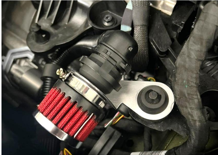
17. USA Golf Gti Only : Secure the bracket (grommet side) onto the airbox mount. Push down to secure.
