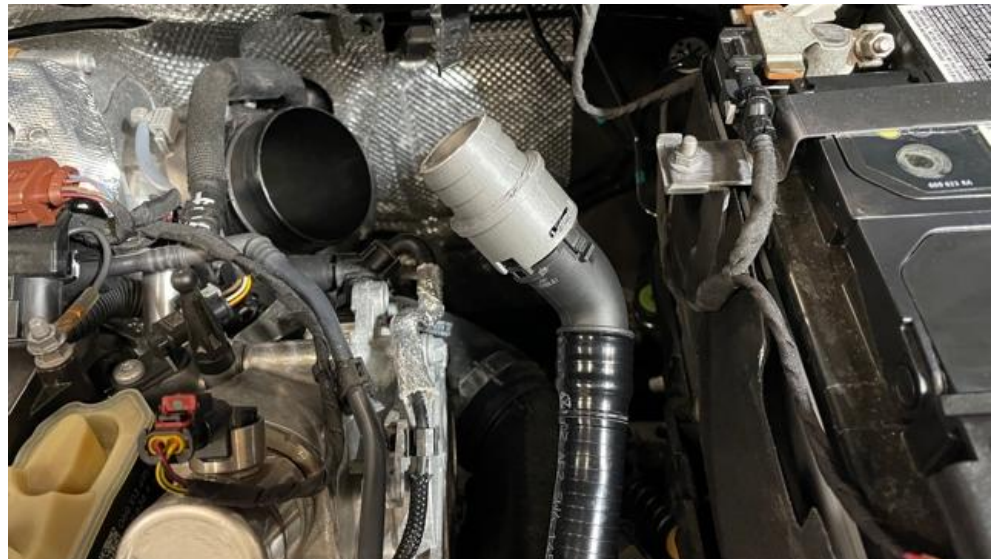
12. For the Golf R – take the machined adapter and clip it onto the bypass tube which was removed in step 7.
