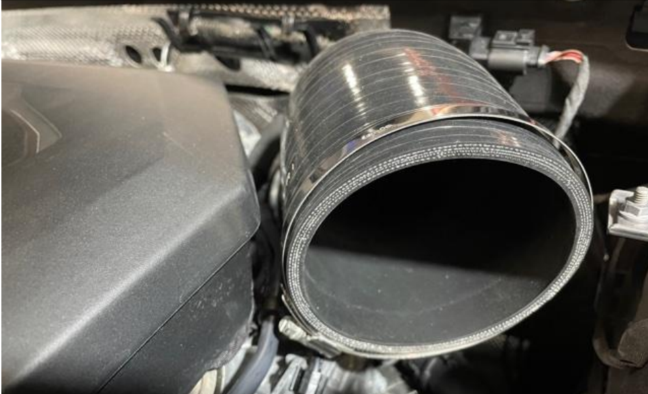
11. Place the engine cover back and rotate the hose to be almost touching the cover. Now tighten the clamp at the turbo side.
