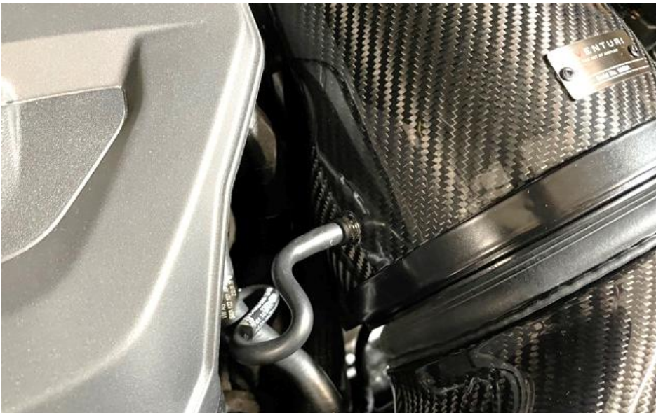
23. Push the vacuum hose onto the filter housing fitment.
