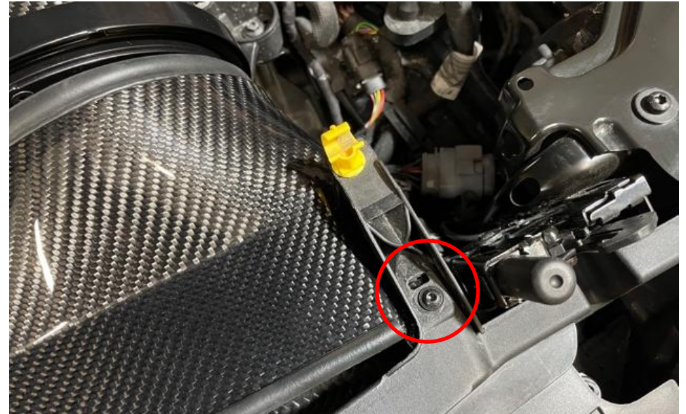
22. Secure the duct with the 2 x M5 screws provided. 1 Screw each side.
