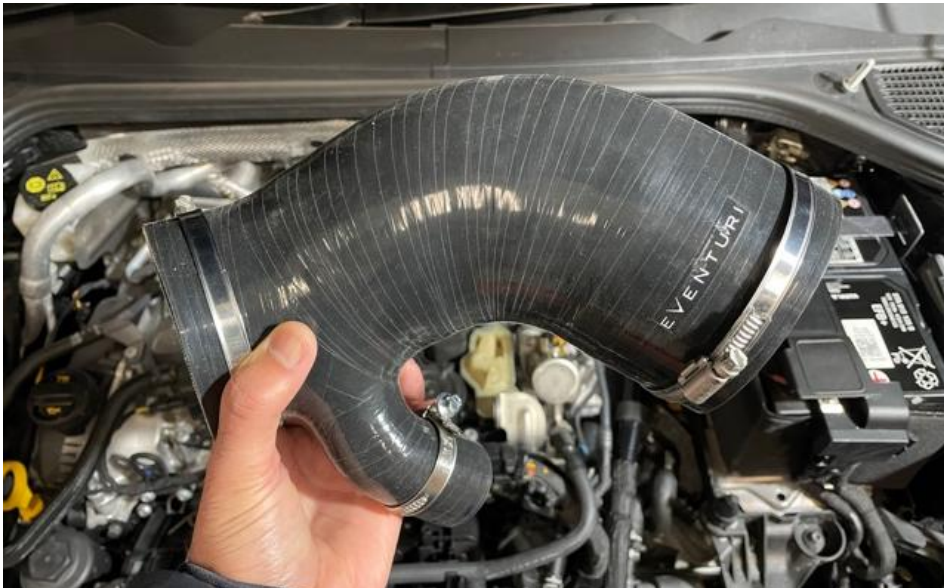
9. Take the new silicon with the hose clamp on each end. Golf R version shown.
