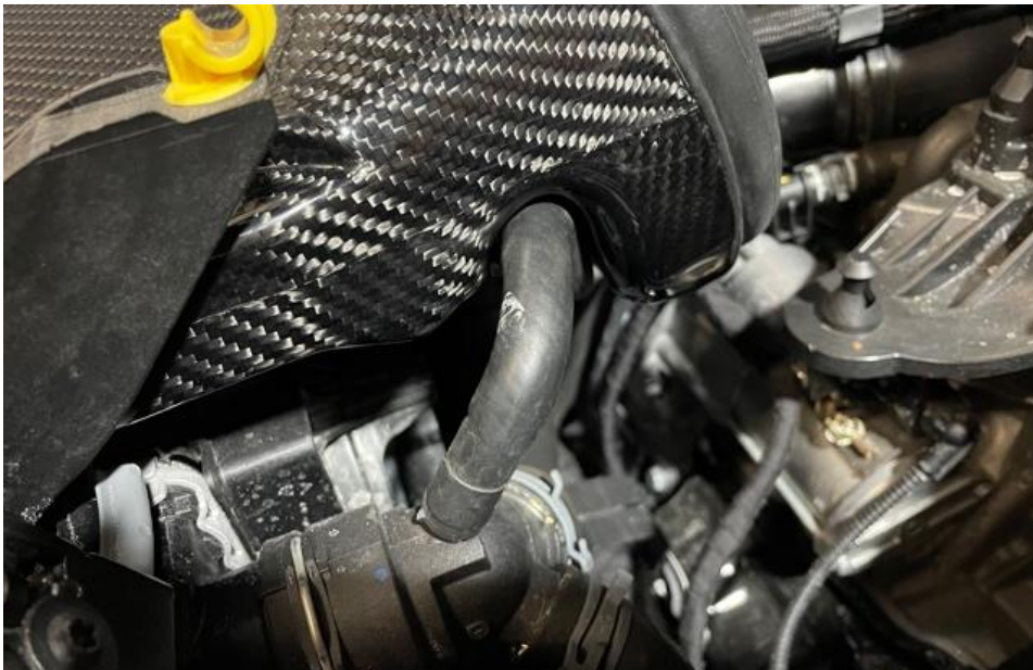
19. The coolant hose will sit inside the recess in the duct. Pull the hose away from the duct to avoid kinks and to give it more slack.
