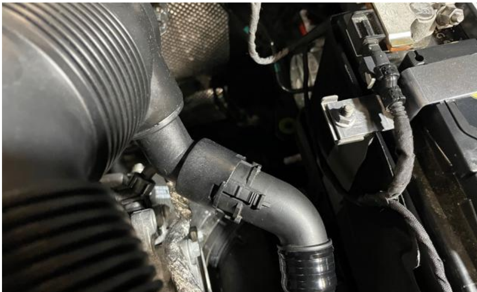
7. The Golf R has a secondary tube attached to the intake tube. Unclip and remove this from the intake tube.
