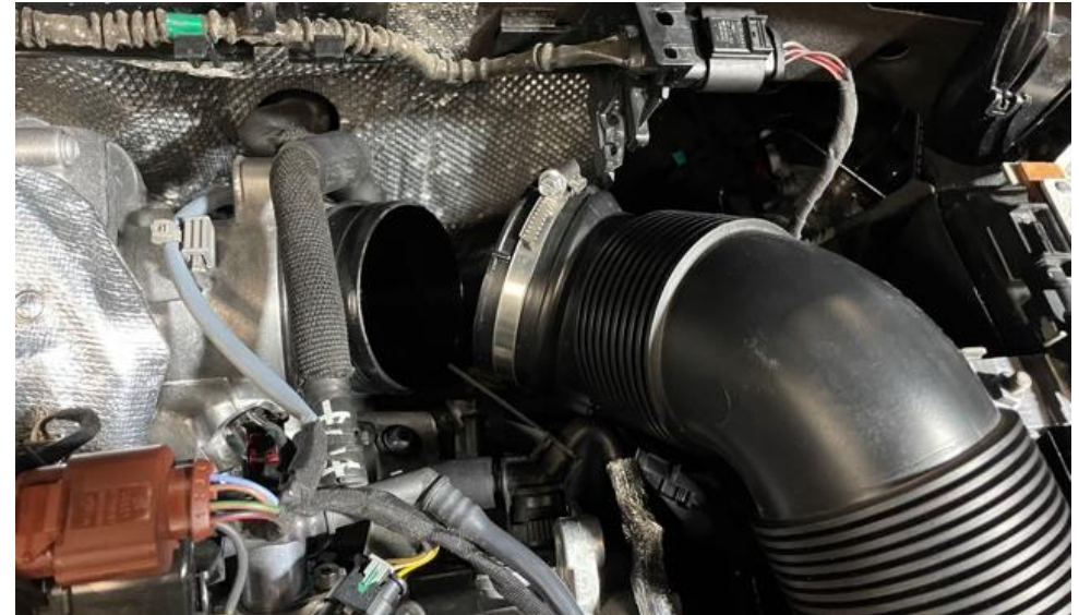
6. Remove the intake tube from the turbo inlet. (Golf R version shown)
