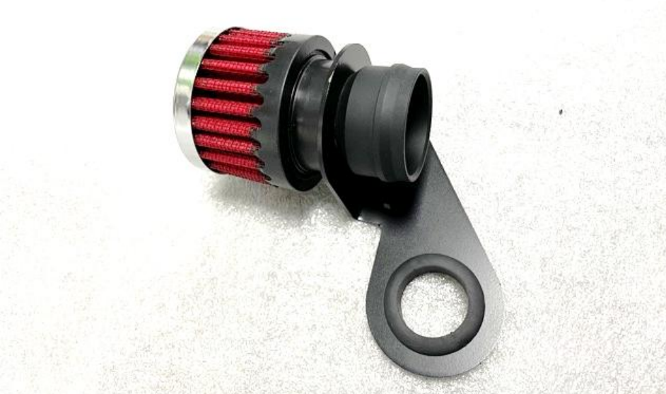
15. USA Golf Gti Only : Push the adapter through the bracket and then push the filter onto it from the other side as shown.
