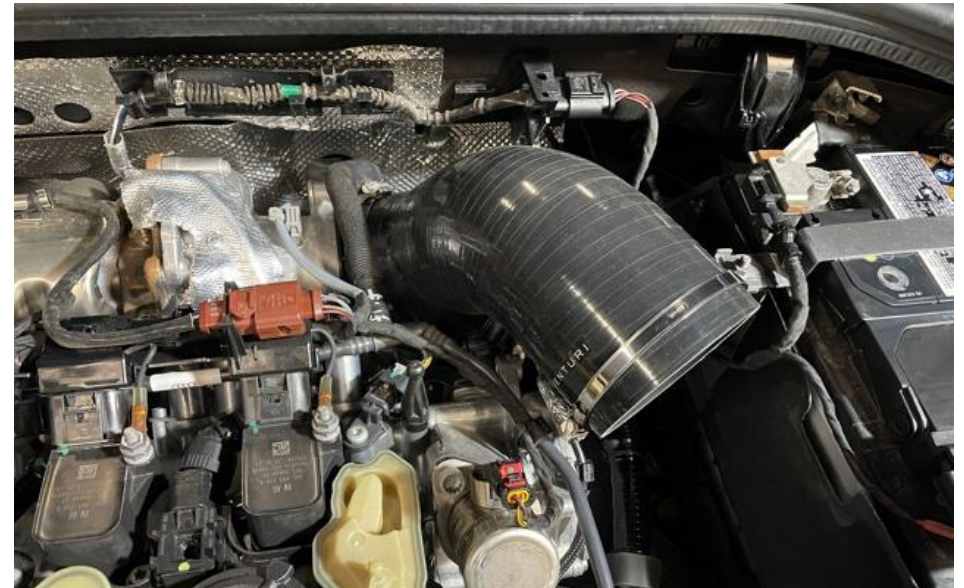
10. Install the silicon onto the turbo inlet.
