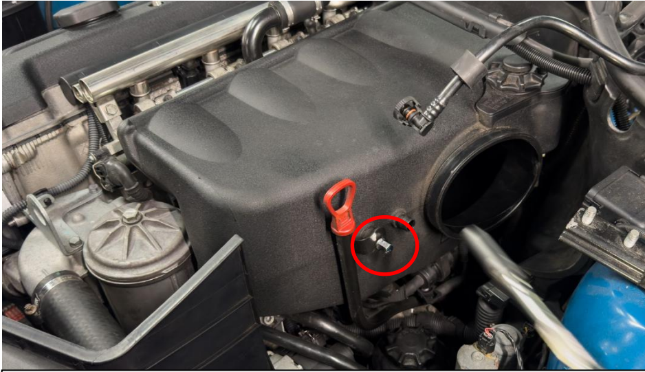
10. Remove the nut holding the oil dipstick to the manifold and move the dipstick away from the manifold for access.
