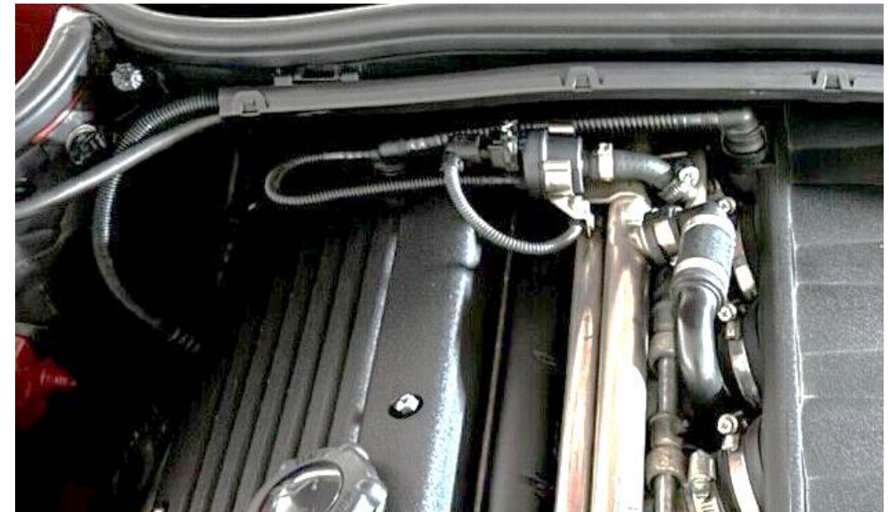
51. If your crankcase breather hose has a valve assembly as shown here then you need to extend the hose by cutting the existing hose off the breather connectors. See next page.
