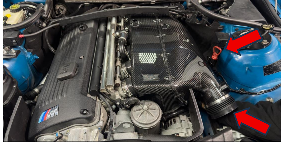
50. Push the remaining breather hose into place underneath the airbox and secure the mount. See next photo to see the breather location. Ignore the dipstick location – this is the E46.
