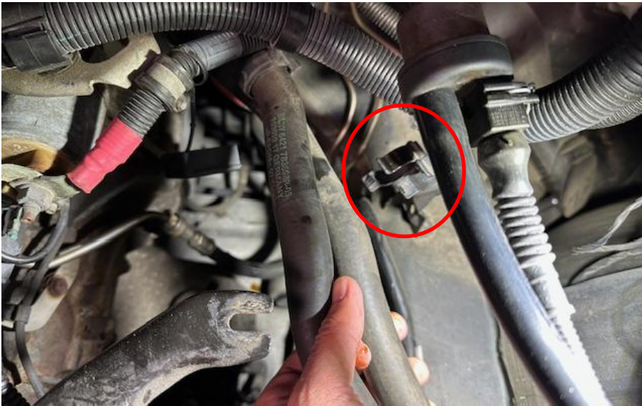
35. At the back of the engine bay, on the chassis you will see 2 pipes secured in the clip shown – remove them from the clip.
