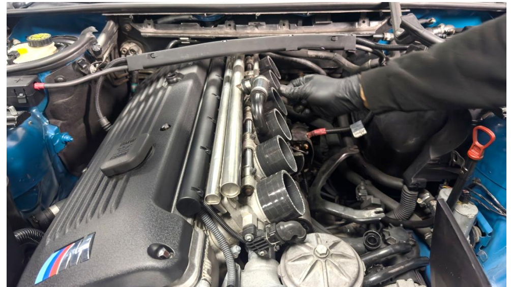
24. Push the new silicon couplers onto the throttle bodies.
