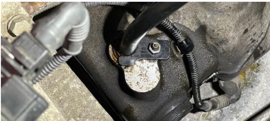
39. Push the dipstick into place and secure it with the plate removed earlier. Ensure the sealing washer is also in place.
