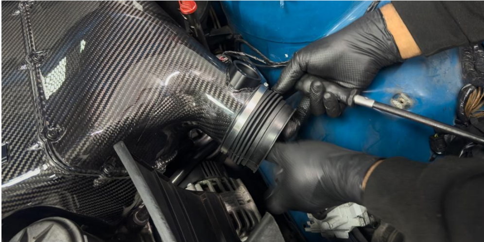
49. Push the flexible hose onto the carbon and secure with a hose clamp. Do not over tighten as you can damage the carbon. 2Nm is enough.
