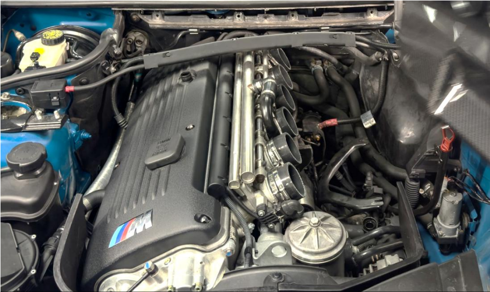
29. Place the second set of hose clamps over the silicons and make sure they are very loose.
