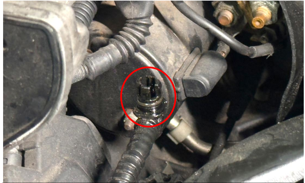
46. Push this breather into the airbox as removed from step 20.
