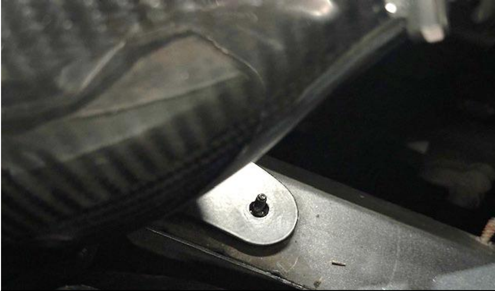
60. There is a bracket attached to the base of the heat shield – this should locate over the stud in the chassis as shown.
