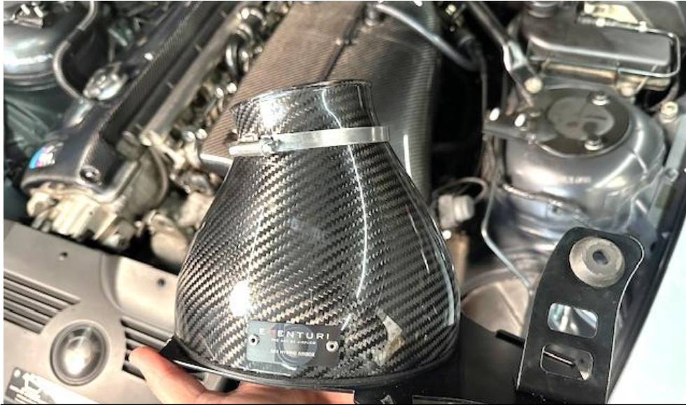
56. Place a hose clamp around the carbon housing loosely.
