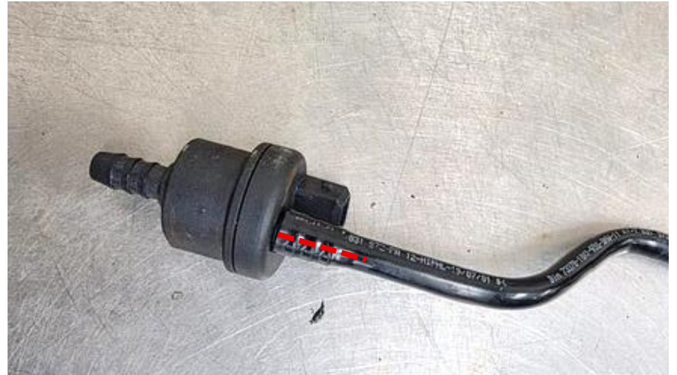
42. Remove the valve from the engine bay. Using a sharp knife, slice along the hard line attached to the valve as shown with the red line. This will allow you to remove the line from the valve.
