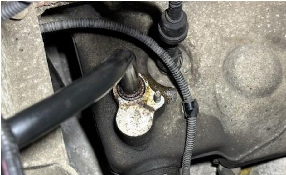
33. Securing plate removed.
