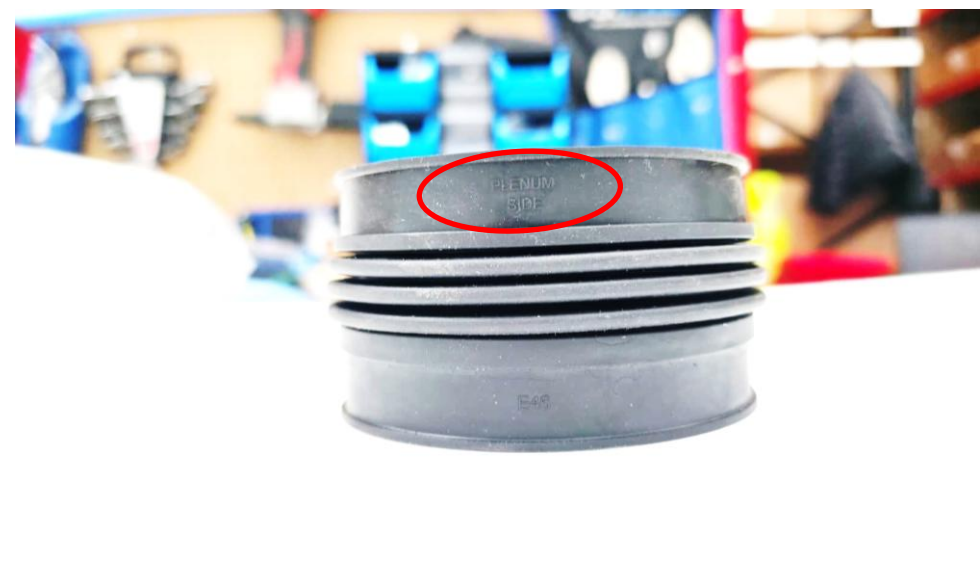
48. Take the flexible hose supplied and note the markings on each side. The side which is marked "PLENUM SIDE" should be pushed onto the carbon airbox.
