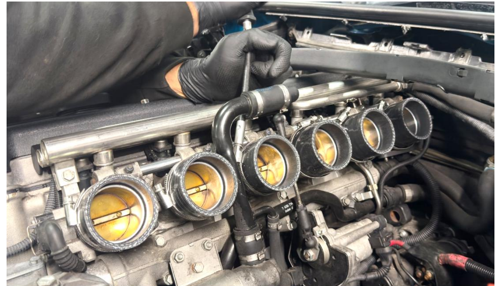
26. Make sure the heads of the clamps are positioned either to the side of the throttle bodies or you can rotate them to be underneath the throttle bodies.
