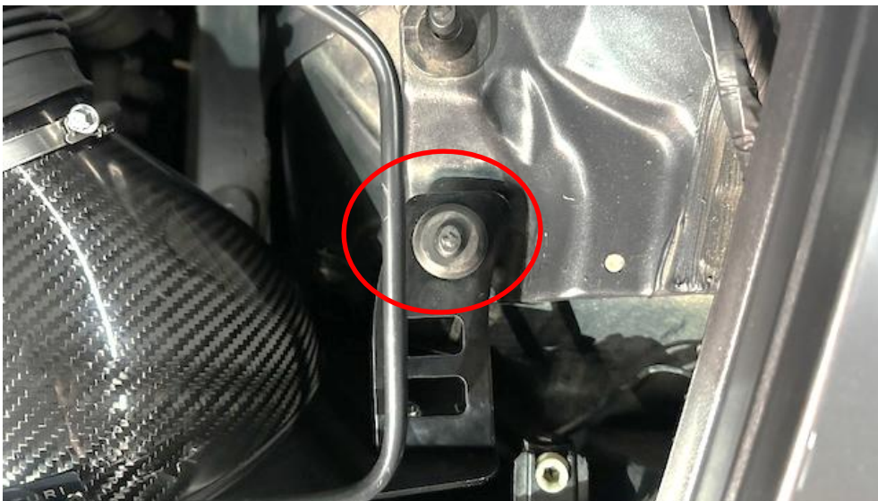
58. Push the rubber mount into position.
