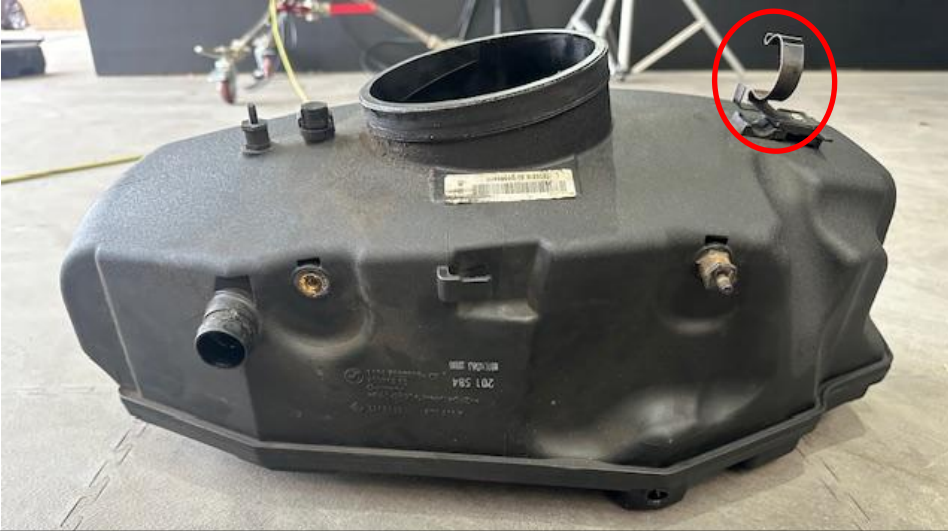
21. Remove the Breather module attached to the clip shown.
