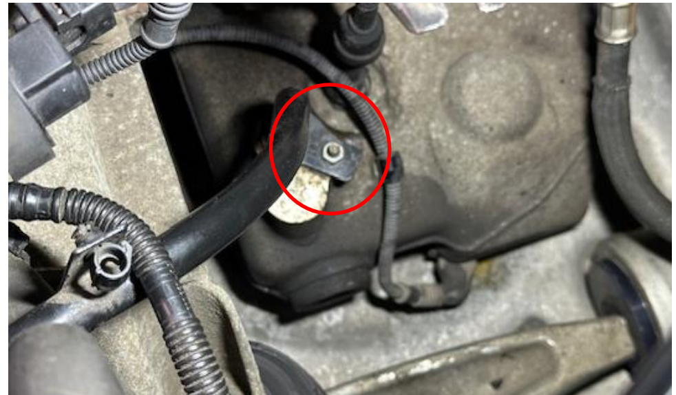
32. Remove the nut holding the securing plate onto the base of the dipstick. Then remove the securing plate. See next image.
