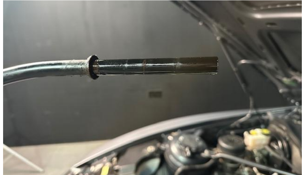
34. Remove the dipstick – be careful to also remove the washer from the dipstick. It may be stuck to the securing plate or the engine.
