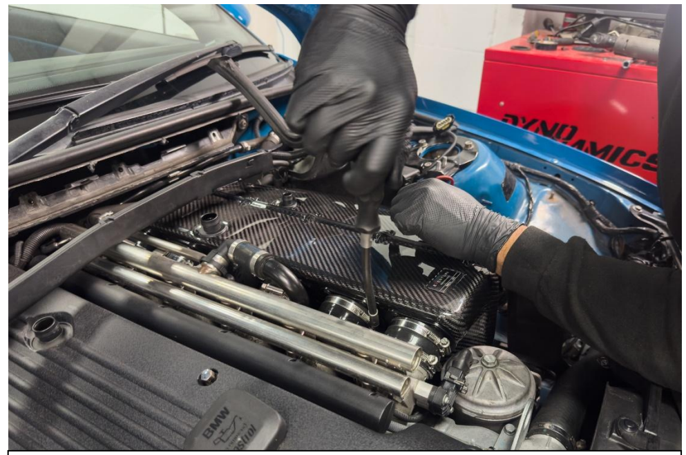
47. Making sure the airbox us fully pushed into the silicons, secure the hose clamps around the trumpets. They only need to be hand tight.
