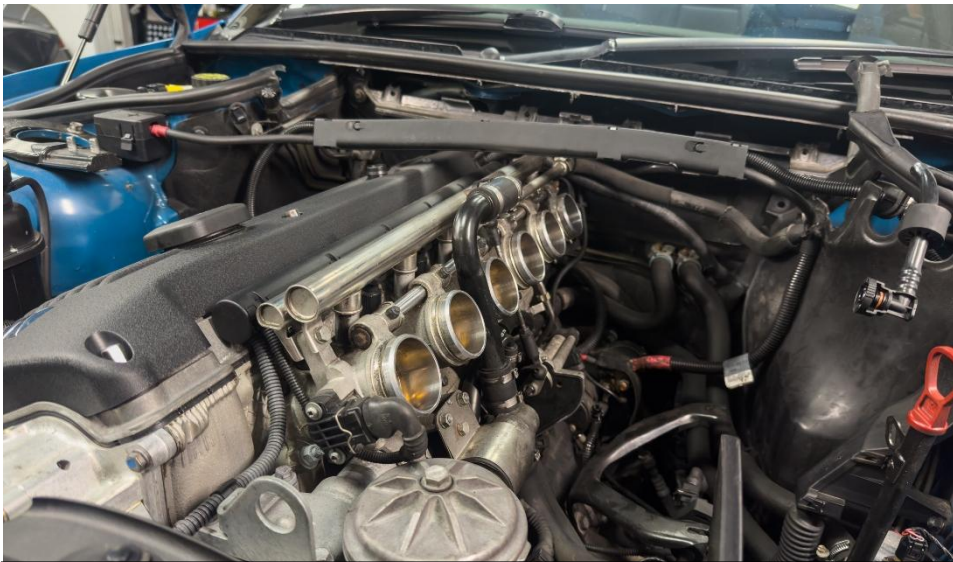
23. Plenum removed from the engine.
