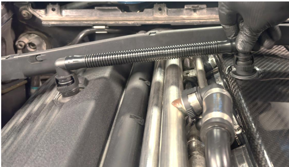
50. Use the new extended crankcase breather hose as supplied in the kit to connect the crankcase to the airbox. Note – the appearance of the tube may vary.
