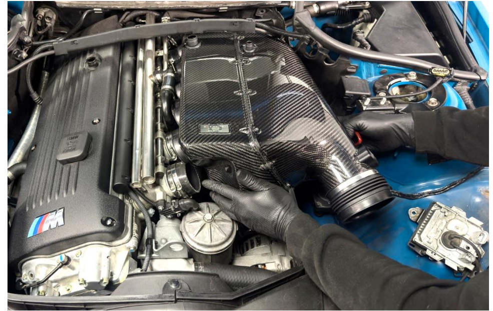
44c. Place the carbon airbox into position.
