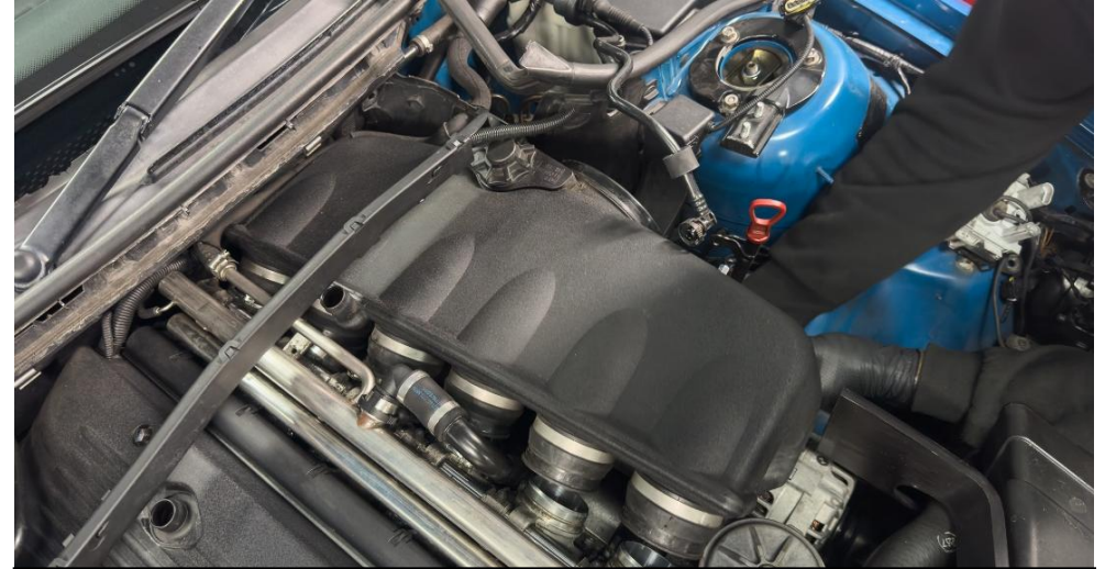
22. With all 6 clamps removed pull the plenum away from the engine and lift up to allow access to the base. Now you can remove the remaining breather hose by pulling it away from the plenum. It will unclip as you pull it out.
