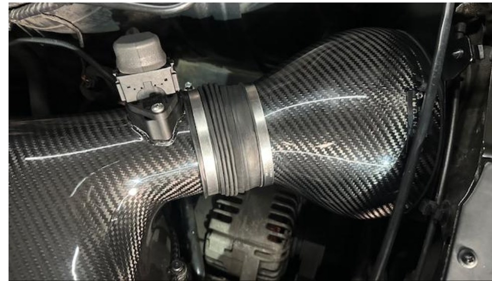
59. Pull the flexible coupler around the housing and then tighten it with the hose clamp. Do not over tighten. 2Nm is enough. Also reconnect the MAF sensor plug.
