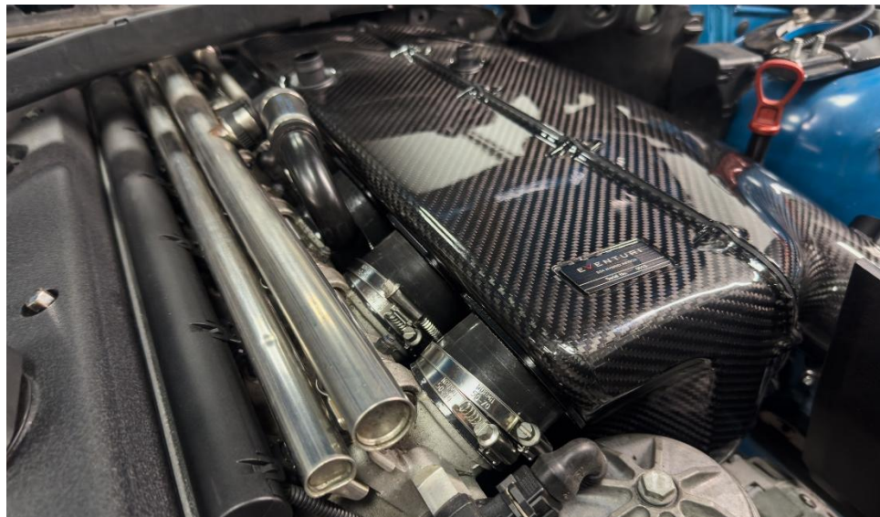
47. Push the airbox into the silicon couplers. The OEM vibration mount installed to the airbox should slot onto the OEM bracket.
