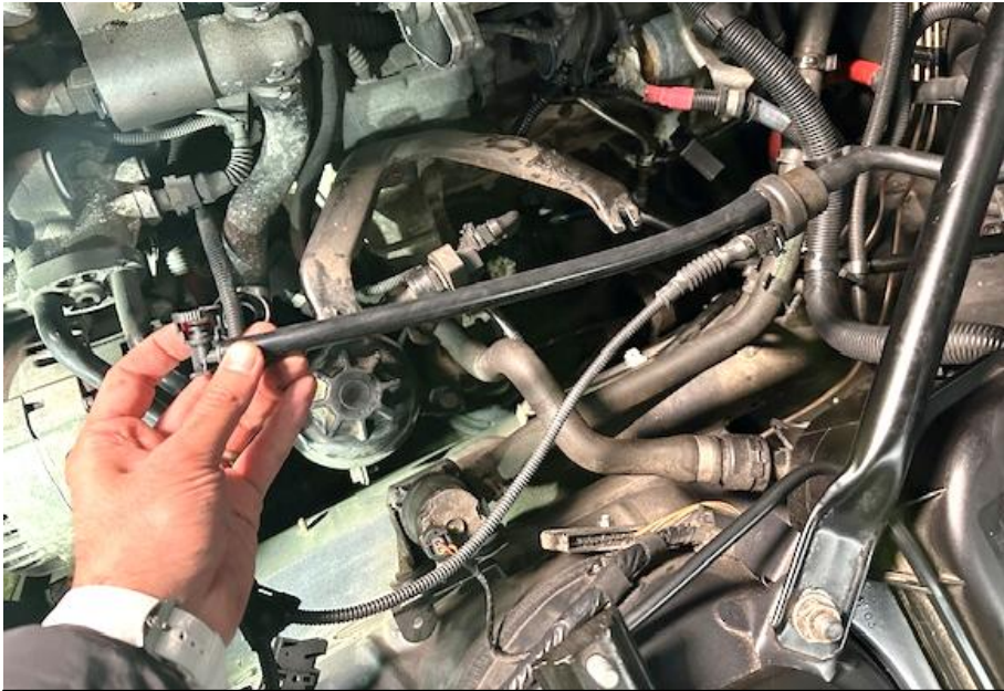
44b. Push the vacuum line onto the module and point the clip towards the engine as shown.
