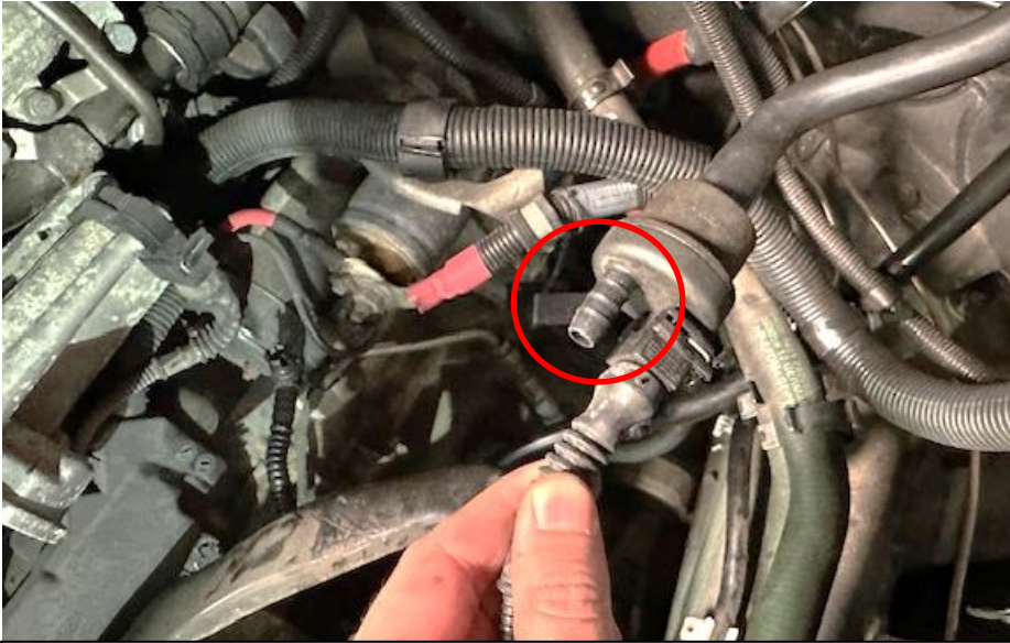
41. Remove the breather hose from the module shown. You may need to cut it off. This breather hose went to the OEM intake elbow.
