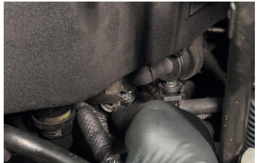
13. Remove the 10mm nut from underneath the mounting point using a spanner.
