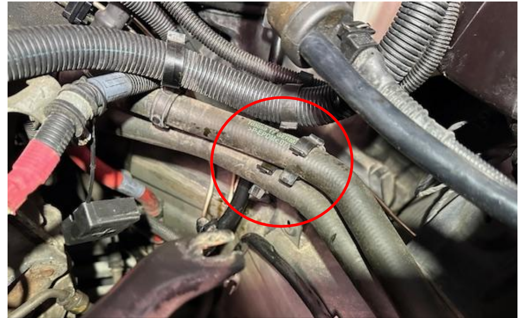
38. With the dipstick relocated, push the hoses back into the clips.
