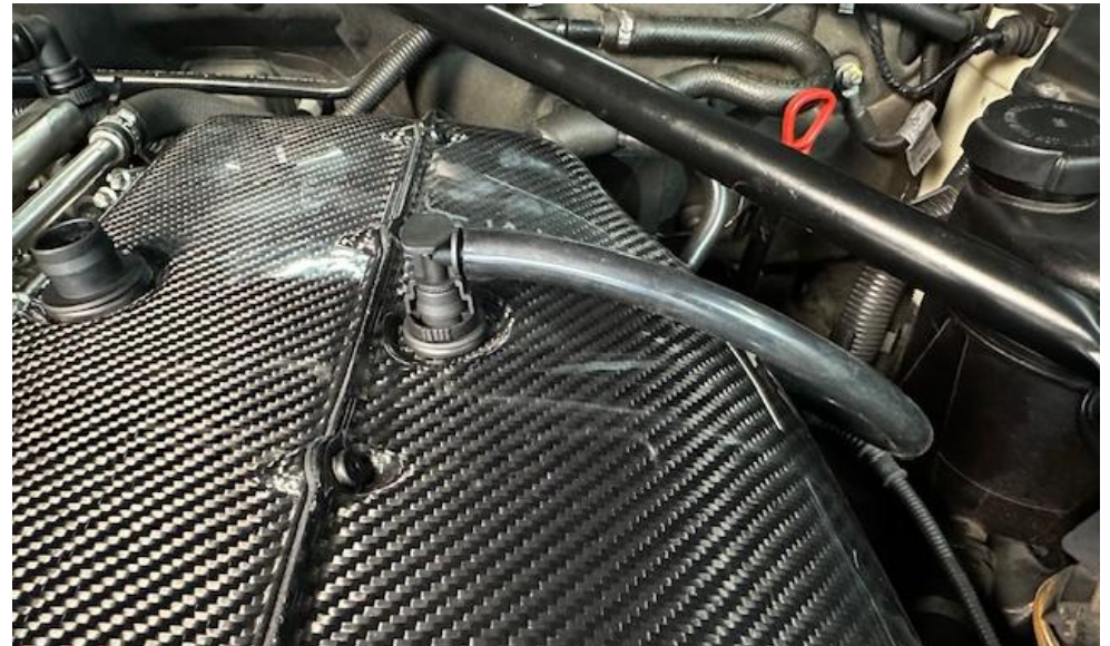
49. Push the clip into the top of the airbox.
