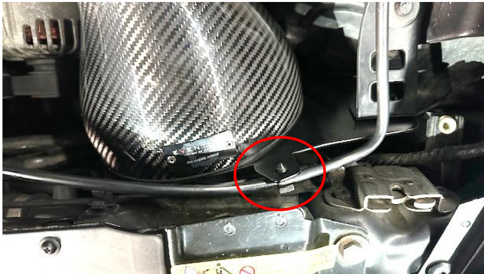
62. Clip the coolant line into the clip on the heat shield.
