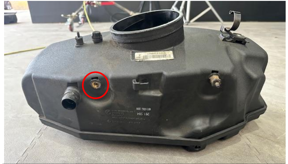
30. Remove one of the vibration mounts from the OEM plenum and transfer it to the base of the carbon airbox. The carbon airbox only has one threaded hole and only requires 1 mount.
