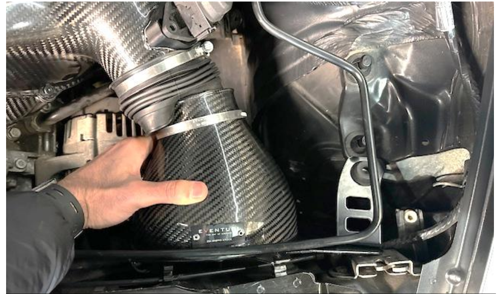
57. Carefully push it down into position. Lift the coolant line over the housing.
