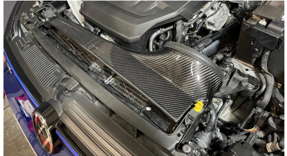
18. Place the new duct into position. The coolant hose goes UNDER the duct – see next step.
