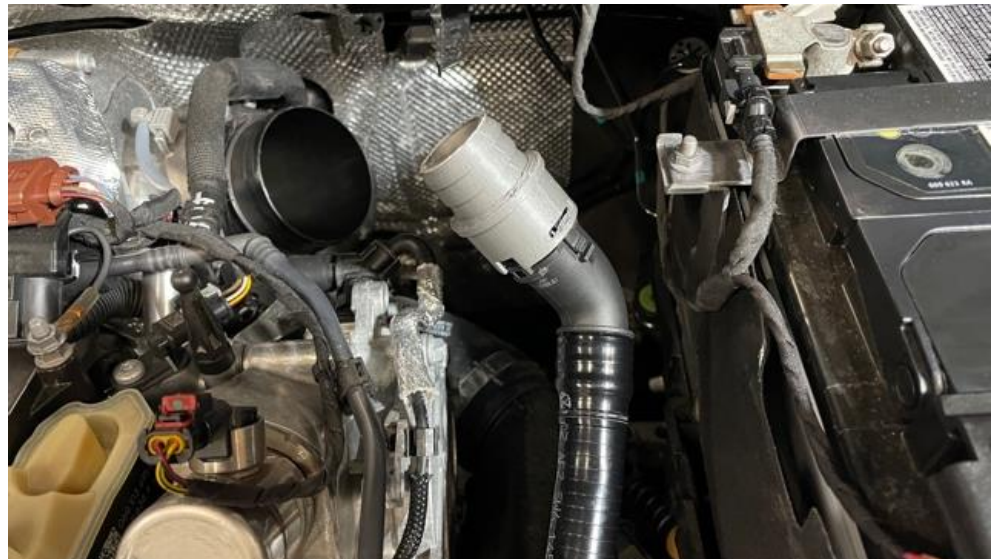
12. Take the machined adapter and clip it onto the bypass tube which was removed in step 7.
