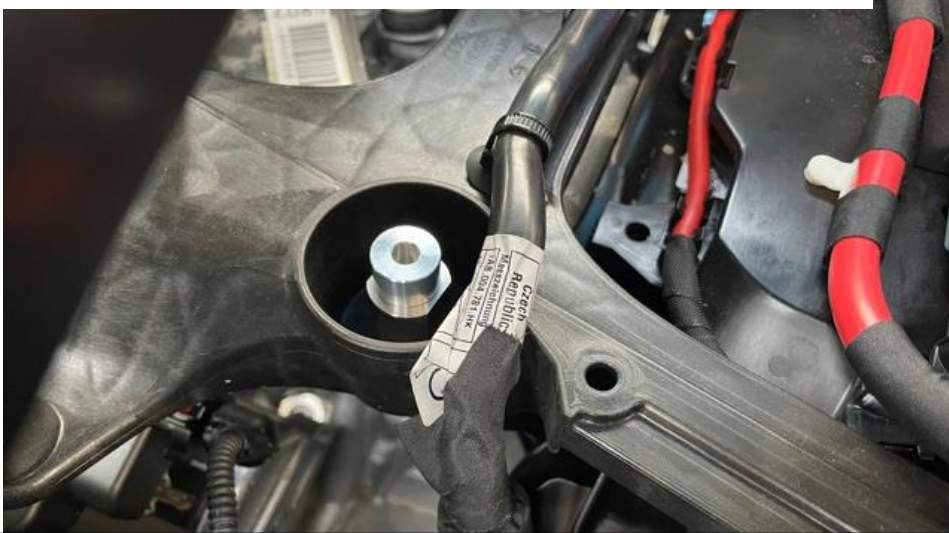
17. For the TTS – use the extra spacer to bring the mounting area level with the top of the panel.
