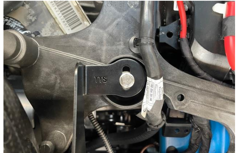
21b. IF your battery is NOT in the engine bay, secure the bracket with the provided M6 screw as shown. Please note – the bracket shape may be different to that shown.
