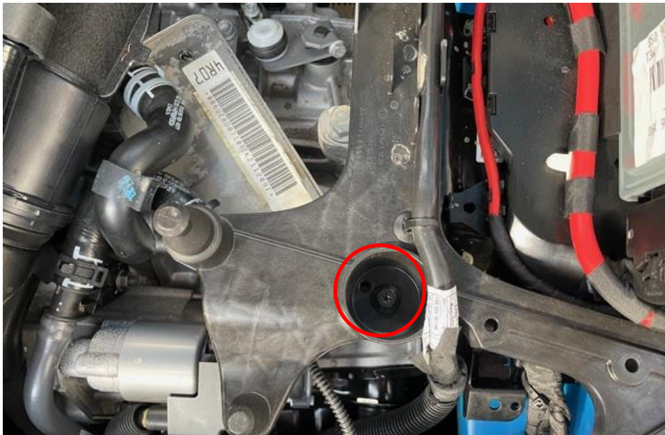
15. Remove the screw shown – this is where the intake will mount to. (ONLY FOR CARS WHERE THE BATTERY IS NOT IN THE ENGINE BAY)
