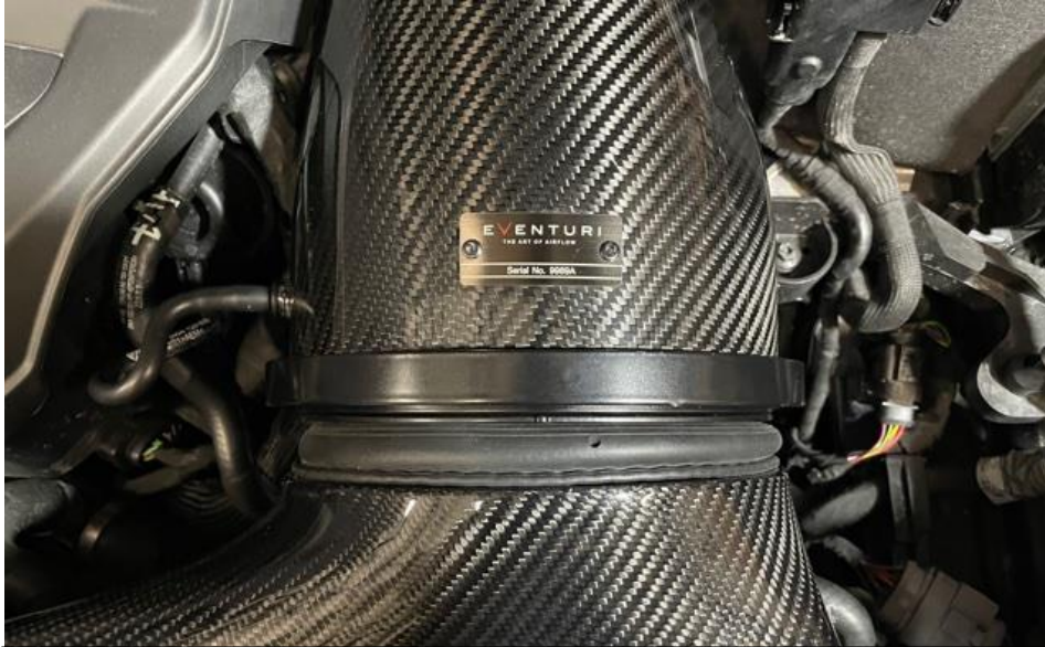
24. Filter housing should sit squarely with the duct. If it does not – the rear silicon needs to be rotated accordingly.
