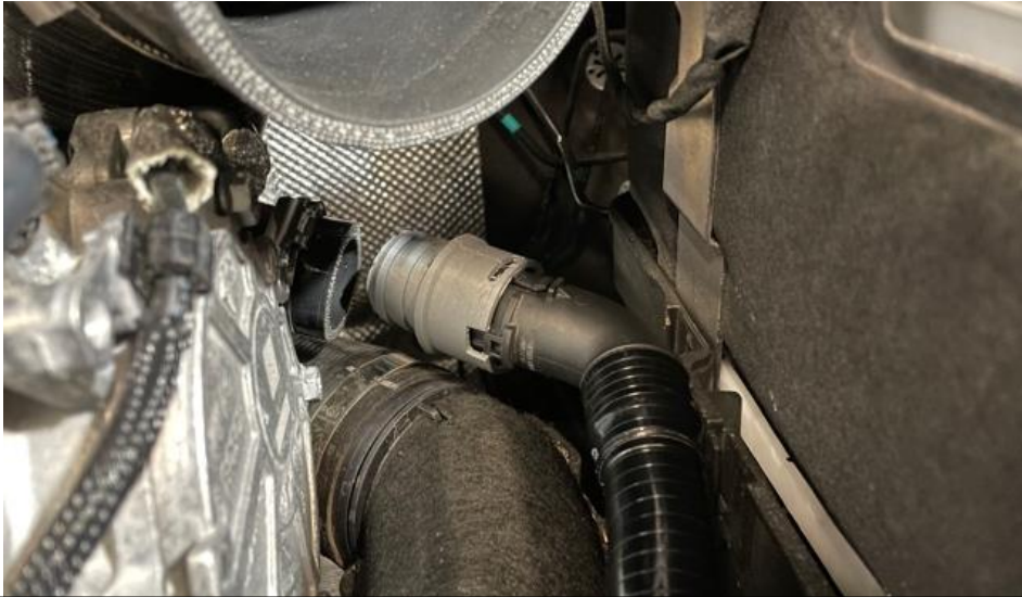
13. Now push the fitment into the silicon hose
