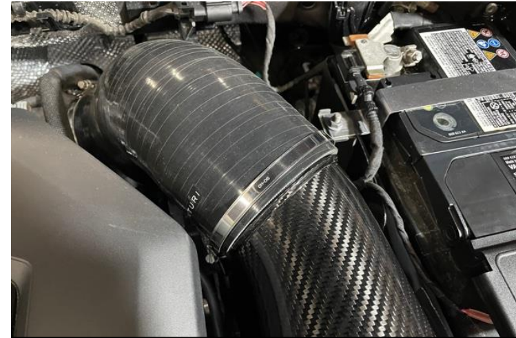
25. Tighten the remaining hose clamp – do not overtighten around the carbon.
