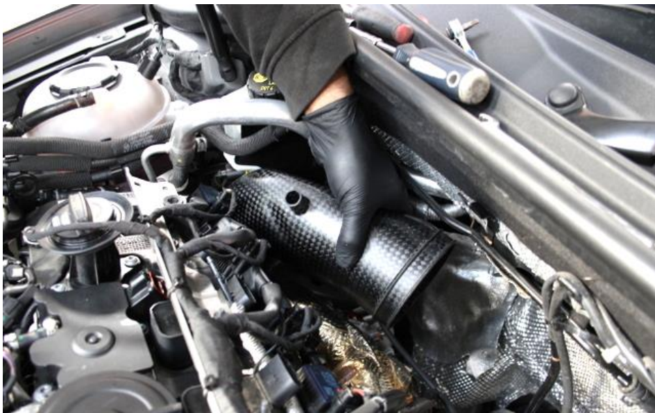
17. Rotate it around the manifold heat shield.
