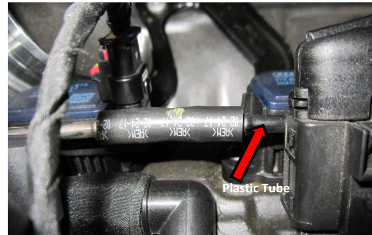
6. Remove the vacuum line from the plastic tube which is between the coil packs.
