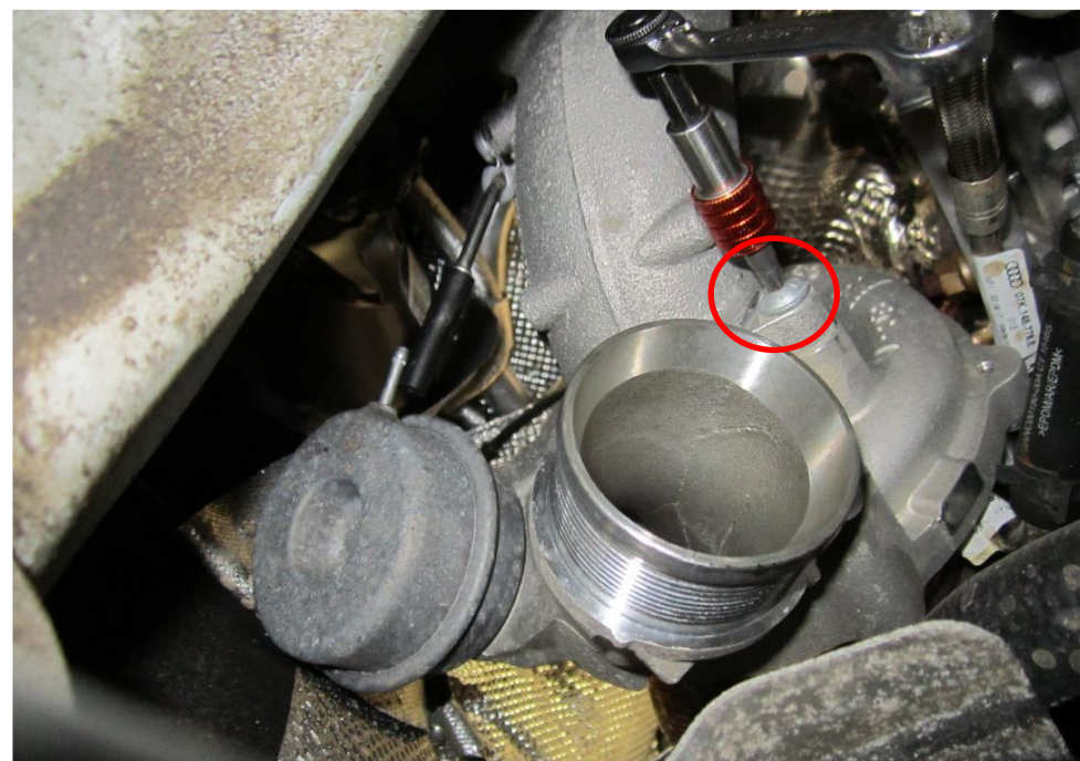
8. Now remove the stock turbo inlet. There are 2 x T30 Torx screws holding it in place. One on each side of the tube.
