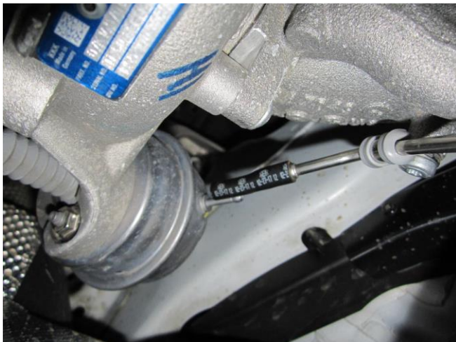
5. Remove the vacuum tube from the actuator.
