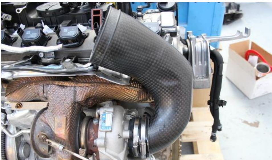
19. Push the inlet tube firmly into the silicon and ensure it is fully in. Do not tighten the clamp yet. (Hose clamps shown here were updated to the V Band clamp)
