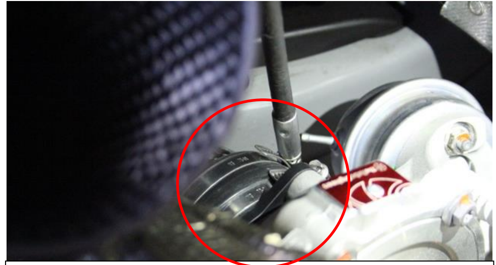
26. Ensure the Carbon tube is still fully engaged in the lower silicon coupler and tighten the hose clamp around the lower silicon. Do not over tighten this with a ratchet. It only needs to be finger tight as the silicon provides a good seal. (Hose clamps shown here were updated to the V Band clamp)
