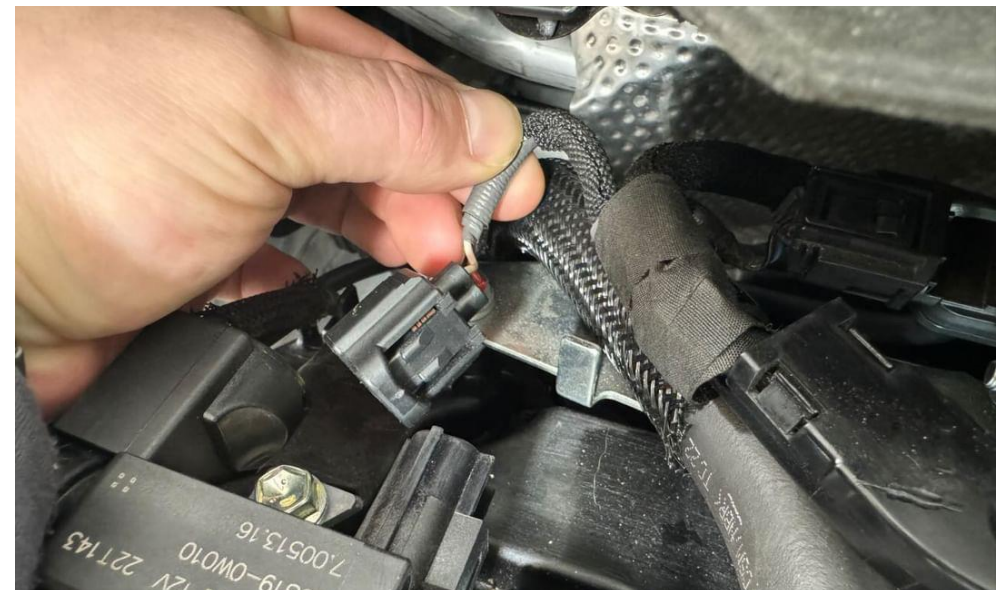
44. Disconnect the connector which goes over the PCV hose at the rear.
