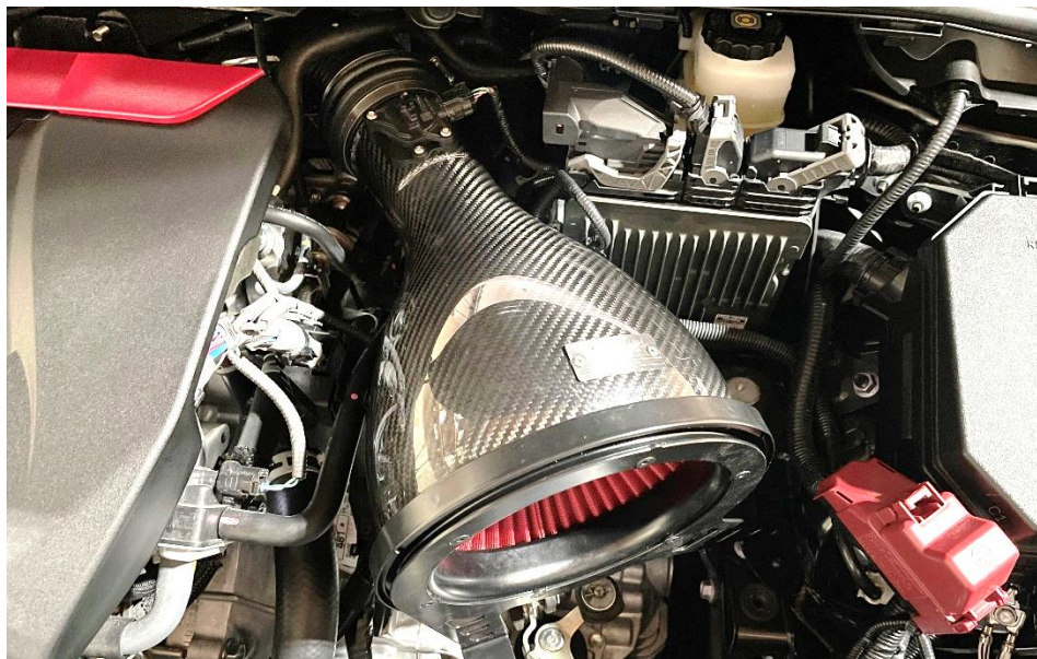
23. Insert the carbon housing into the flexible hose – DO NOT tighten it yet.
