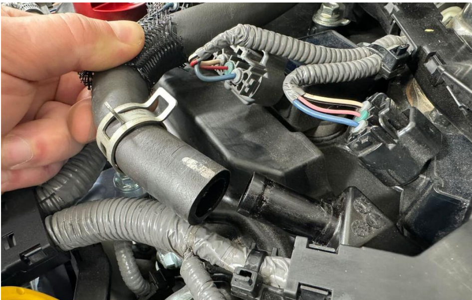
43. Disconnect OEM hose from the valve cover.
