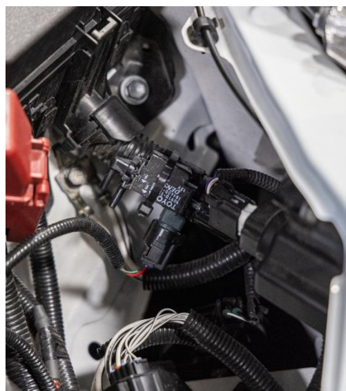
7. Remove all hoses from the vacuum module and resecure the module within the engine bay.
