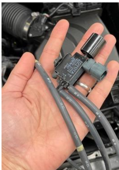
7. Remove all hoses from the vacuum module and resecure the module within the engine bay.
