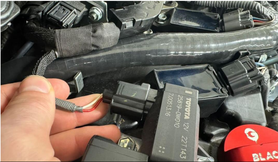
49. Reconnect the connector crossing the hose at the rear.
