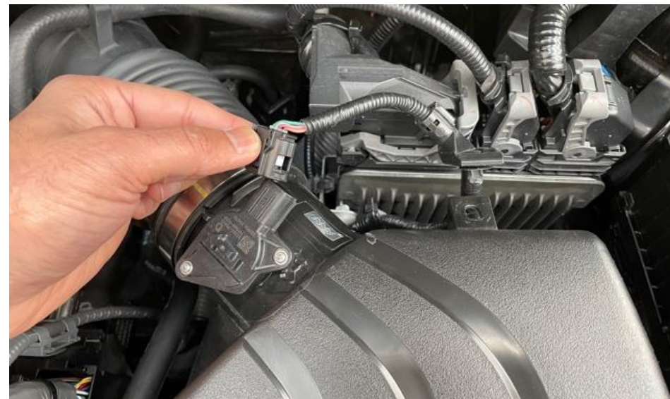
8. Disconnect the MAF sensor plug – make sure the ignition is OFF.
