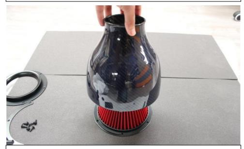
${\bf 8. \ Line \ up \ and \ place \ carbon \ housing \ over \ filter.}$
