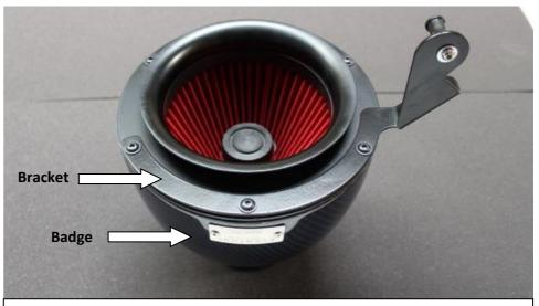
2. If there is a bracket attached – make note of the position of this bracket with respect to the Eventuri Badge. Take a photo for easy reference. You will need to reinstall the bracket in the same position.
