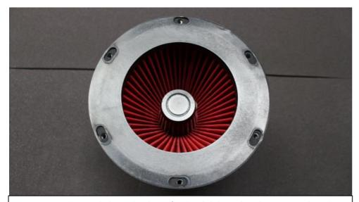
9. Turn over and ensure holes are lined up – if gasket slightly overlaps the inserts on the carbon it is ok.
