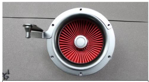
10. Place the Cowl and bracket back on the filter. Bracket must be IN THE SAME POSITION as it was originally.
