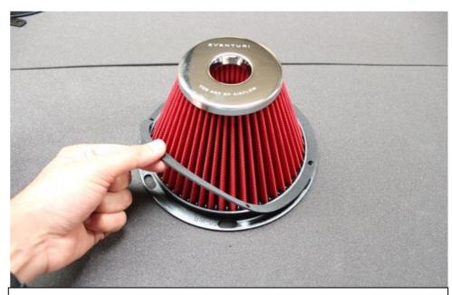
6. Place new gasket around the new filter – line up the holes with the filter holes.
