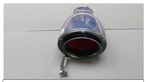
1. If you have this type of filter housing where there are 6 screws in the front face (with or without a bracket) then you have a Filter called a "190 Filter". Please follow these steps for replacement.
