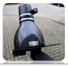
12. Insert the MAF tube into the silicon joiner. The tube must be oriented so that the MAF sensor opening as shown previously is facing into the carbon housing.
