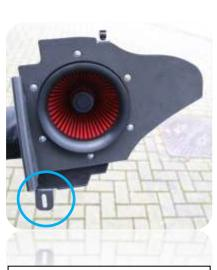
14. The mounting bracket on the heat shield as shown locates onto the bolt from step 7.
