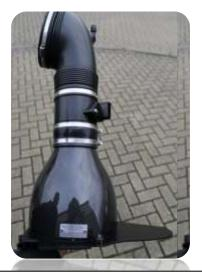
13. Rotate the MAF tube 45 degrees as shown and tighten hose clamps over silicon. Insert the OEM elbow over the MAF tube but do not tighten this yet.
