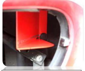
23. Insert supplied plastic push clips and firmly push in the heads so that they click into place and lock the scoop. Re-install the grill.
