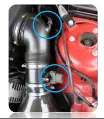
18. Push MAF connector onto MAF sensor firmly until it clicks into place.Push the breather hose onto the back of the elbow.
