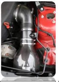
15. Lower the intake into the engine bay and locate the mounting bracket into the bolt from step 7. Do not tighten yet.
