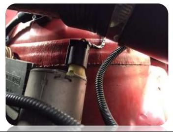
16. Push elbow onto the manifold. Take care that the rubber gasket remains in position. The elbow will be oriented slightly downwards than the original position. Allow some clearance under the elbow for the water pump connector. Tighten both elbow hose clamps.
