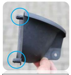
21. Photo showing plastic push clips which secure the original duct in place.
