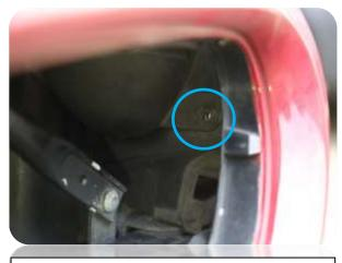
20. Remove duct by firstly removing plastic screw/rivet from the leading corner as circled. The duct can now be pulled out – it is held in place with 2 push clips at the back as shown in the next photo.
