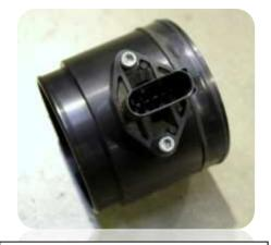
9. Push the MAF Sensor with its original O-Ring into the new MAF tube. Make sure the sensor is correctly oriented to match the shape of the boss. Secure with supplied bolts.
