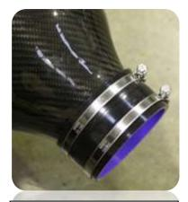
10. Push Silicon joiner onto carbon fibre housing.
