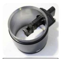
11. The front of the MAF sensor has a small opening as shown above. This is the side which should face into the carbon housing.
