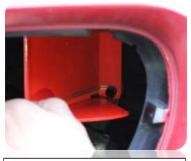
22. Put new scoop in place by lining up the mounting holes to the back panel where the original duct was secured.
