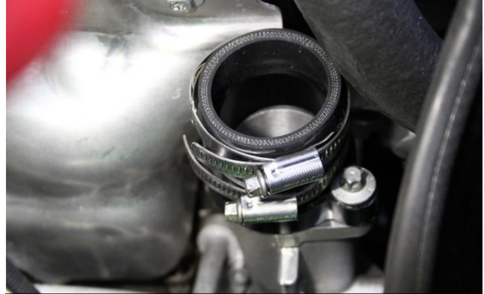
10. Install the smaller hose clamps (40-60mm) onto the silicons. Make sure the clamps do not interfere with the screw - face them away as shown. Tighten the clamps around the flange.
