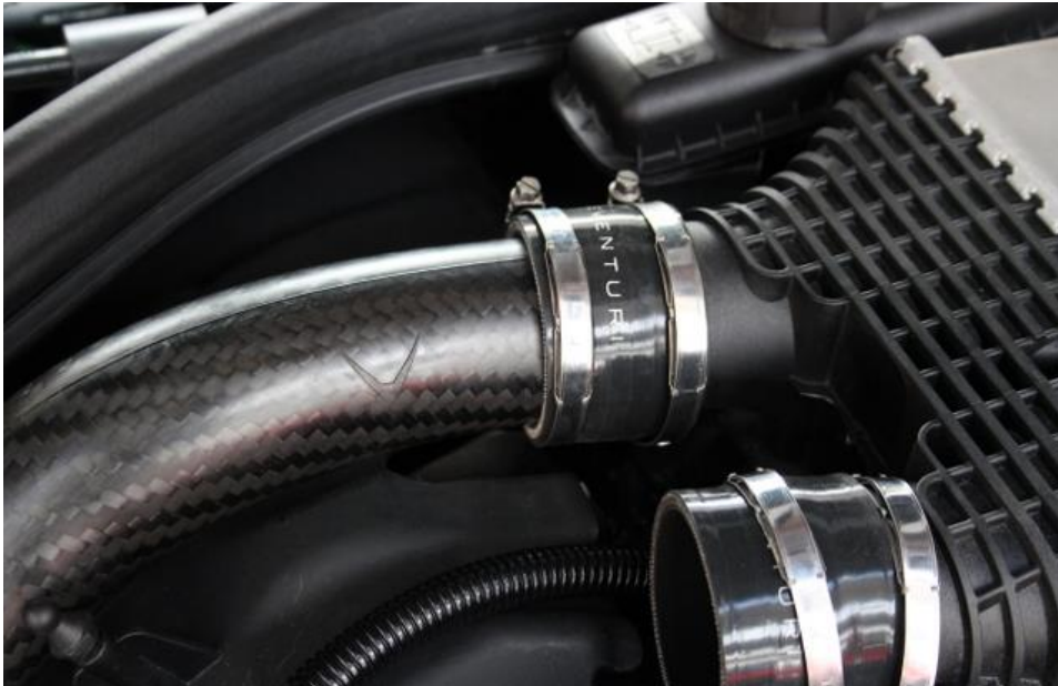
13. Now push into the upper silicons. For easier access you can loosen the charge cooler and lift it slightly.
