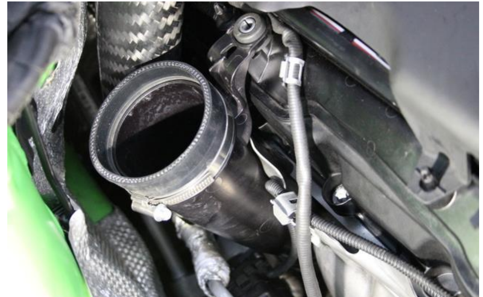
14. Install the turbo inlet tube again and secure with the OEM screw.
