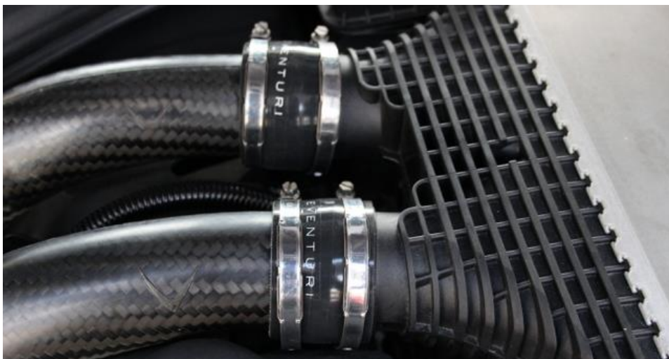
15. Install both chargepipes and tighten all clamps.
