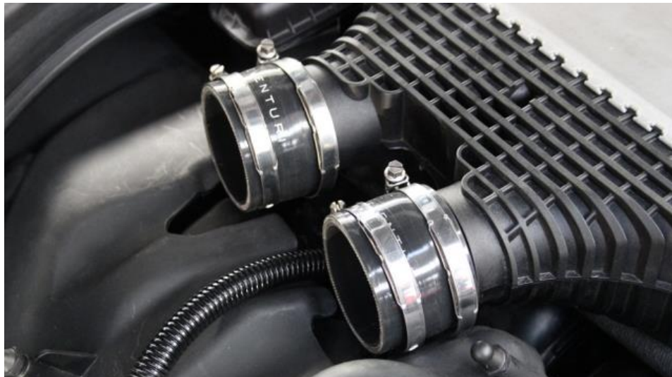
11. Push the larger silicons onto the charge cooler with the larger hose clamps. Tighten the clamps around the cooler.
