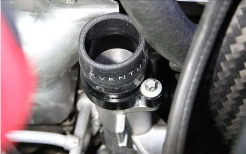
9. Push the smaller silicon couplers onto the flanges all the way down.
