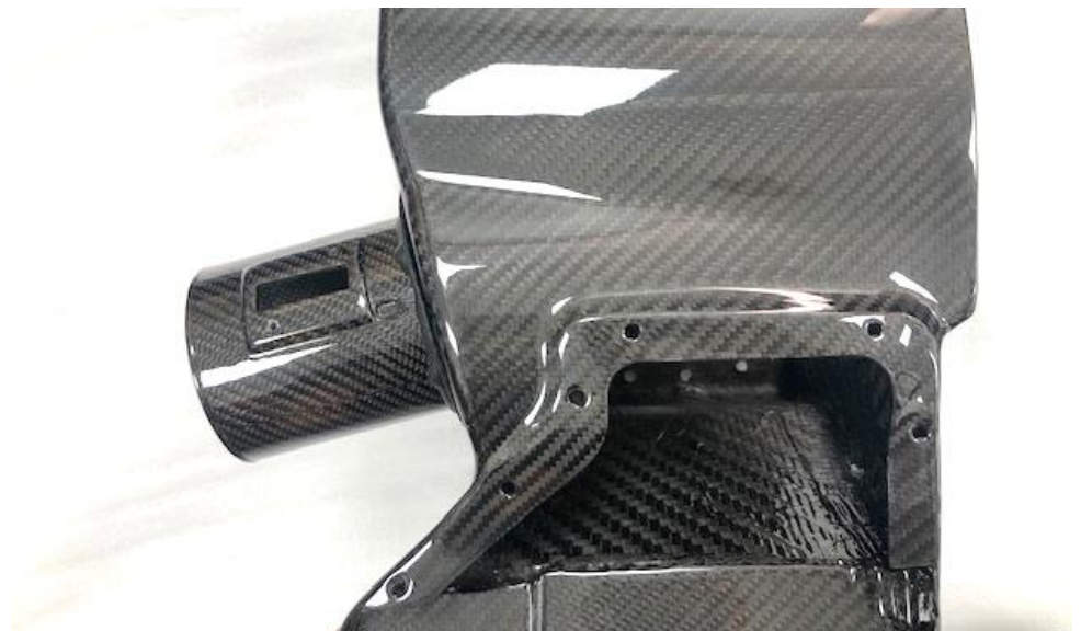
8. Push the new V2 MAF tube through the opening.
