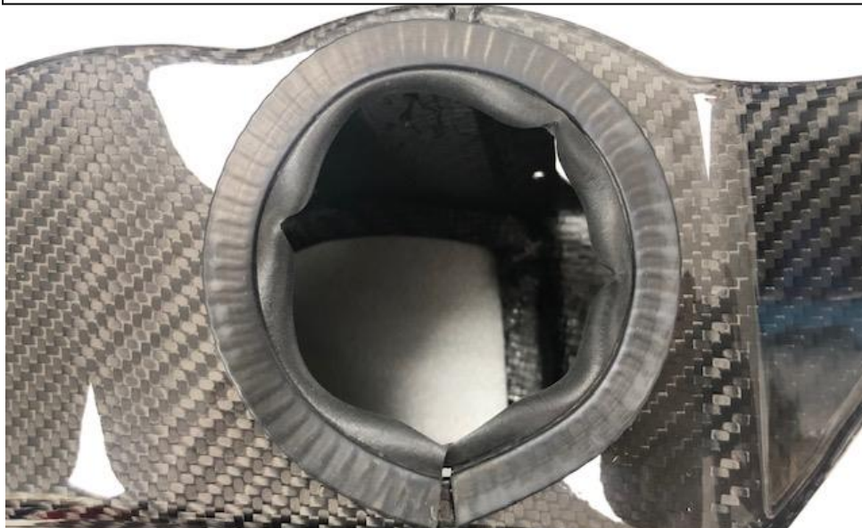
7. Refit the seal to the airbox – the UNCUT section should be facing to the outside of the airbox as shown. Make sure the seal pushed into the airbox all the way around.
