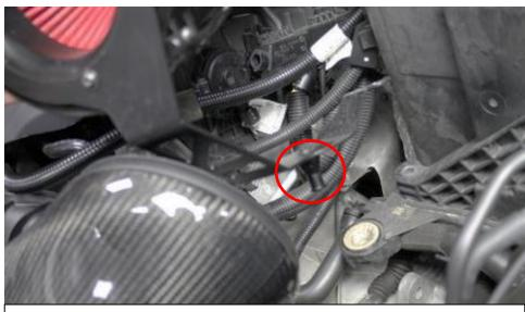
18. At the base of the bracket on the housing there is a mounting locator (circled) – push this into the rubber grommet indicated by the arrow.
