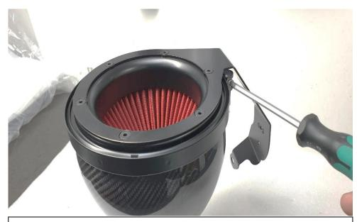
2. Unscrew and remove the V-band which is holding the filter to housing with a 4mm Hex screwdriver
