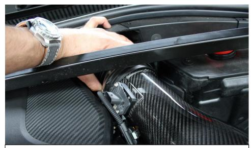
17. Push the filter housing into the turbo inlet pipe. Make sure it is all the way in. The pipe should almost touch the MAF sensor holder.
