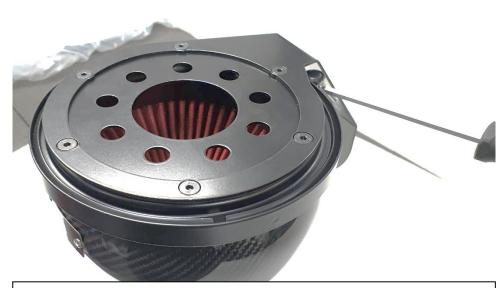
17. Place the V-band around the housing the latch of the v-band must be under the bend of the housing bracket. Secure with 4mm Hex screwdriver
