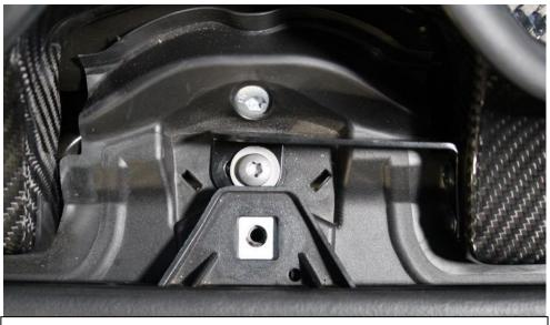
14. Secure the middle bracket with the Torx screw removed previously.
