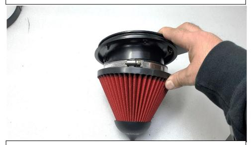
12. Place the housing bracket assembly into the filter making sure that it is properly inserted
