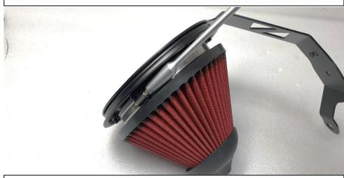
3. Once the filter assembly has been removed unscrew the screw clamp from the filter with a 7mm socket and remove the housing bracket assembly from the filter.
