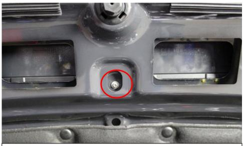
22. Now we will remove the bonnet scoop. Start by removing the torx screw shown.
