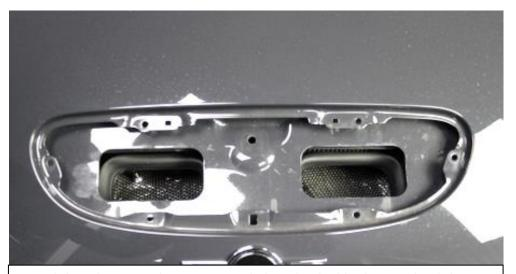
28. Stick the sealing strip to the scoop area marked in red. It should go between the 2 holes on each side. See next photo. Do not cover the holes.
