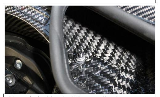
16. Secure the duct through the openings with the nuts removed in step 2.
