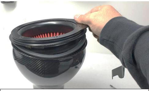
2. Remove the Filter assembly and the gasket from the housing.
