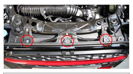
10. First remove the 3 Torx screws which secure the top of the front bumper.
