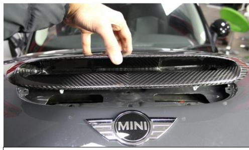
30. Carefully lower the carbon scoop into position – make sure the 6 clips are already installed on the back of the scoop.
