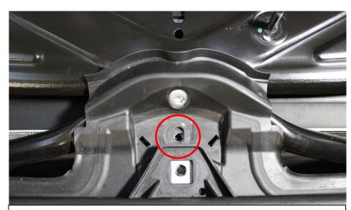
11. Now remove the middle Torx screw which is partially under the plastic tab of the bumper.
