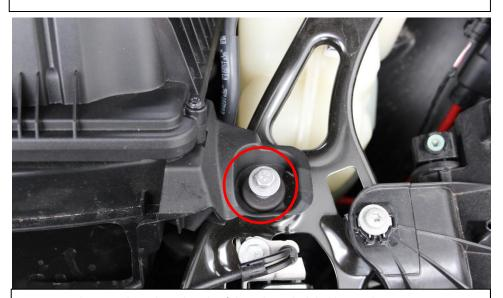
4. Remove the M6 Bolt on the right side of the airbox which holds it in place.
