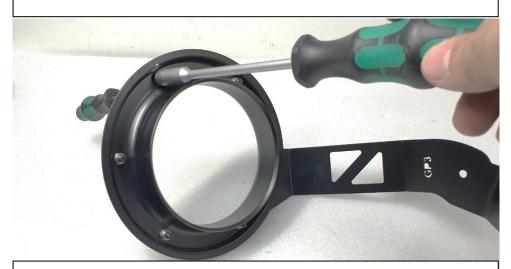
4. Once the housing bracket assembly has been removed unscrew the housing bracket from the cowl with an 8mm socket and 3mm Hex screwdriver.
