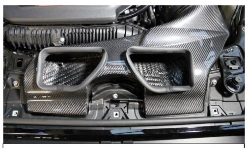
12. Push the duct into place and ensure the studs in step 8 go through the rubber grommets in step 9.
