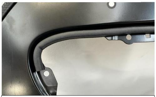
29. Close up of one side of the location for the strip. Make sure to avoid covering the holes.
