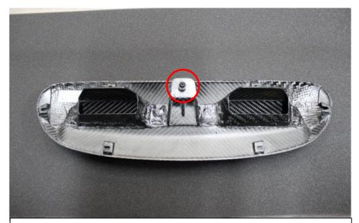
26. Check the back of the carbon scoop – if you have an M5 screw pre-installed as shown then remove it. If not - simply continue to the next step.
