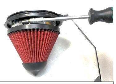
13. Secure the filter to the housing bracket assembly with a 7mm socket
