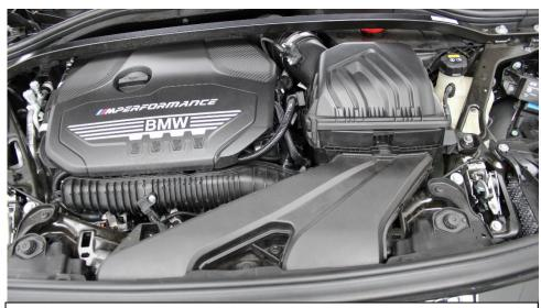
1. We will start by removing the stock airbox and duct. BMW 135i engine shown which is the same.
