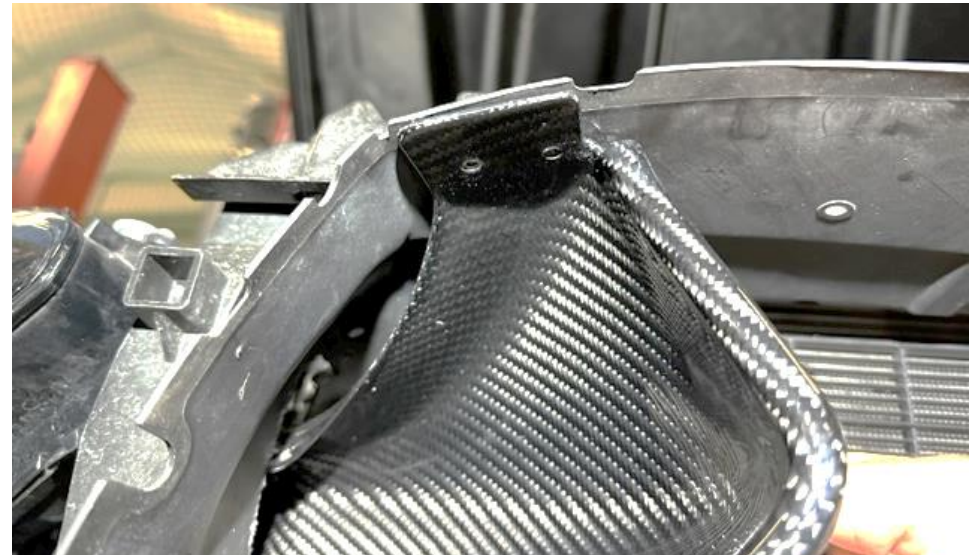
12. Line up the top of the scoop with the edge of the surround as shown. Mark the 2 hole positions through the scoop and drill them – remove the scoop to make the holes.
