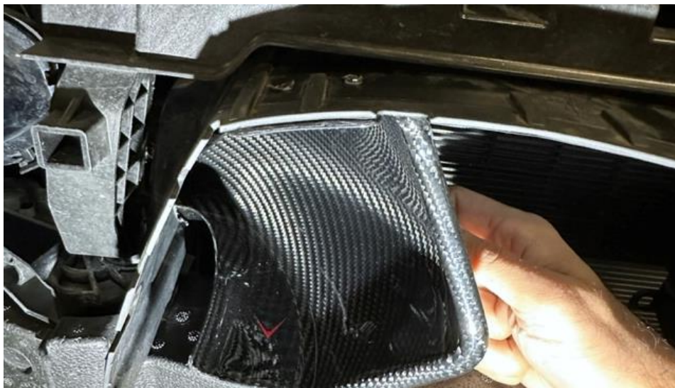
11. Take the LHS Scoop and push it through the opening. The red V should be at the bottom. The base of the scoop should be resting flat against the crash pad.
