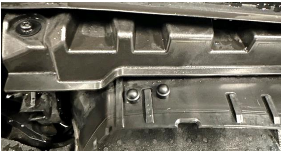
15. Now use the supplied caps to cover the nuts. The scoop is now fully installed.
