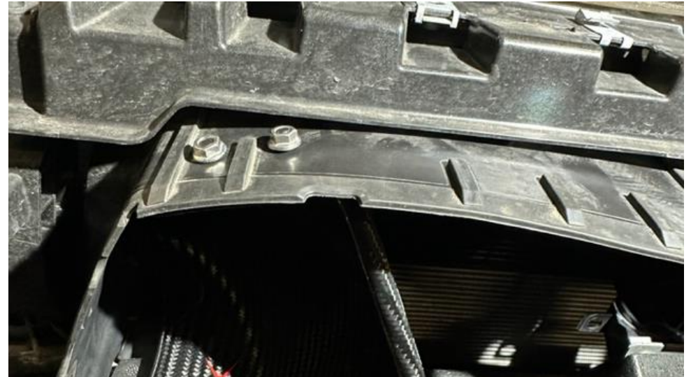
14. Use 2 of the supplied M5 nuts to secure the screws.
