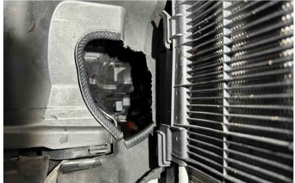
10. Install the longer trim to the edge closer to the front of the car and the small trim at the bottom as shown.
