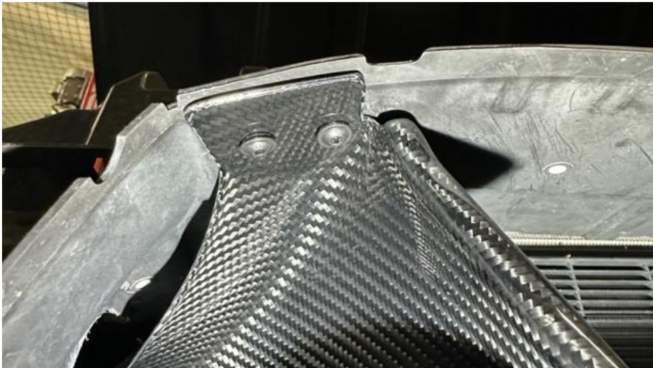
13. Push the 2 supplied M5 screws and plastic washers through the holes in the scoop.
