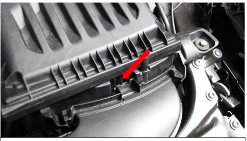
2. Release the front of the duct by pushing in the clip on the airbox.
