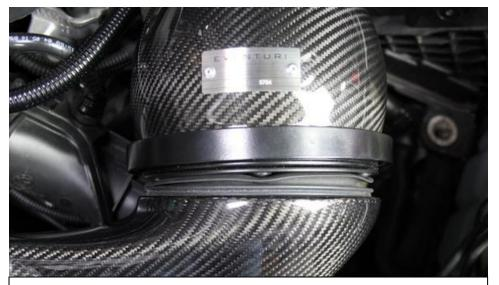
17. Align the duct and housing so that the rubber seal is covering the filter housing all the way around.
