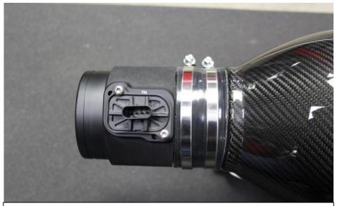
9. Assemble the MAF tube to the filter housing using the silicon coupler and 2 hose clamps. The tube must be inserted into the silicon as shown here. It is VERY IMPORTANT to get the sensor direction correct. You can see the arrow on the sensor indicating flow direction.
