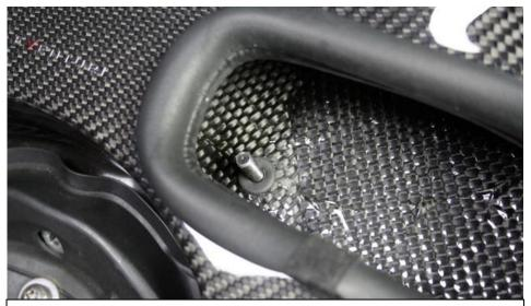
13. The threaded studs should go through the holes as shown – there is another one on the other side of the duct. Do not secure them yet.
