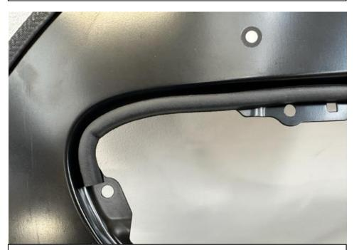
31. Close up of one side of the location for the strip. Make sure to avoid covering the holes.
