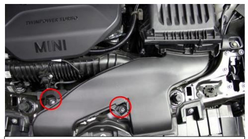
1. We will start by removing the intake duct. Remove the 2 x 10mm nuts as circled.
