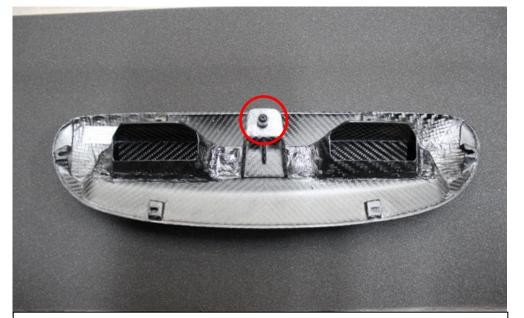
28. Check the back of the carbon scoop – if you have an M5 screw pre-installed as shown then remove it. If not - simply continue to the next step.
