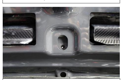
34. Once clipped into place – secure the scoop by screwing the torx screw removed in step 24. IF your scoop came pre-assembled with a new screw in this position from step 28 – use the new screw to secure the scoop.
