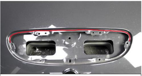
30. Stick the sealing strip to the scoop area marked in red. It should go between the 2 holes on each side. See next photo. Do not cover the holes.
