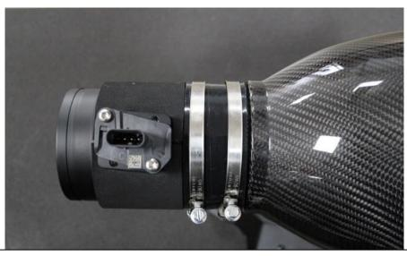
10. Similarly here is the LCI version. Assemble the MAF tube to the filter housing using the silicon coupler and 2 hose clamps. The tube must be inserted into the silicon as shown here. It is VERY IMPORTANT to get the sensor direction correct. You can see the arrow on the sensor indicating flow direction.
