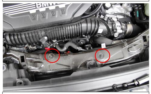
8. The new duct will be installed with these M6 Studs locating into the holes at the base of the carbon duct – see next photo.
