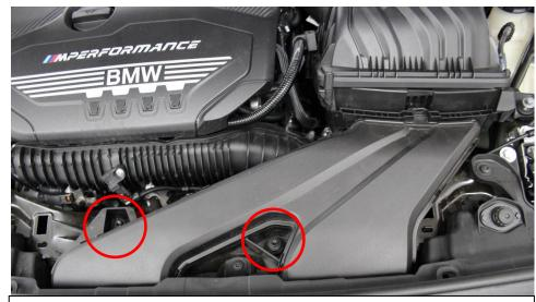
2. Remove the 2 M6 nuts holding the duct in place. Remove the duct by unclipping it from the airbox.
