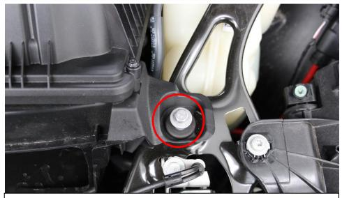
4. Remove the M6 Bolt on the right side of the airbox which holds it in place.
