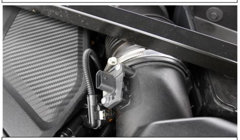
3. Disconnect the MAF sensor Plug. Loosen the hose clamp around the tube.
