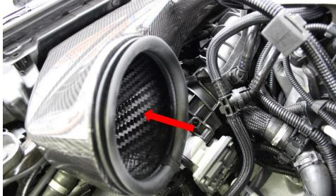
13. Secure the remaining side by reaching into the opening.
