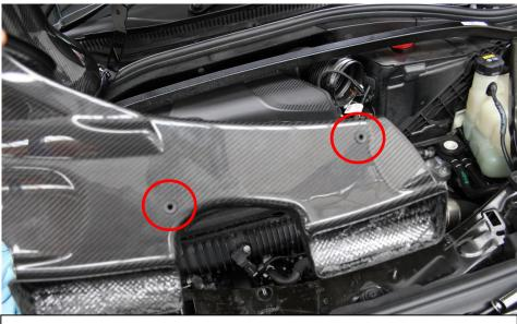
9. Here are the 2 holes which the studs go into.
