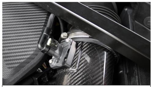
18. Reconnect the MAF plug and secure the hose clamp around the inlet tube. Do not over tighten.
