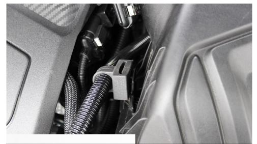
5. Remove the rubber loom holder from the left side of the airbox.
