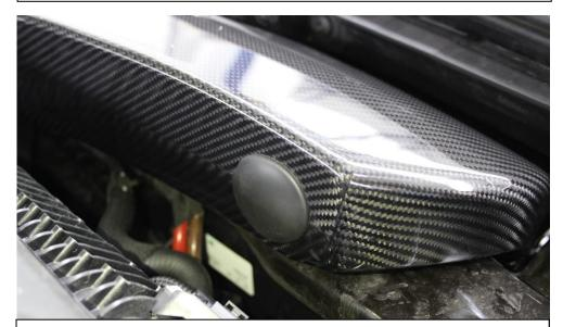
12. Close the Access Hole with the supplied rubber plug.
