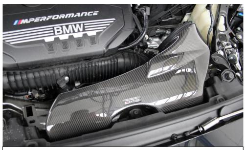
10. Install the duct into place.
