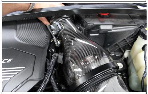
16. Line up the filter housing with the duct and then secure the bracket with the Bolt removed previously. See next step.
