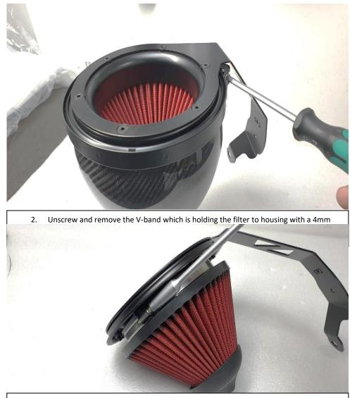
3. Once the filter assembly has been removed unscrew the screw clamp from the filter with a 7mm socket and remove the housing bracket assembly from the filter.
