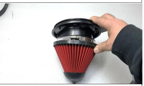
12. Place the housing bracket assembly into the filter making sure that it is properly inserted
