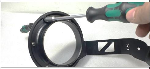
4. Once the housing bracket assembly has been removed unscrew the housing bracket from the cowl with an 8mm socket and 3mm Hex screwdriver.
