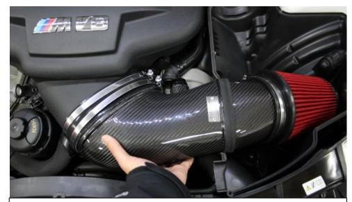
8. Lower the tube into the box and push into the silicon hose – ensure the clamp around the silicon is loose.
