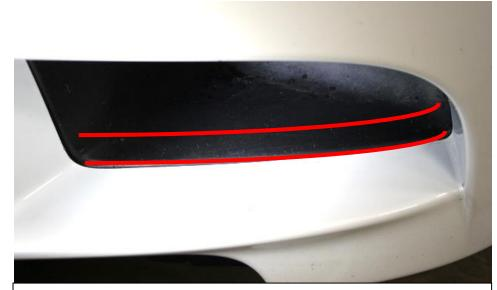
17. Use the supplied 3M wipe to clean the front portion of the intake duct under the headlamp. You only need to clean the first 25mm or so – as shown.
