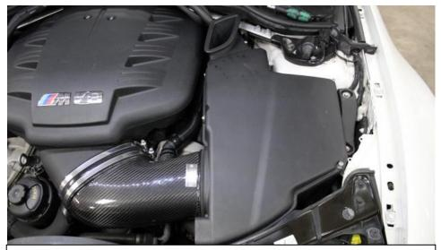
14. Put the airbox lid back on and tighten the Torx screws.
