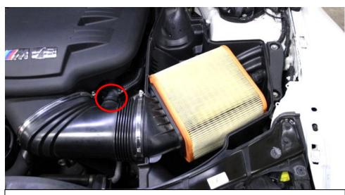
3. Remove the lid from the airbox and you will be left with the stock filter and tube. Loosen the hose clamp around the tube at the inlet manifold. Unclip the breather from the tube as circled.
