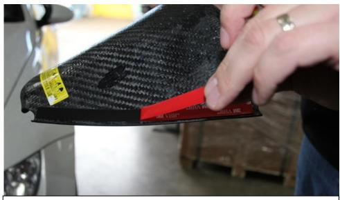
18. Remove the protective film on the 3M adhesive at the base of the carbon scoop.
