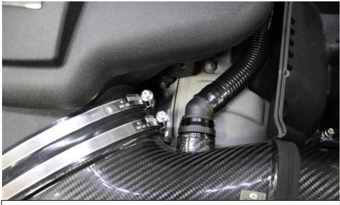
10. Tighten the remaining hose clamp and also insert the breather tube into position. It will click into place.
