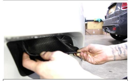
20. Insert the scoop as shown – go underneath the temperature sensor to avoid it. Push the scoop all the way back.
