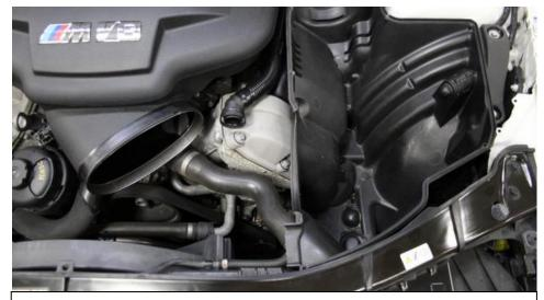
4. Remove the inlet tube and filter from the airbox.
