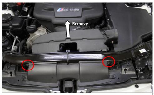
1. Start by removing the engine side of the top duct. Remove the 2 screws as circled and pull out the duct.
