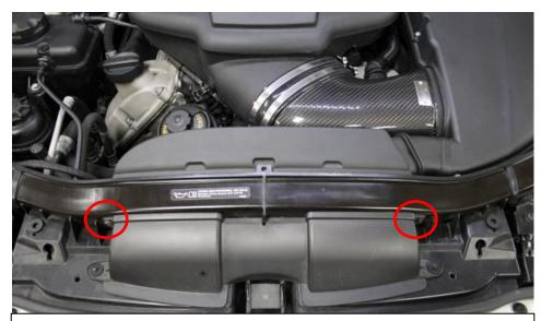
16. Insert and tighten the screws for the duct again.
