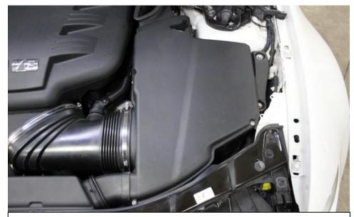
2. Loosen the Torx screws around the top of the airbox lid.
