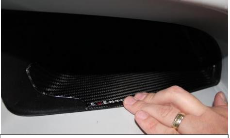
21. Locate the front edge of the scoop into the gap between the black plastic duct and the bumper. Press down on the front of the scoop for 10 seconds firmly to ensure a good bond.
