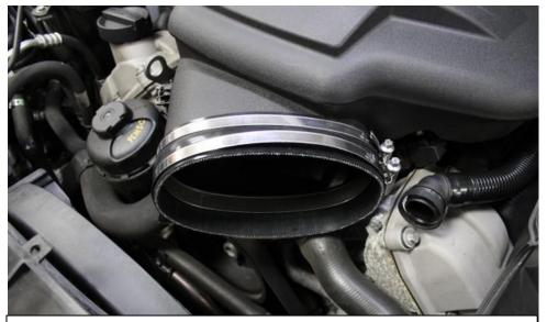
5. Push the silicon hose onto the inlet manifold – make sure it is evenly inserted all around. Place the 2 supplied hose clamps onto the silicon. The clamps are circular but will bend into shape once tightened. See next step before tightening.
