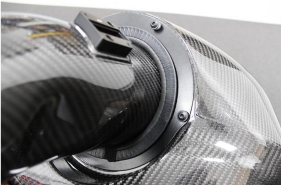
17. Another view of the sealing plate secured to the airbox.
