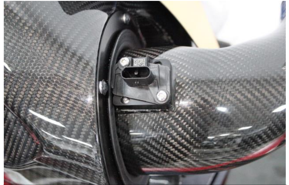
18. Install the temperature sensor onto the tube using the supplied screws. DO NOT use the stock screws.
