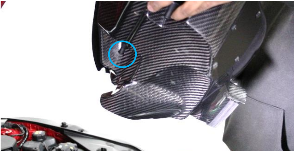
19. Carefully lower the airbox into the engine bay. The mount circled blue should sit in the rubber mount shown in next photo.
