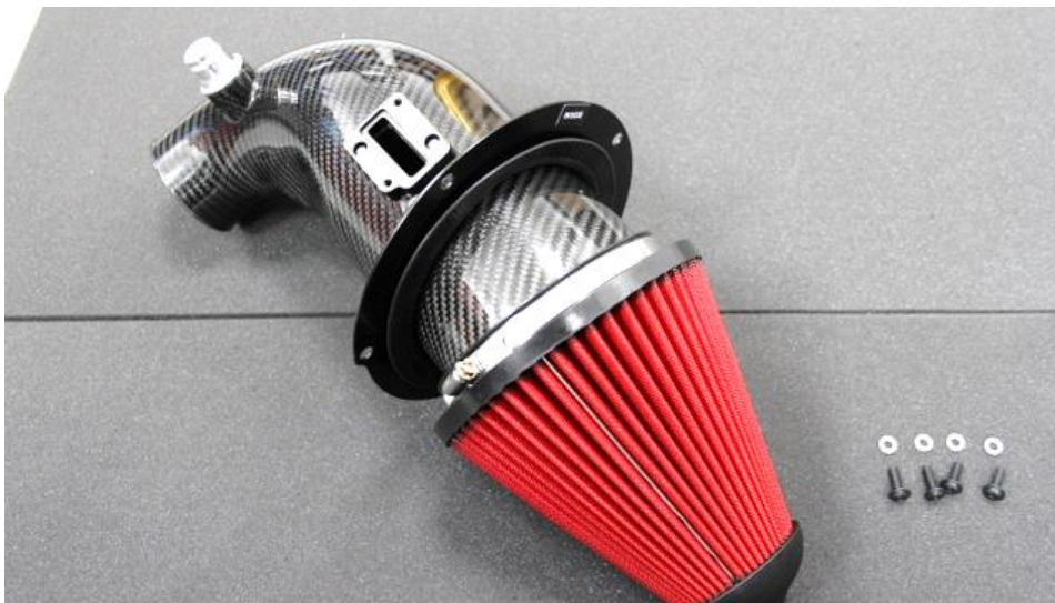
15. Push the sealing plate onto the tube – ensure the INSIDE label is facing the filter side. Now push the filter fully onto the tube and secure with the attached clamp.
