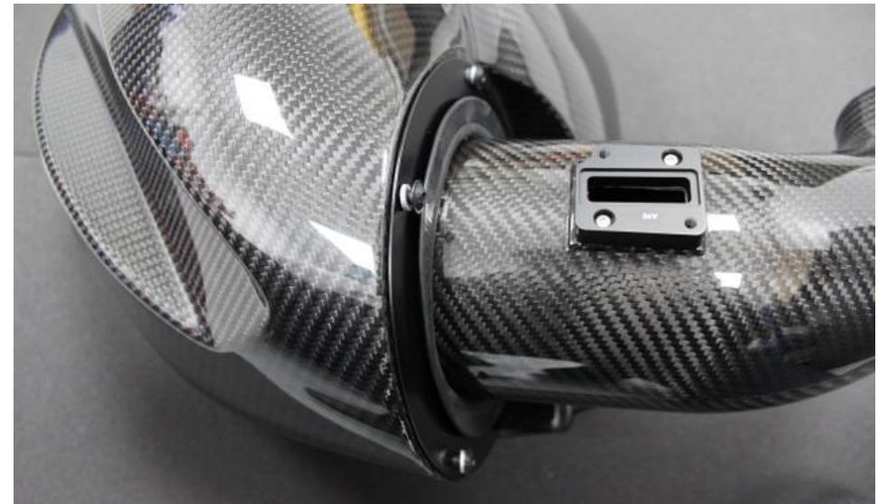
16. Insert the filter into the airbox and line up the holes on the sealing plate. Secure with the supplied M5 screws and lock washers.
