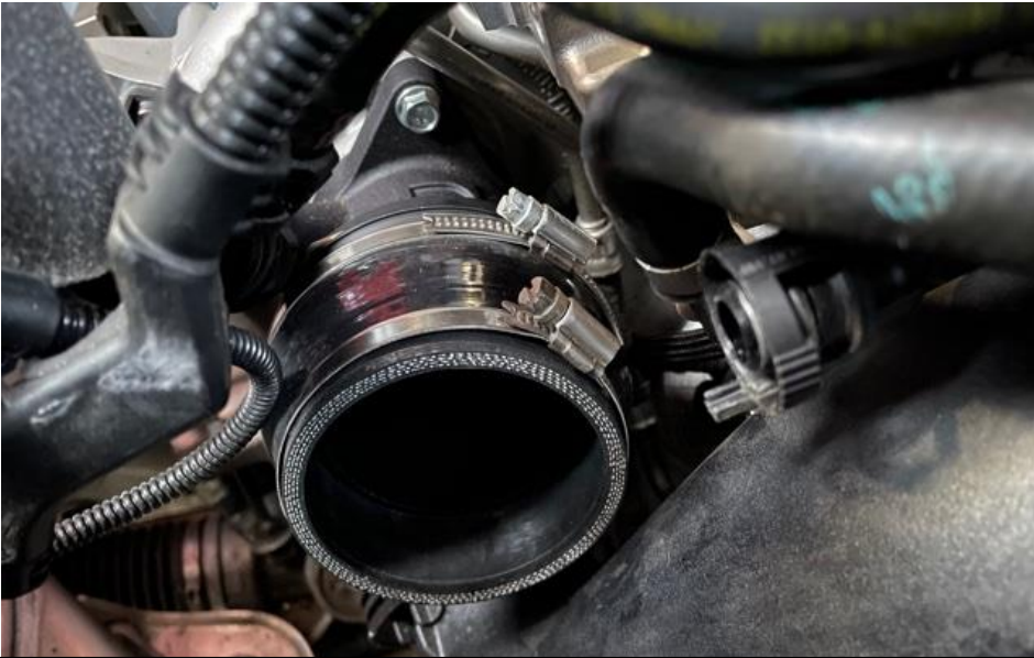
13. Install the flange assembly onto the turbo inlet – it will click into place.
