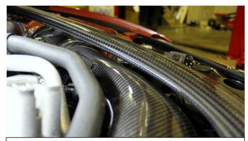
45. Place the strut brace into position to check for clearance above the carbon tube. Rotate tube if necessary. There should be a small gap between the tube and the strut brace and between the tube and fan shroud below. Remove strut brace.
