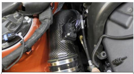
35. Now tighten the lower clamp on the tube – ensure there is no gap between the flange on the carbon tube and the silicon.
