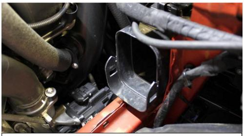
25. Looking at the other side – identify the 2 holes on the stock opening which will again be used for location and securing the left side duct.
