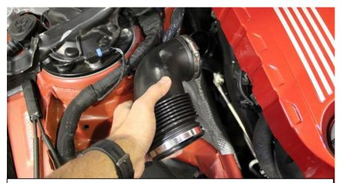
8. Loosen the remaining hose clamp on the intake tube and remove from engine bay.
