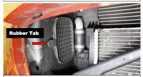
48. With the grills removed, you will see these inner grids which need to be removed. Simply pull the rubber tab to release the grid and remove completely. See next photo.
