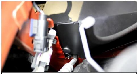
24. Now do the same with the other side. You will need to push the duct away from the chassis metal work to get access to the hole. Once secured – you will notice that the duct still has some movement – this is required for allowing adjustment on the intake housing.
