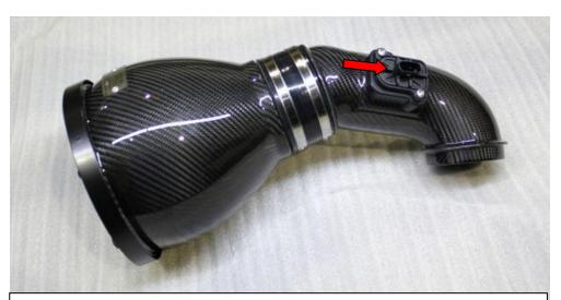
31. Assemble the LHS intake with the LHS tube (shorter tube) with the 80mm silicon coupler and 2 hose clamps. Orient the tube as shown here and in the next photo. When pushing the silicon coupler onto the intake – **DO NOT PUSH ON THE FILTER ITSELF.** Ensure airflow arrow on sensor is as shown.
