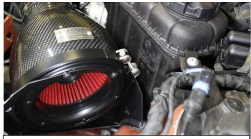
40. Place the mouth of the intake into the duct – rotate the Band Clamp to avoid the duct.
