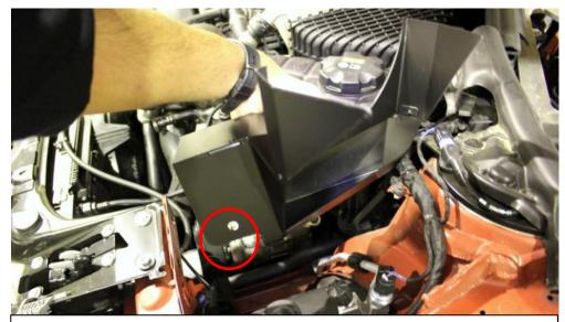
21. Take the right side duct (larger one) and locate the holes at the back over the holes shown previously on the stock duct opening. The new duct should go OVER the stock one.
