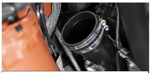
29. Taking the shorter 76mm coupler, push over the intake tube on the LEFT side of the engine. Make sure the coupler is pushed down fully and put two hose clamps around the coupler as shown. Tighten the LOWER clamp only.
