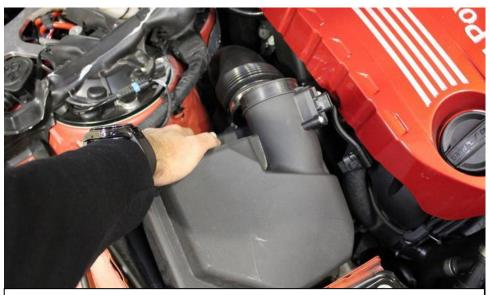
6. Push the intake tube off the airbox and then pull the back of the airbox upwards to remove. It is held in place by 2 rubber grommets. Remove the airbox from the engine bay.
