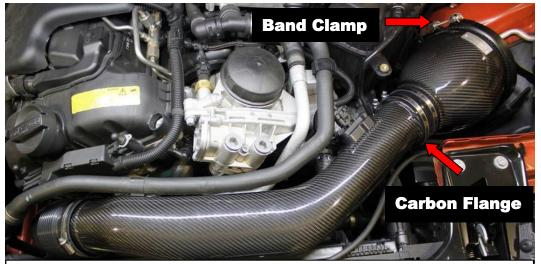
46. Once positioned correctly, tighten the hose clamps on both sides of the carbon tube. Ensure there is no gap between the flange on the carbon and the silicon as shown. Tighten the Band Clamp holding the filter and housing together. Reinstall strut brace with all 13mm bolts and the 10mm bolt.
