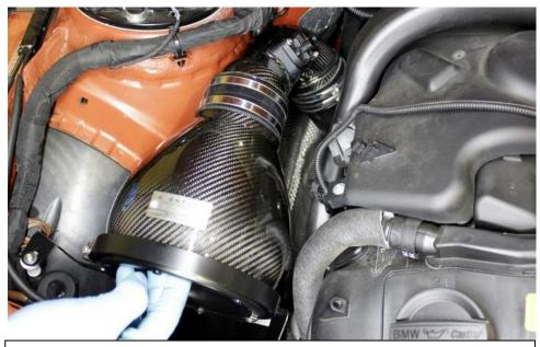
33. Lower the intake assembly into the left side and push the tube into the silicon coupler installed previously. Locate the opening of the intake into the duct installed previously. Rotate band clamp if needed for clearance with duct – see step 35.
