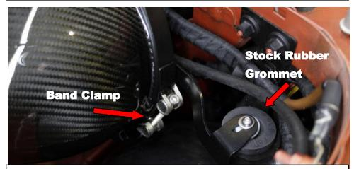
35. Push the plastic boss on the mounting bracket into the stock rubber grommet fully. You might need to rotate the Band Clamp to avoid the duct. This has been left loose to allow rotation.
