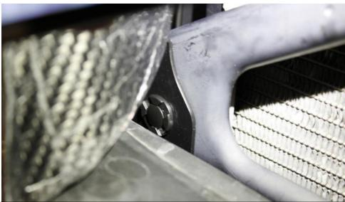
56. Push rivet fully secured in place.
