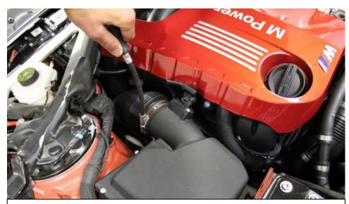
4. Loosen hose clamp on the left side (looking at the engine) airbox.
