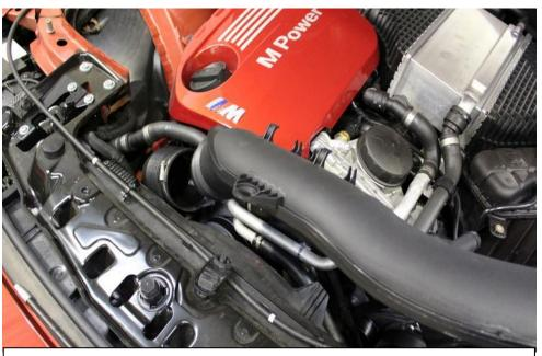
14. Loosen hose clamp and pull the tube out from the intake pipe.
