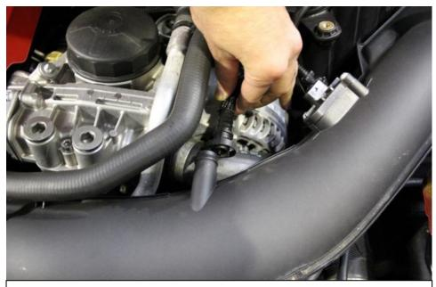
13. Remove Breather hose from tube. Pinch the sides of the plastic ring inwards and pull out.
