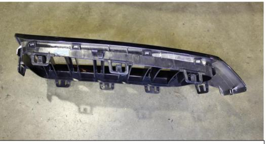
Here is the removed grill with tabs shown. If you cannot release the tabs as shown, you will need to remove the Torx screws holding the top of the bumper in. They are under the rubber strip. You can then pull the top of the bumper out and gain access from the top.
