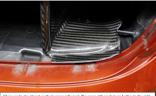
57. Lower lip should rest on the bumper grill panel. The scoop still needs to go further to the right to be in correct position. See next steps.
