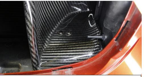
59. Pull the bumper area around the bottom of the scoop out to allow the lower lip of the scoop to go underneath as shown. The scoop should now locate as shown.
