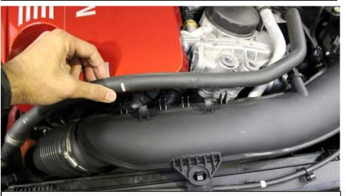
11. Pull the rubber hosing out of the long intake tube.
