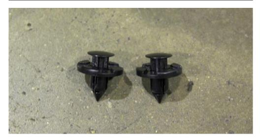
55. Using one of the smaller push rivets supplied, insert into the aligned bracket and lock into place by fully pushing in the head as shown next.
