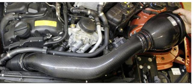
38. Lower the assembly into the engine bay – locate the carbon tube into the stock intake tube and push in.
