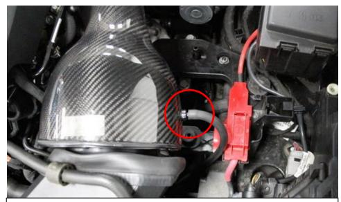
20. Route the extension tube around the bottom of the intake and push into the connector on the side.
