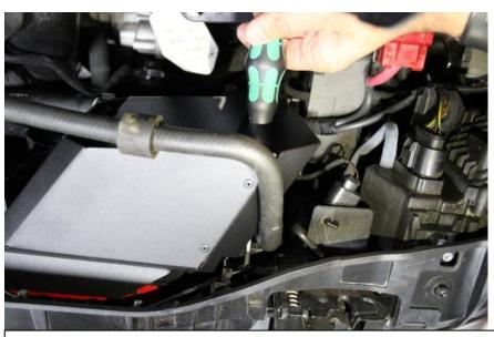
14. Secure the duct by using the same torx screws removed from the stock duct bracket in step 6. There is a hole in the right side of the new duct to allow a tool to pass through and secure the screw.
