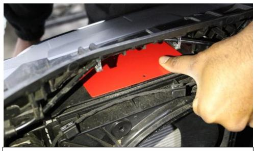
10. Put the scoop into position as shown and secure with the 2 panel clips as shown in next step.
