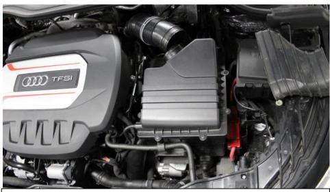
2. Loosen the clamp around the intake tube at the back of the airbox and remove the tube from the airbox. (Use appropriate spring clamp tool). Also remove the rubber duct attached to the front of the airbox. It will simply pull out.
