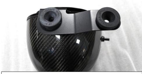
5. Install the rubber mounts into the new bracket as shown.
