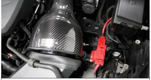
21. Ensure the rubber edging is on the outside of the intake all the way around – it does not need to seal with the intake since the scoop forces air to the filter. A small gap also derestricts the intake path.
