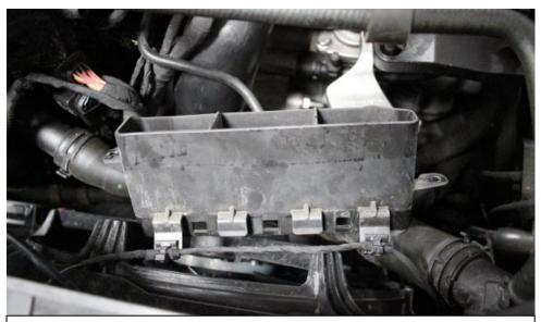
7. Remove the wire attached to the base of the duct by prising the 2 clips off the duct.
