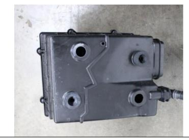
4. Remove 2 rubber mounts from the base of the airbox. We will use them in the new bracket.
