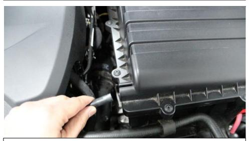
3. Remove the vacuum tube from the airbox – it will pull out.
