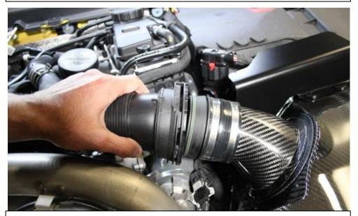
12. Remove the tube from the airbox side.
