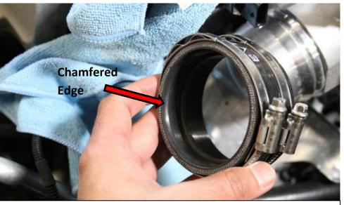
18. Take the small silicon coupler – the chamfered edge should face AWAY from the turbo.
