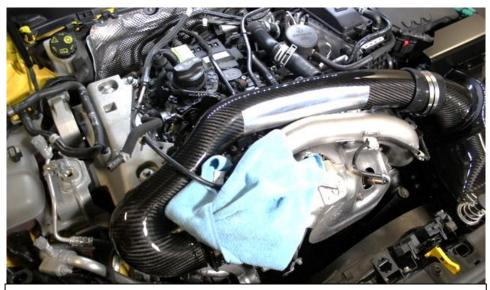
22. Carefully slide the tube into position – make sure the cloth is still covering the exposed metal coolant tubes.
