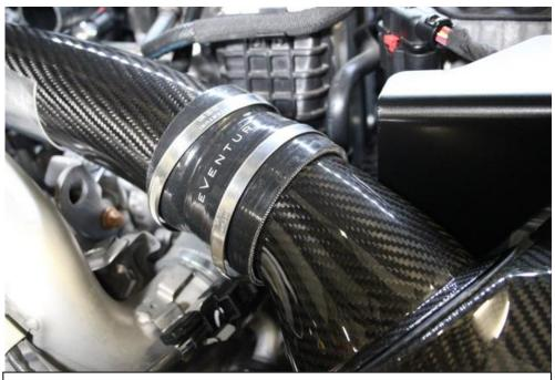
34. Secure the hose clamps at the airbox side too. Make sure the intake tube is sitting flush against the airbox.
