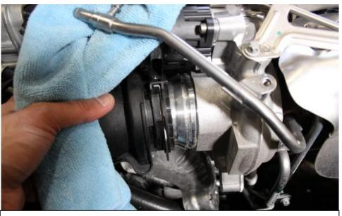
14. Remove the tube from the turbo.
