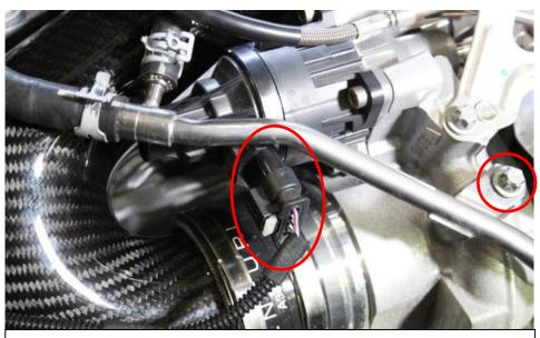
31. Install the securing screw removed previously. Also reconnect the sensor plug.
