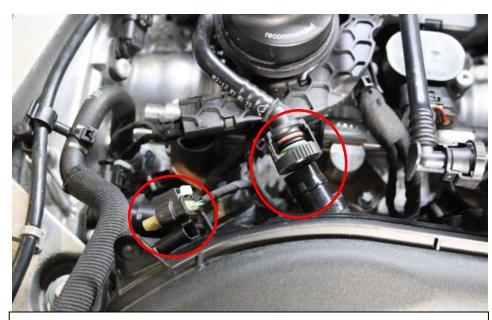
4. Remove the remaining single breather pipe and unplug the MAP sensor plug.
