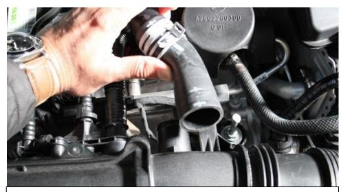
1. The turbo tube can not be used with the stock airbox – please ensure you have our intake fitted already. Start by removing the breather pipe from the back of the tube.
