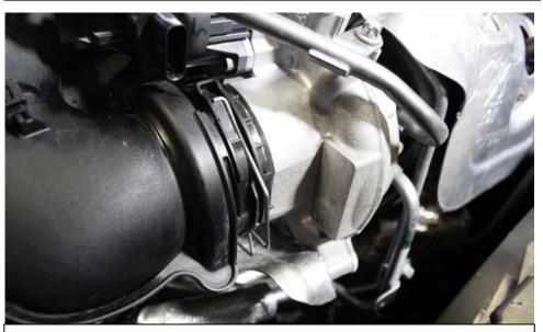
11. Pull the wire clip out which secures the tube to the turbo.
