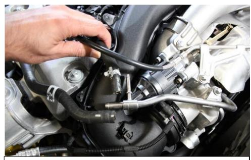
8. Remove the coolant lines as shown.
