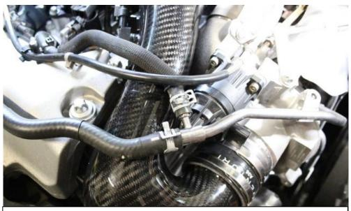
30. Re-connect the coolant hoses and the clamps.
