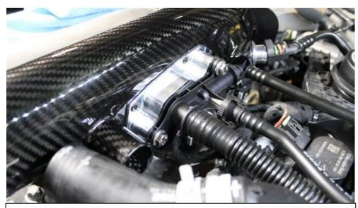
26. Push the breather block into the machined block and secure with the supplied M6 bolts.
