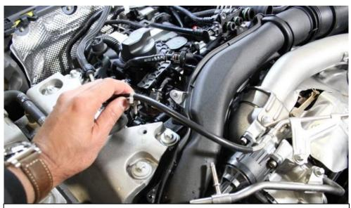
10. Pull this cable clip out for more space to remove the tube.
