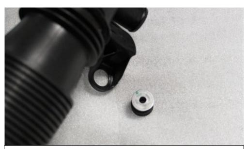
28. Remove the second rubber mount from the original tube.
