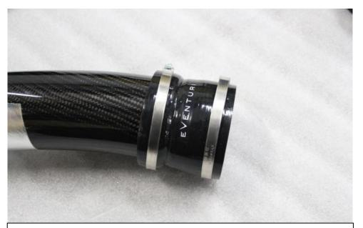
20. Insert the larger silicon hose onto the airbox side of the tube as shown.
